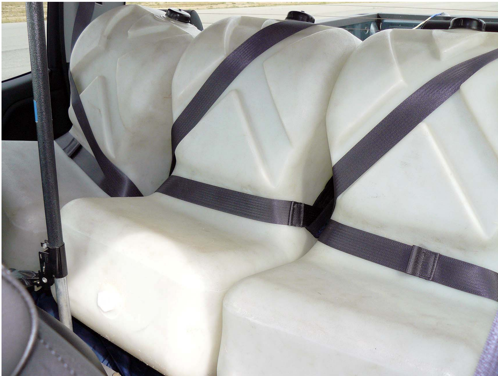
Figure A7. Ballast Condition
