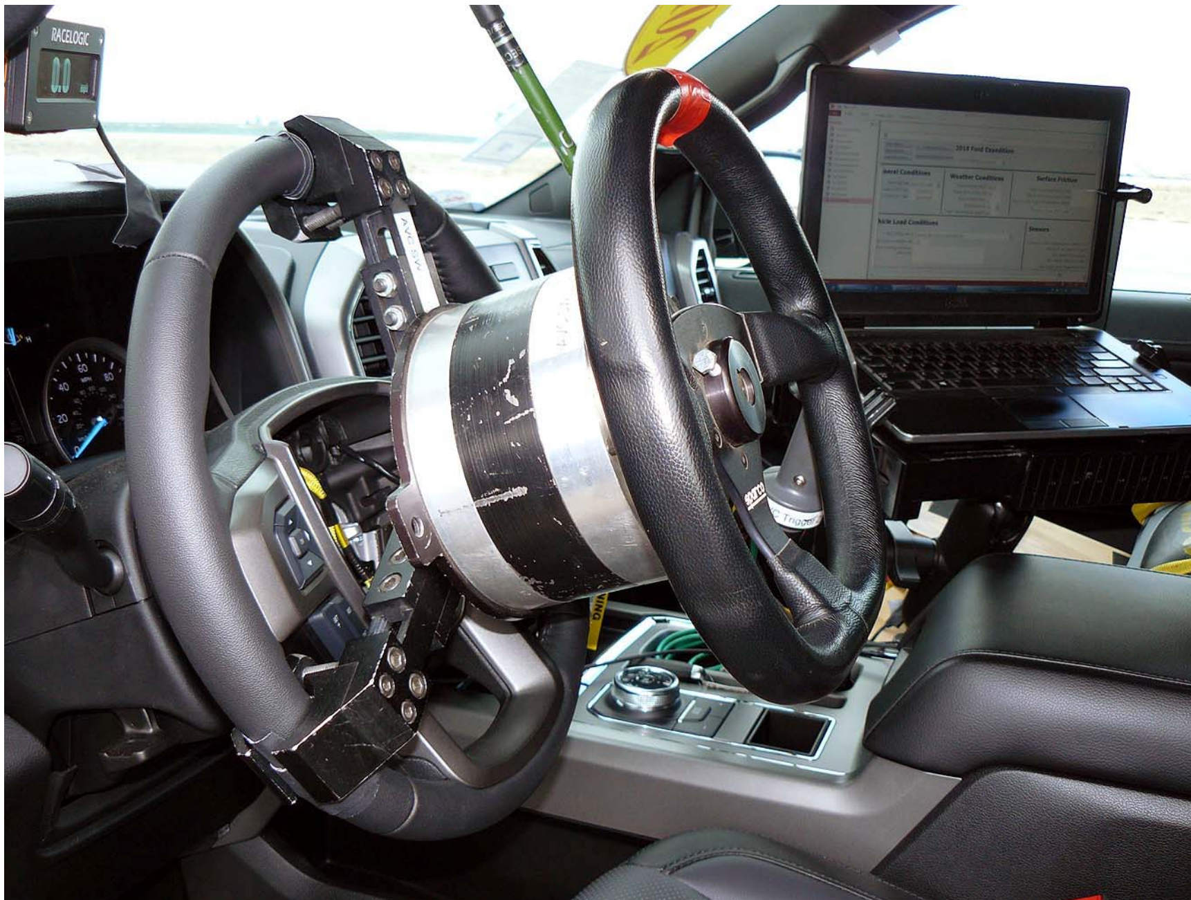
Figure A7. Steering Controller and Computer
