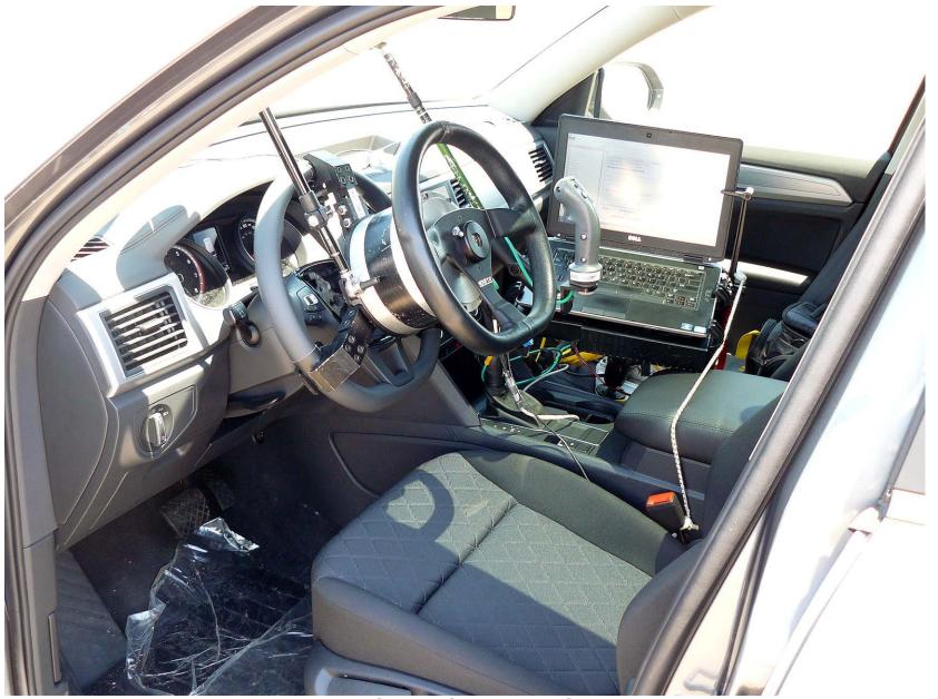
Figure A7. Steering Controller and Computer
