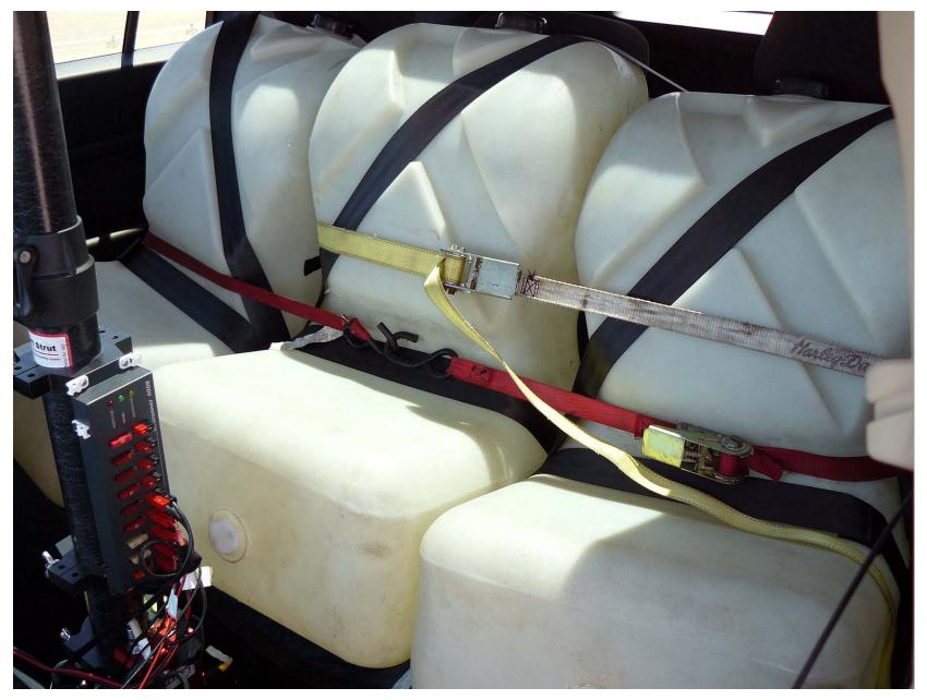
Figure A8. Ballast Condition
