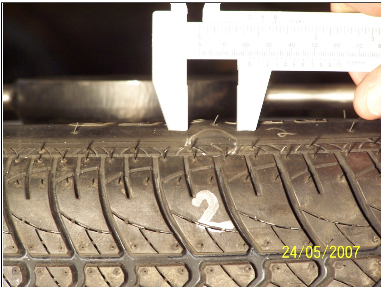
Figure 6.3 Sidewall Bulge Measurement
