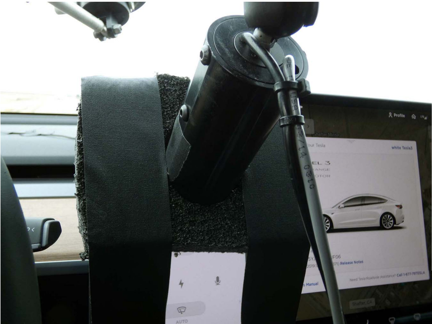
Figure A12. Sensor for Detecting Visual Alerts
