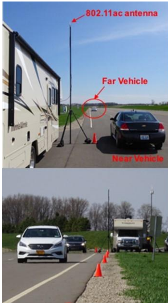
Figure 6: Test Procedure – Outdoor AP Test Configuration
