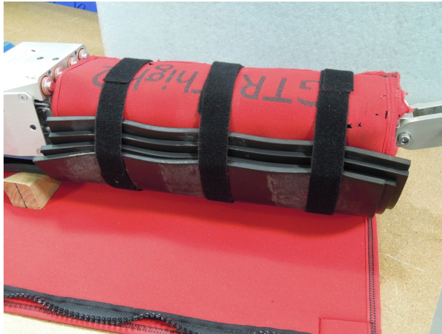
Figure 67. Securing the rubber assembly with the Velcro straps
