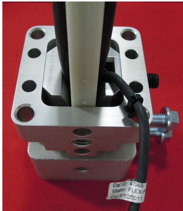
Figure 6. Insertion of bone and clamp into the base
