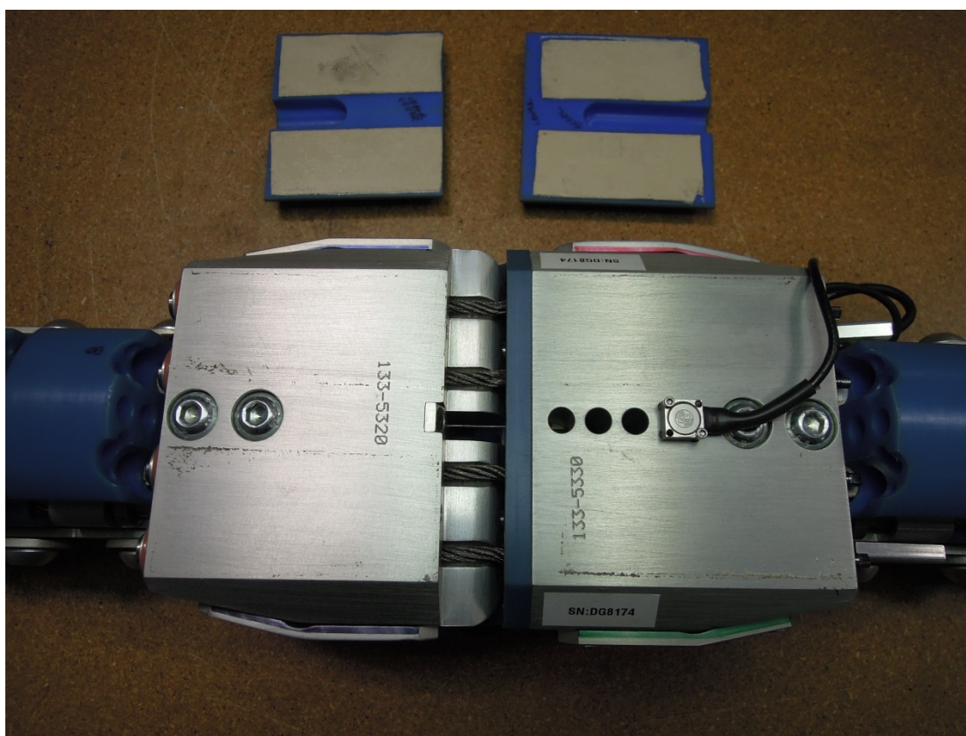
Figure 60. Knee accelerometer location on tibia knee block
