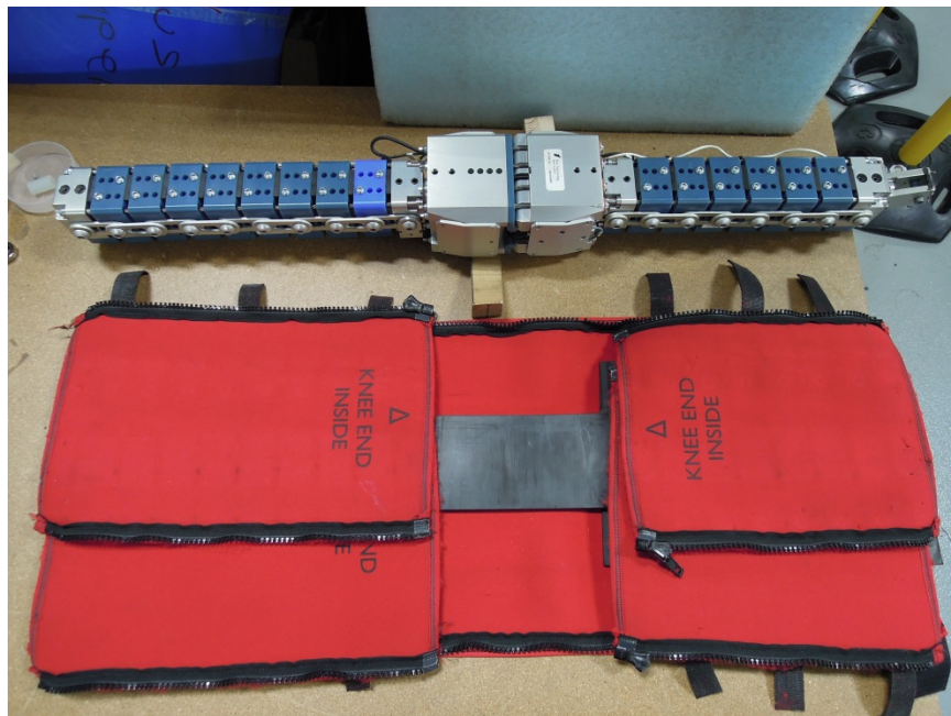
Figure 64. Positioning of thigh and leg neoprene covers
