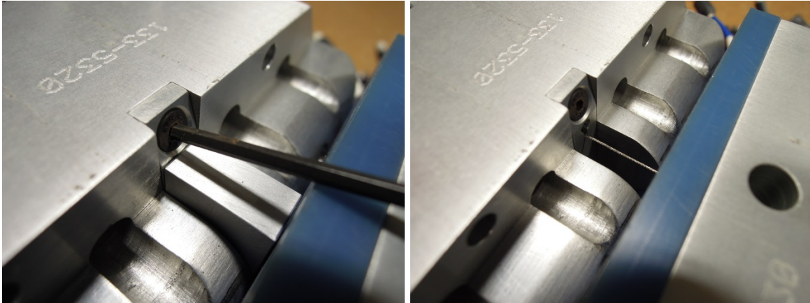
Figure 53. Fixing the string potentiometer attachment plate and removal of the spacer
