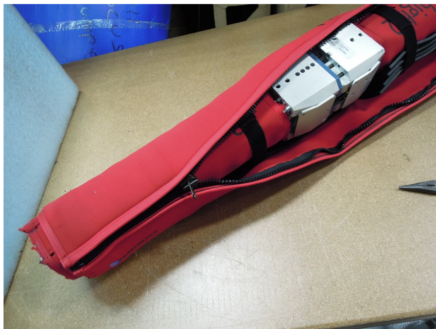
Figure 68. Zipping up the outer neoprene cover
