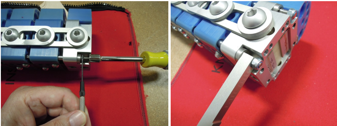
Figure 21. Setting the gap and tightening the Nylok nut
