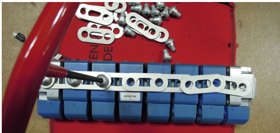
Figure 19. Installation of femur side links
