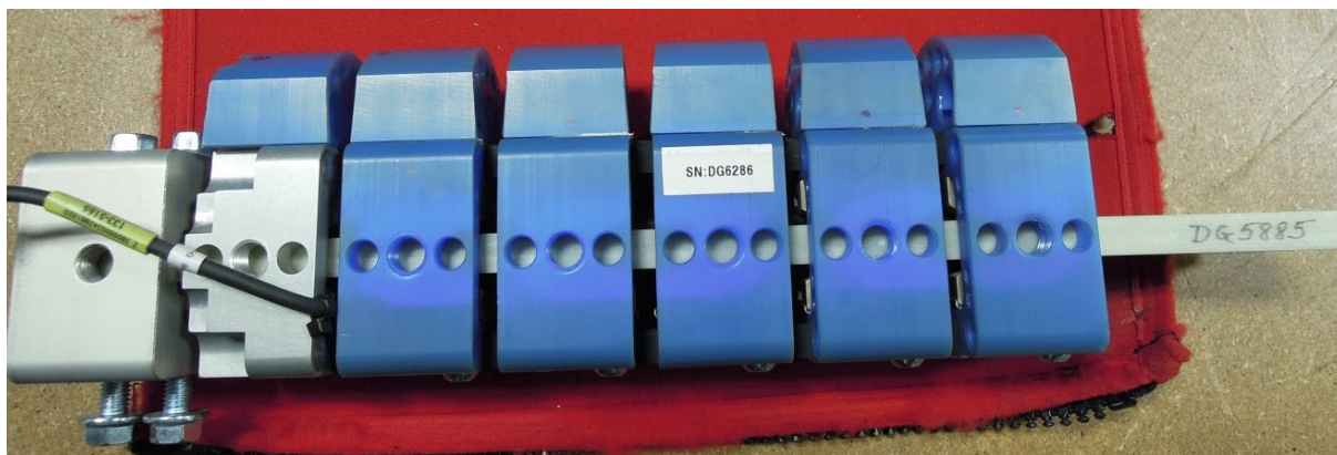
Figure 12. Femur assembly with the inner knee segment and five blue segments
