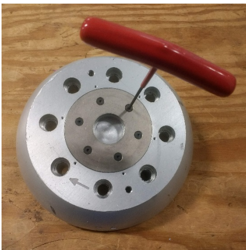
Figure 8. (Left) Attachment of back plate disc; (Right) Attachment of the back plate assembly to the skull casting assembly
