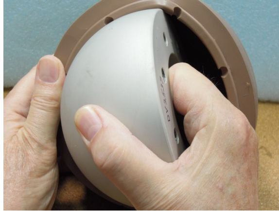
Figure 7. Insertion of skull casting assembly into the headform flesh
