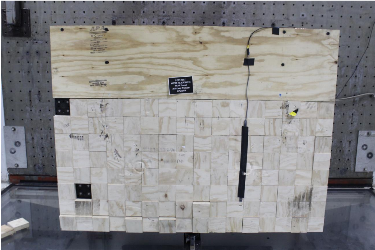
Figure A-3: Post-Test Load Cell Wall
