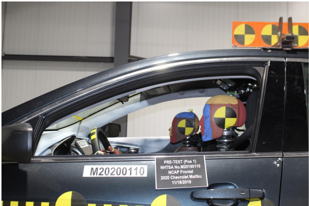
Figure A-32: Pre-Test Driver Dummy Window View
