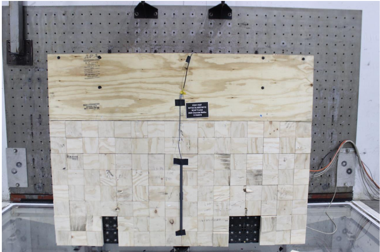
Figure A-3: Post-Test Load Cell Wall
