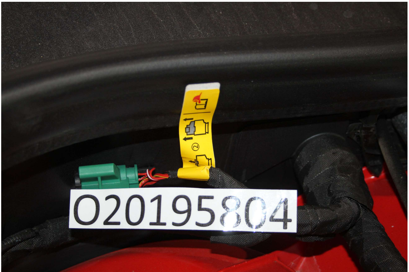
Photo No. 003 - First Responder Warning Label
