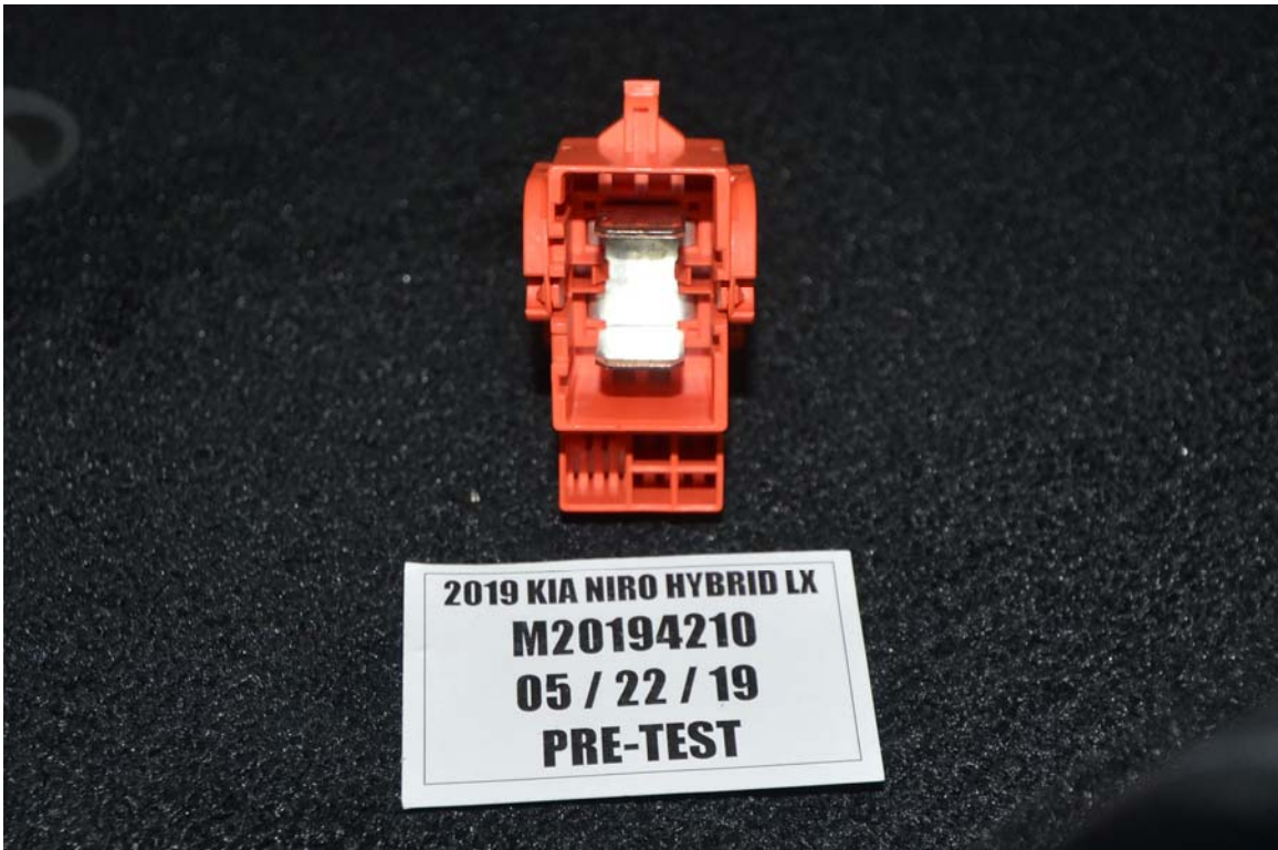
FIGURE 7. Manual High Voltage Service Disconnect Removed
