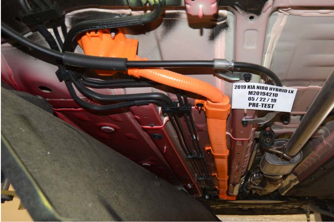
FIGURE 18. Pre-Impact View of High Voltage Interconnect(s)
