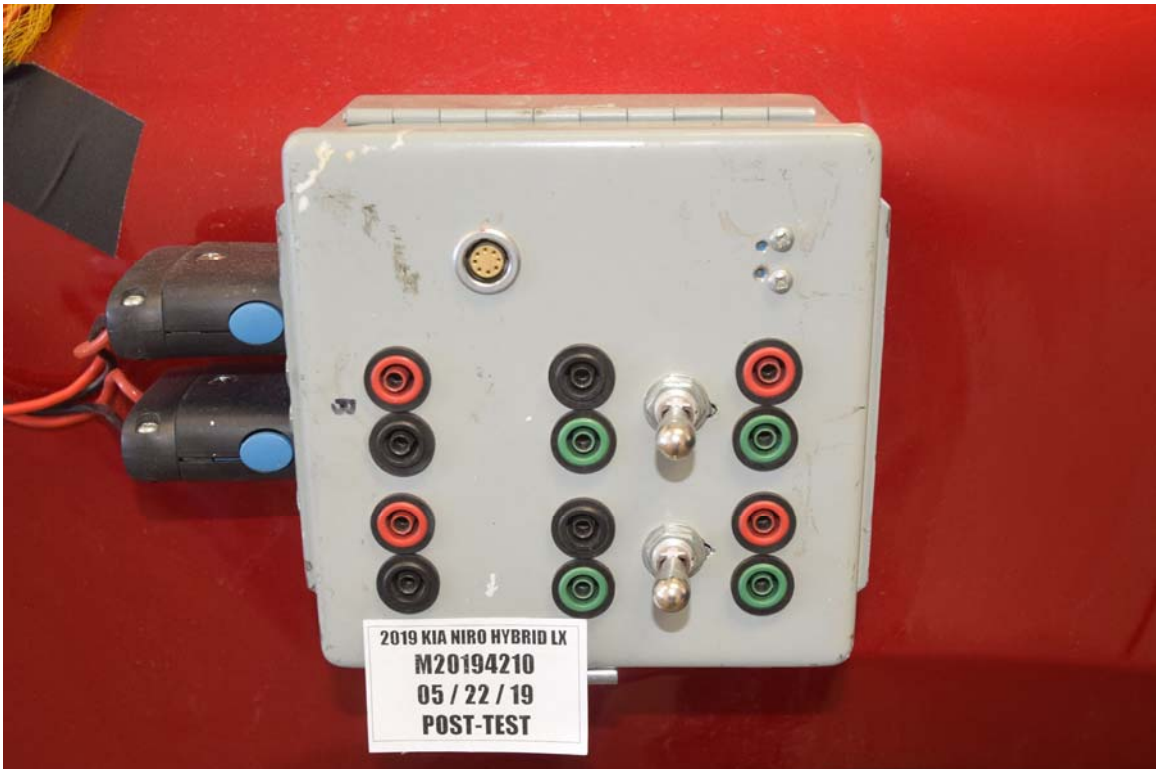
FIGURE 25. Post-Impact View of Installed Test Interface Port
