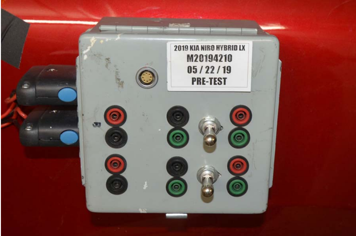
FIGURE 24. Pre-Impact View of Installed Test Interface Port
