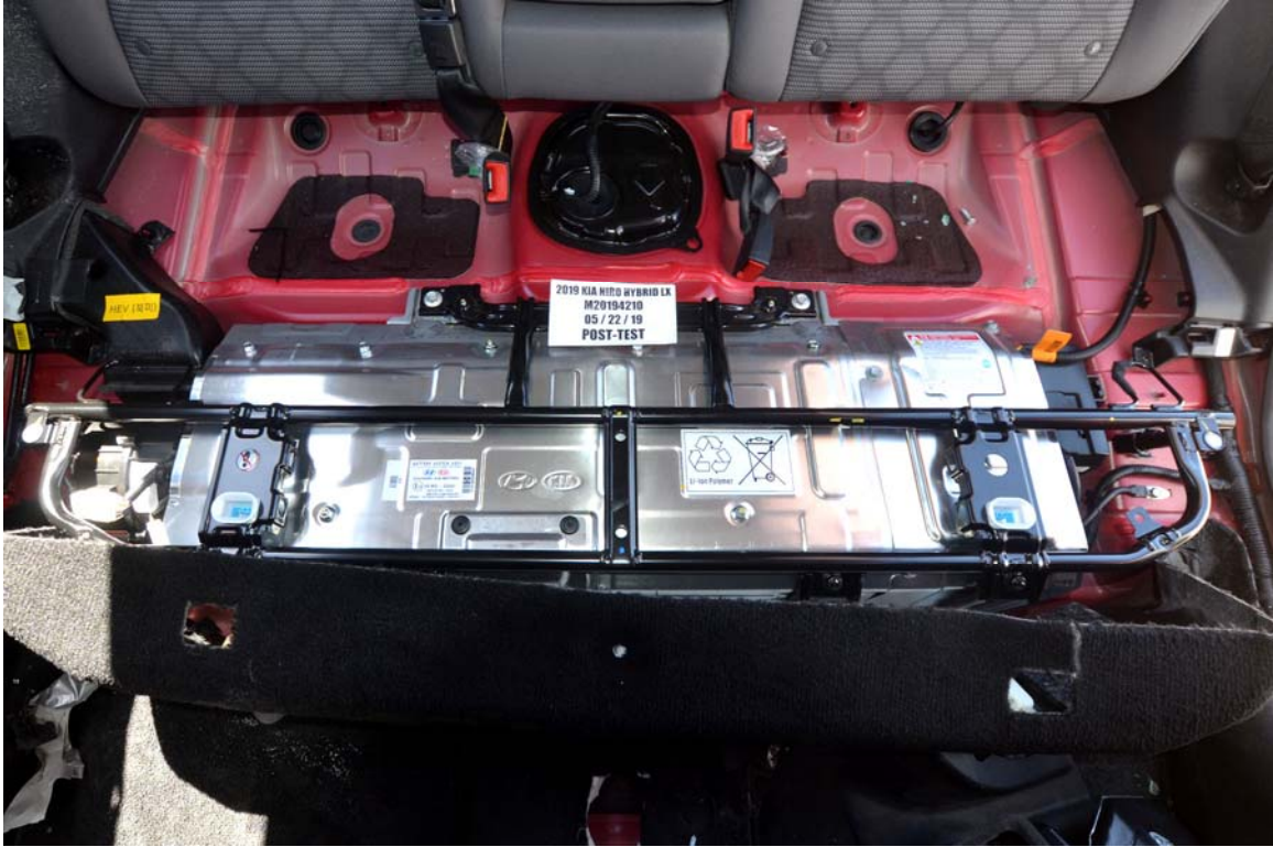
FIGURE 10. Post-Impact Front View of Propulsion Battery
