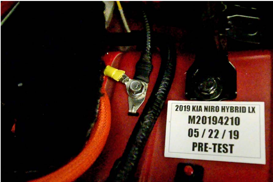
FIGURE 21. Pre-Impact View of Ground Lead Attached
