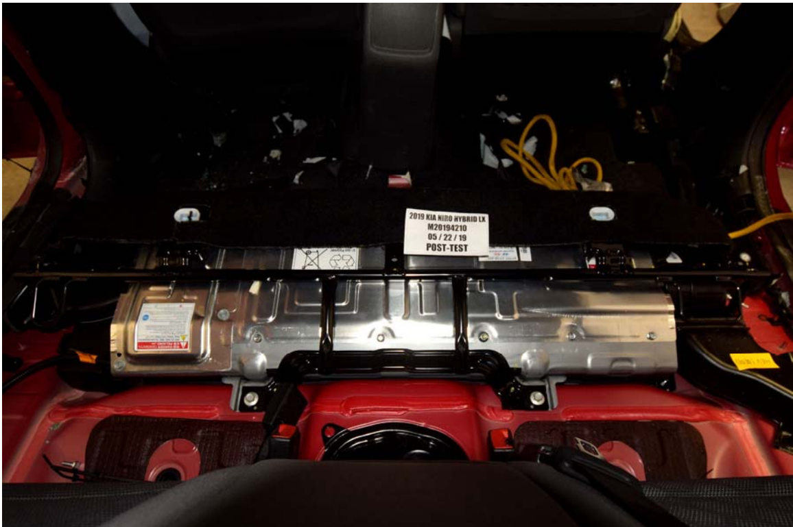
FIGURE 11. Post-Impact Rear View of Propulsion Battery
