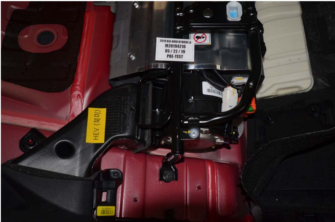
FIGURE 19. Pre-Impact View Propulsion Battery Venting System(s)
