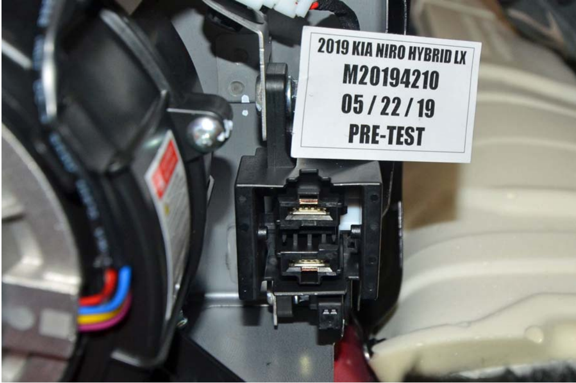
FIGURE 8. Manual High Voltage Service Disconnect Removed
