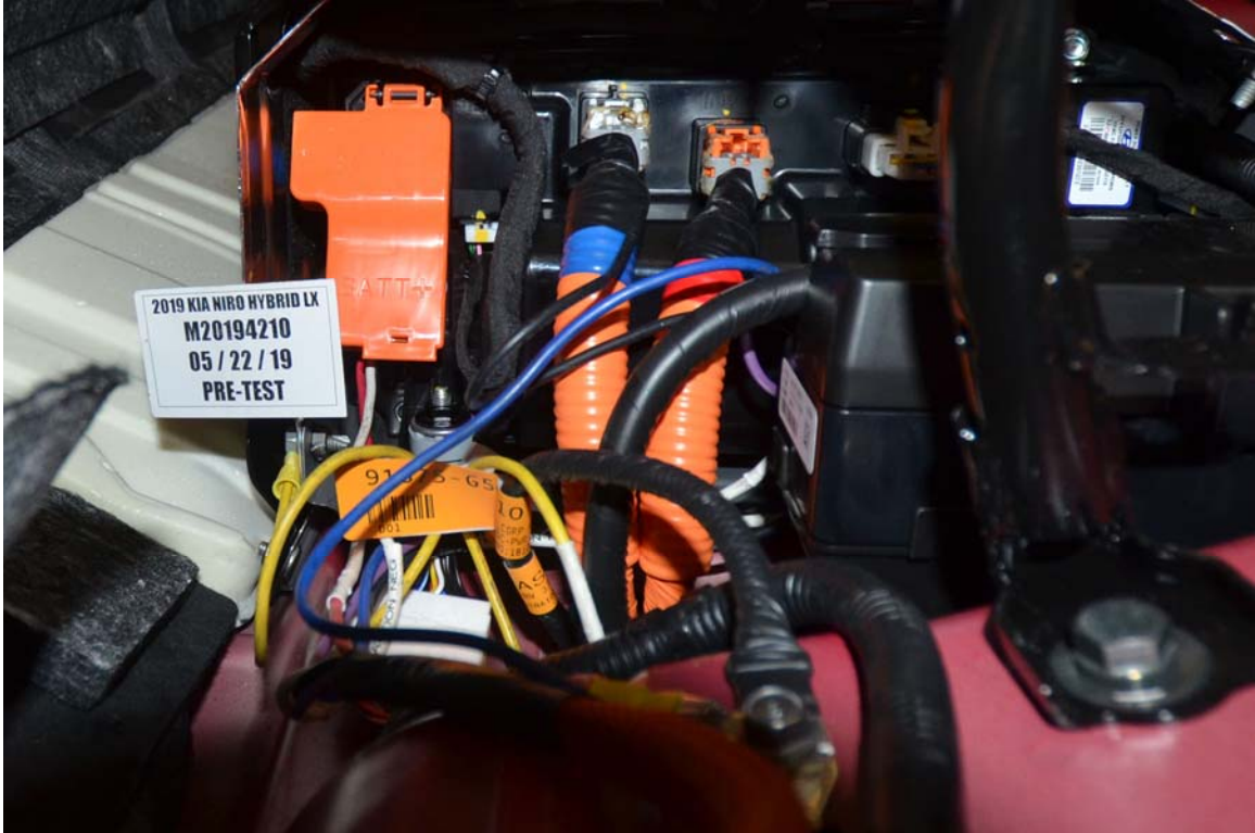
FIGURE 22. Pre-Impact View of High Voltage Leads Attached
