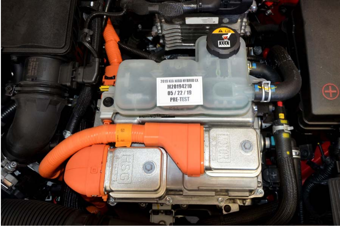
FIGURE 16. Pre-Impact View of Electric Propulsion Drive
