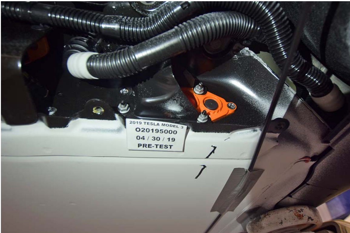
FIGURE 28. Pre-Impact View of Propulsion Battery Venting System(s)
