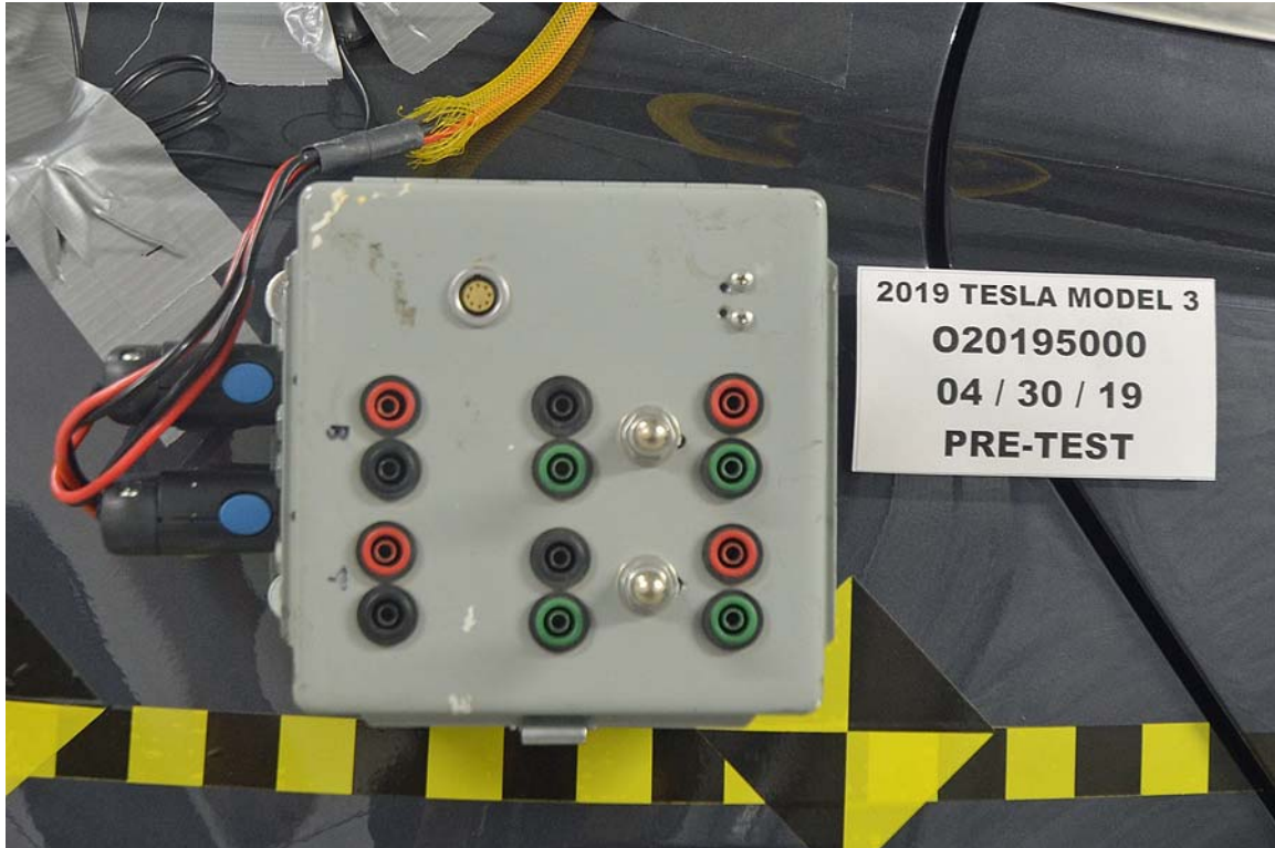
FIGURE 35. Pre-Impact View of Installed Test Interface Port
