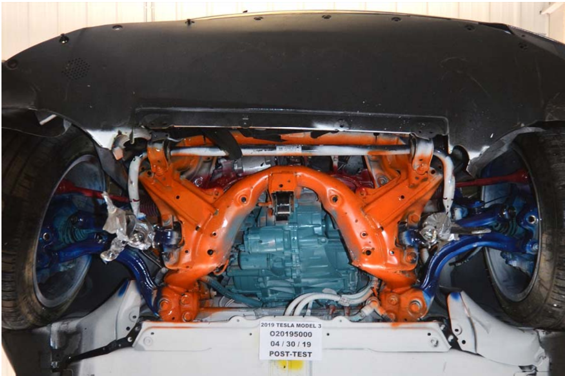
FIGURE 22. Post-Impact View of Electric Propulsion Drive
