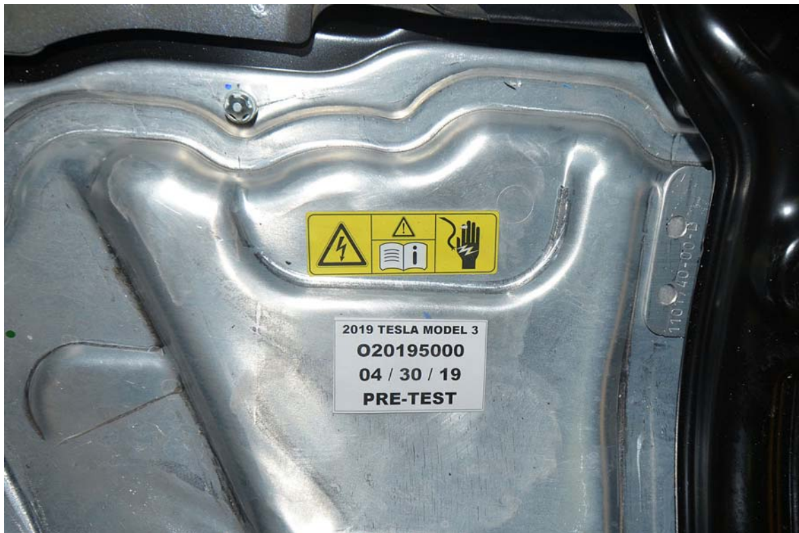
FIGURE 2. Power Inverter Warning Label
