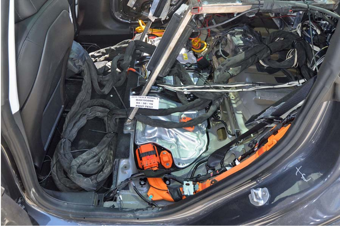
FIGURE 45. Post-Impact View of the Vehicle Passenger Compartment Adjacent to Propulsion Battery
