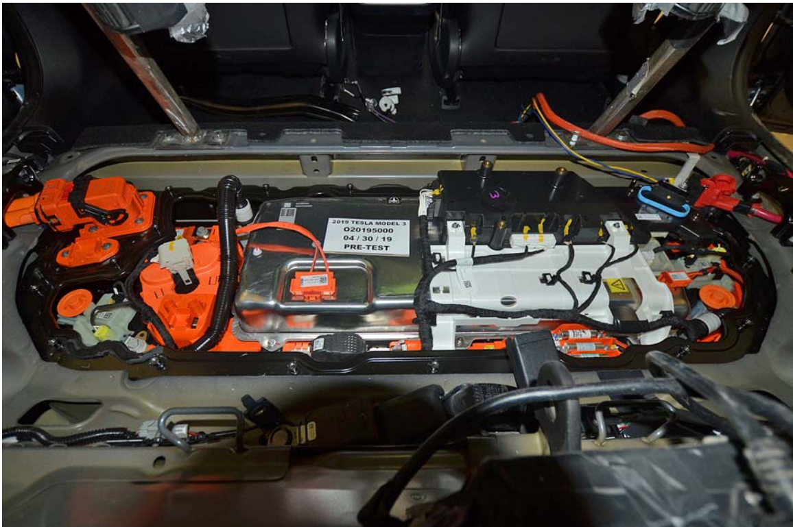
FIGURE 32. Pre-Test View of High Voltage Leads Attached
