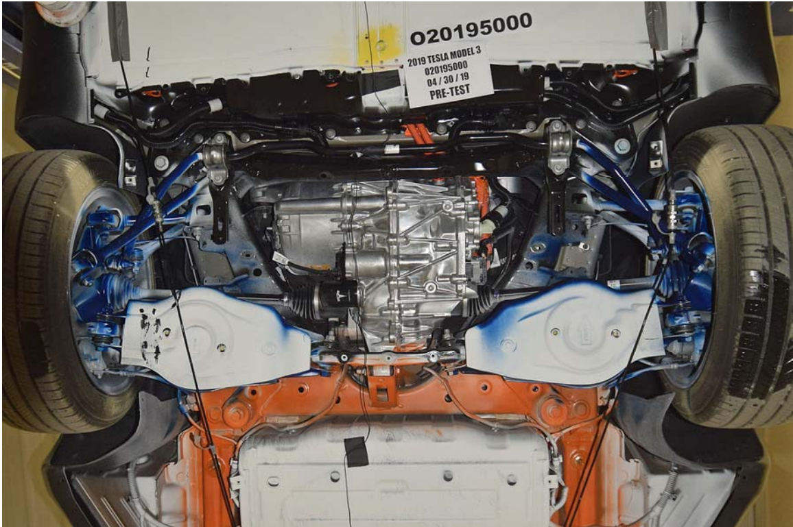
FIGURE 19. Pre-Impact View of Electric Propulsion Drive
