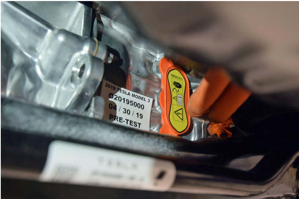
FIGURE 6. Other Vehicle Label(s) Related to Electrical Propulsion System
