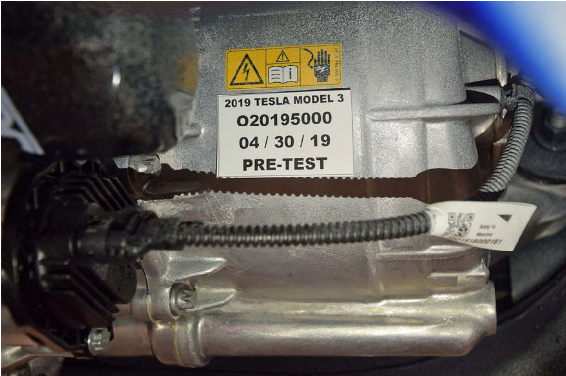
FIGURE 5. Other Vehicle Label(s) Related to Electrical Propulsion System
