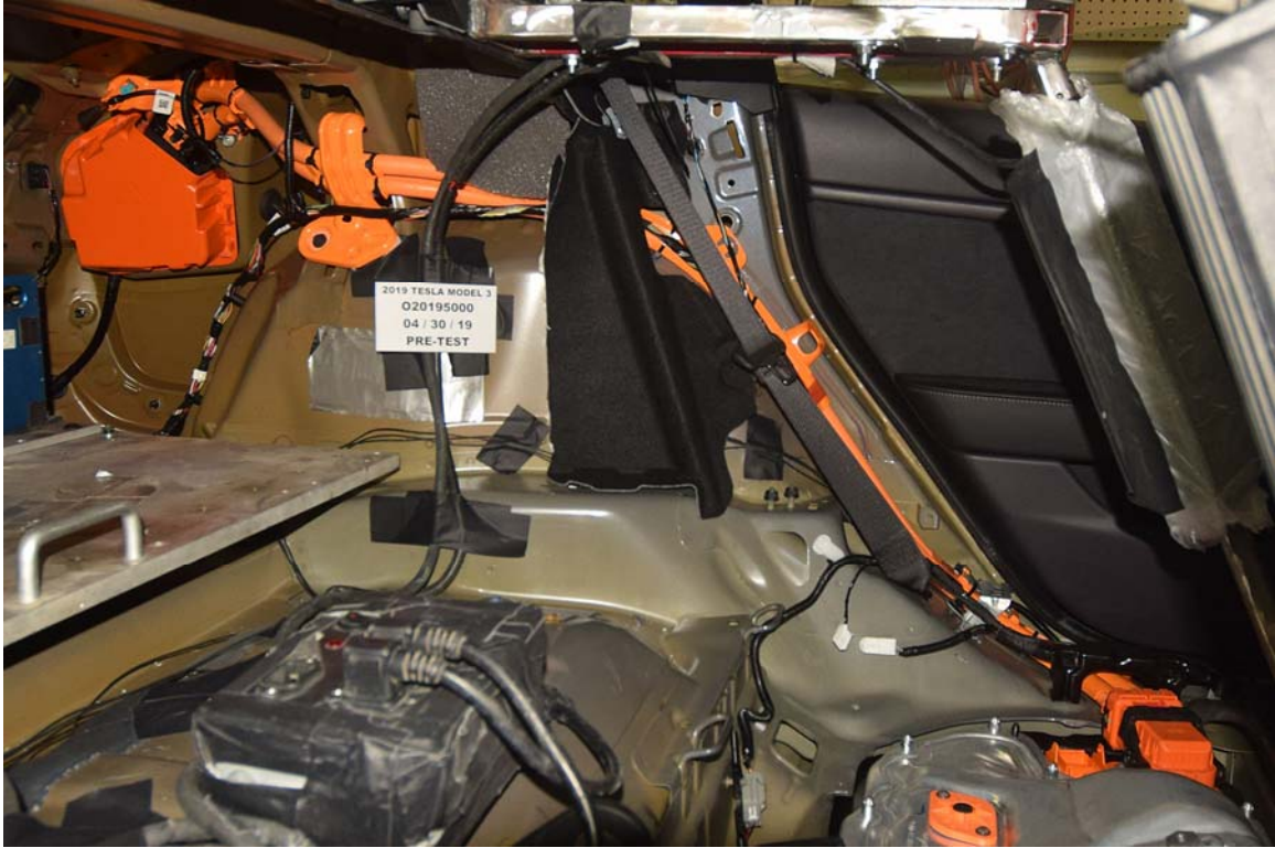
FIGURE 23. Pre-Impact View of High Voltage Interconnect(s)
