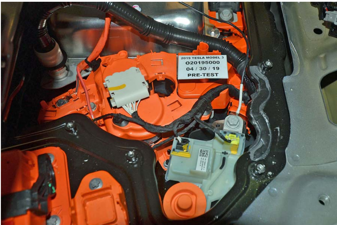
FIGURE 34. Pre-Impact Close-Up View of High Voltage Leads Attached
