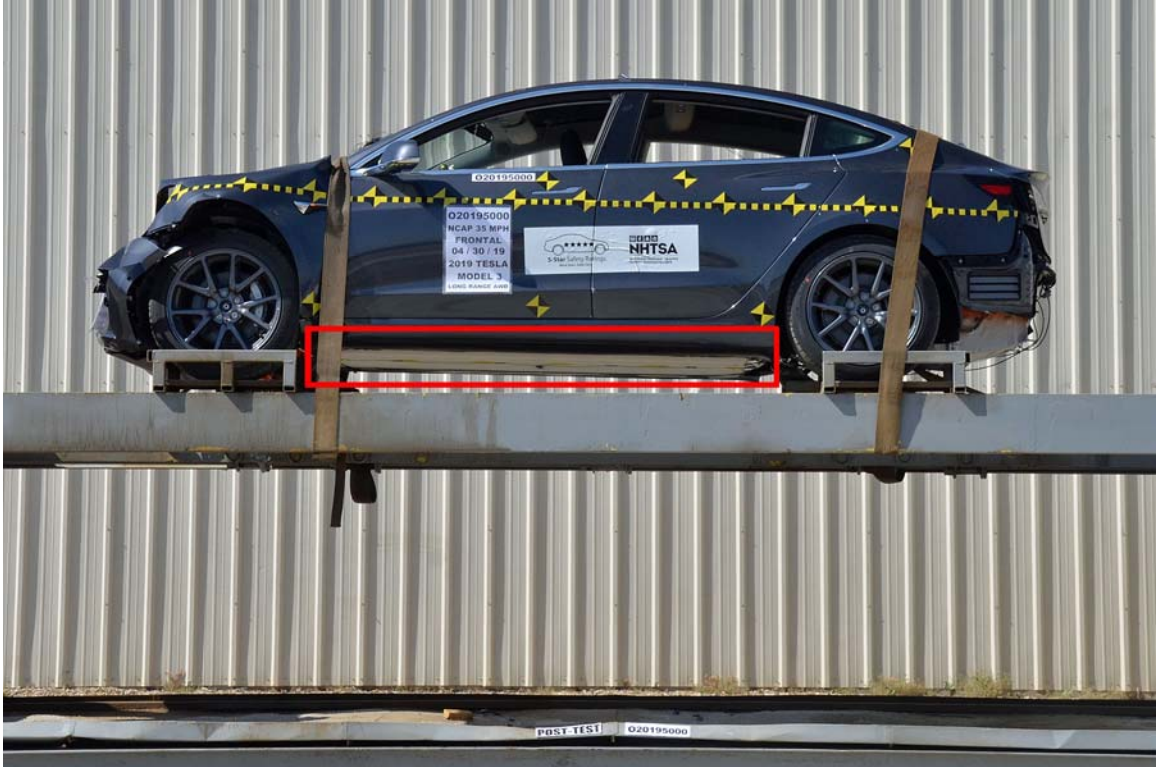
FIGURE 43. FMVSS No. 305 Static Rollover at 360°
