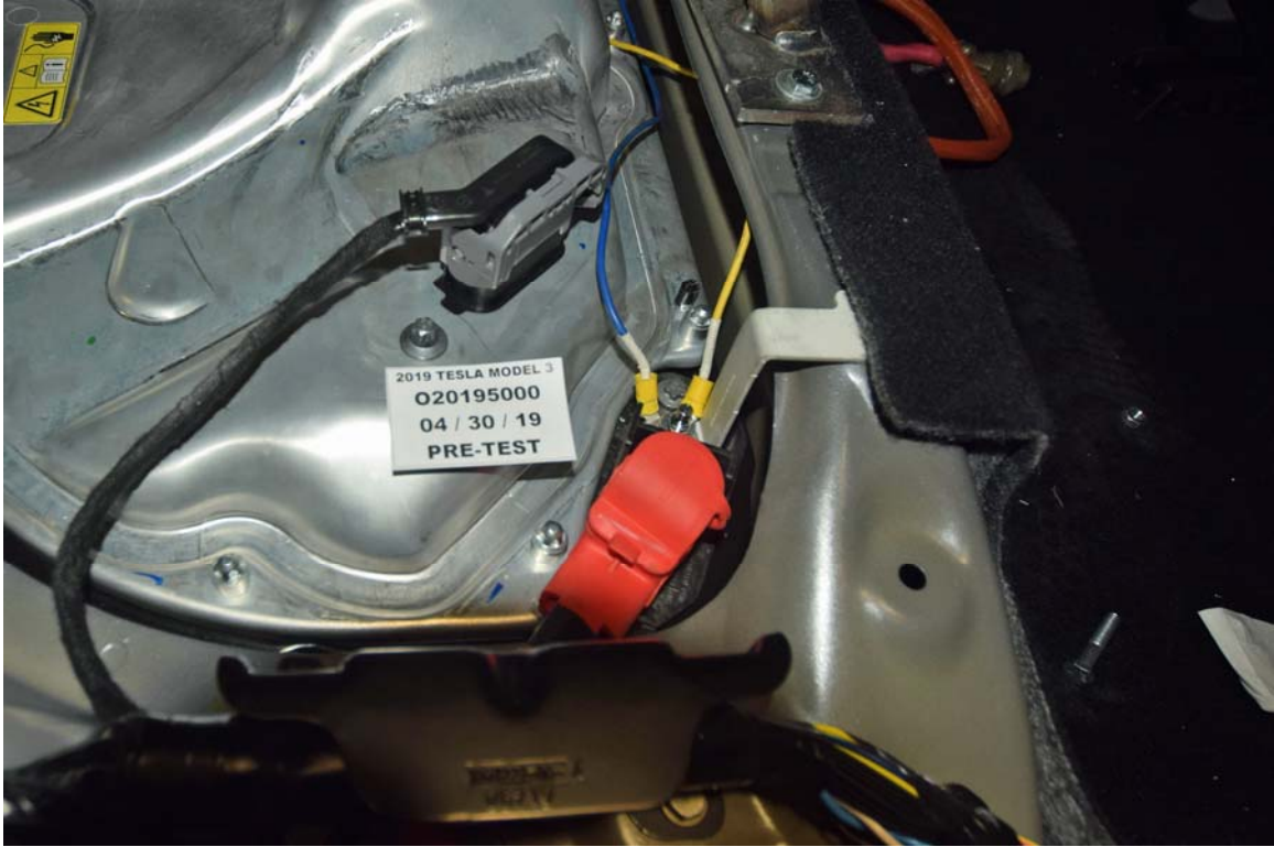
FIGURE 7. Manual High Voltage Service Disconnect in Place
