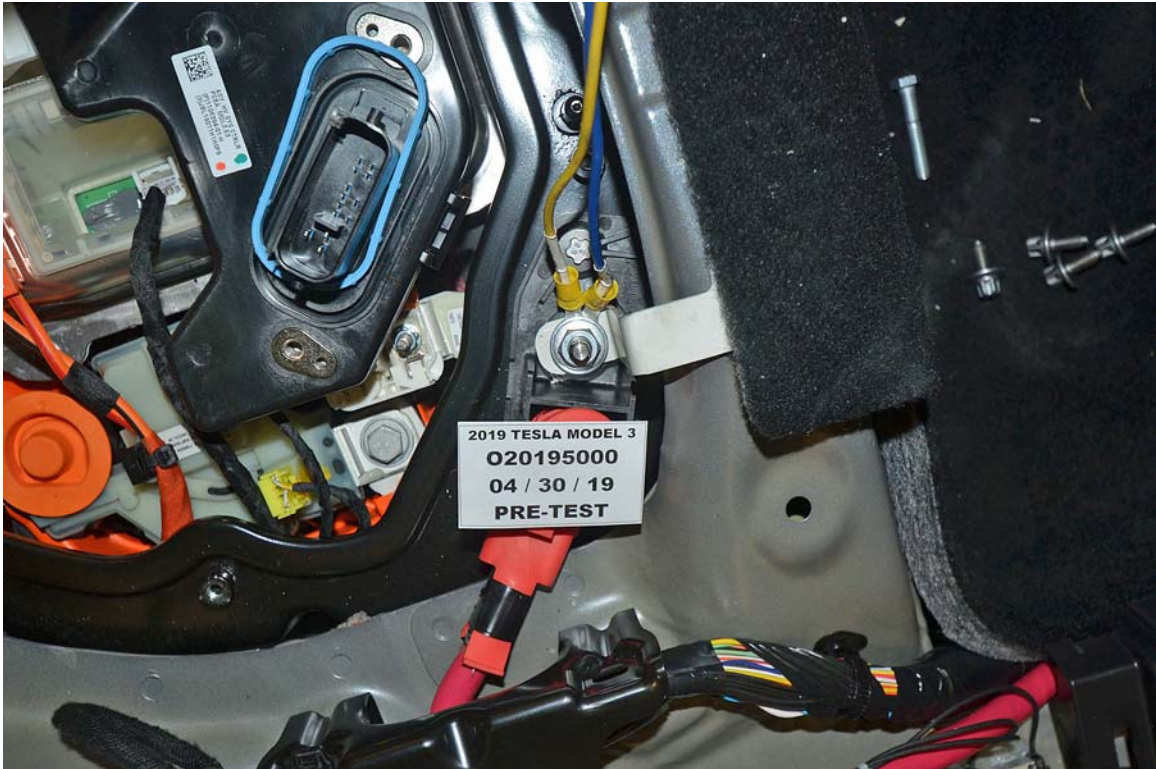
FIGURE 31. Pre-Impact View of Ground Lead Attached
