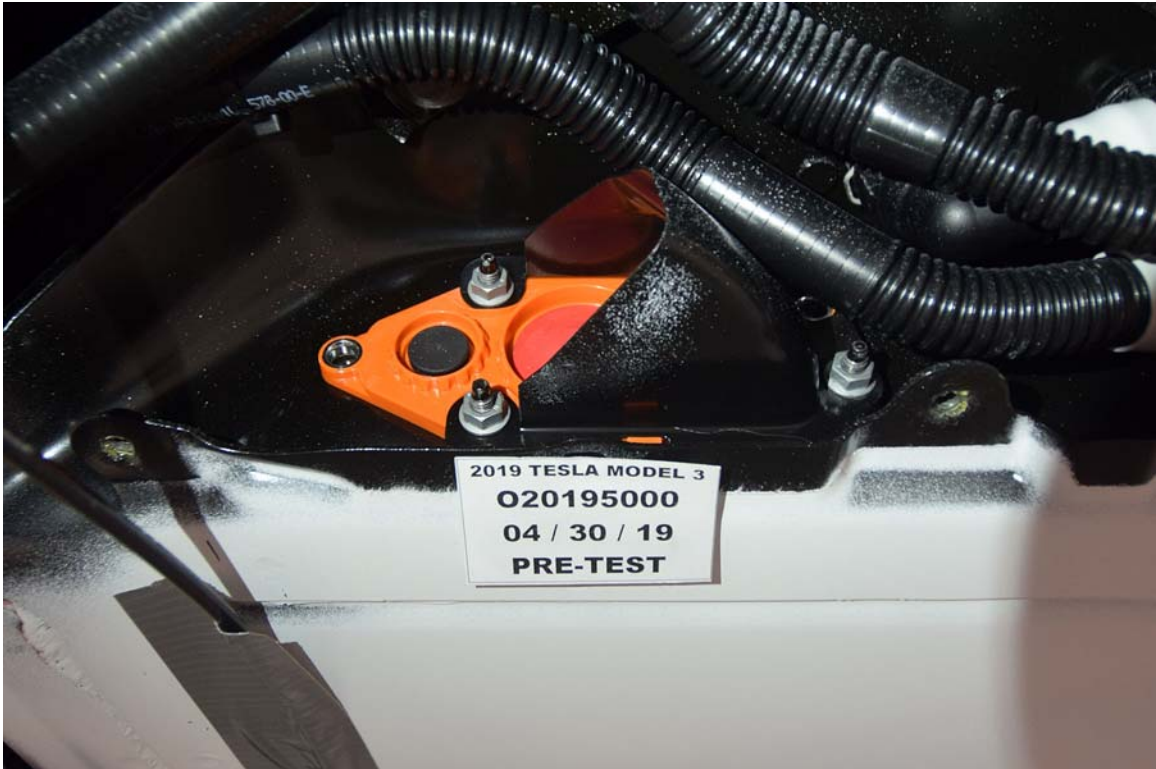
FIGURE 29. Pre-Impact View of Propulsion Battery Venting System(s)
