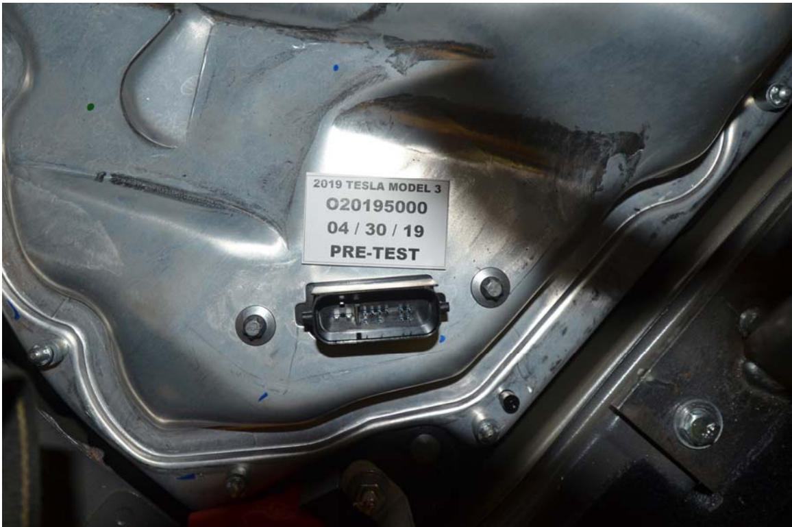
FIGURE 8. Manual High Voltage Service Disconnect Removed
