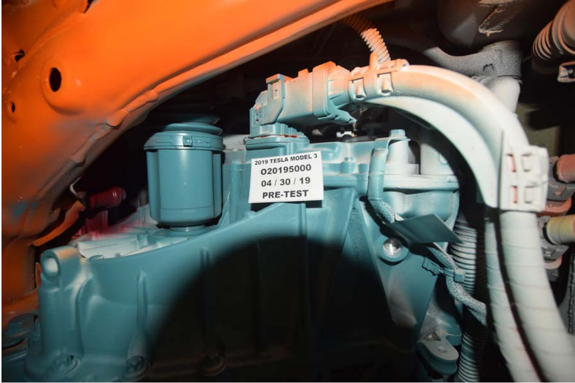
FIGURE 27. Pre-Impact View of High Voltage Interconnect(s)
