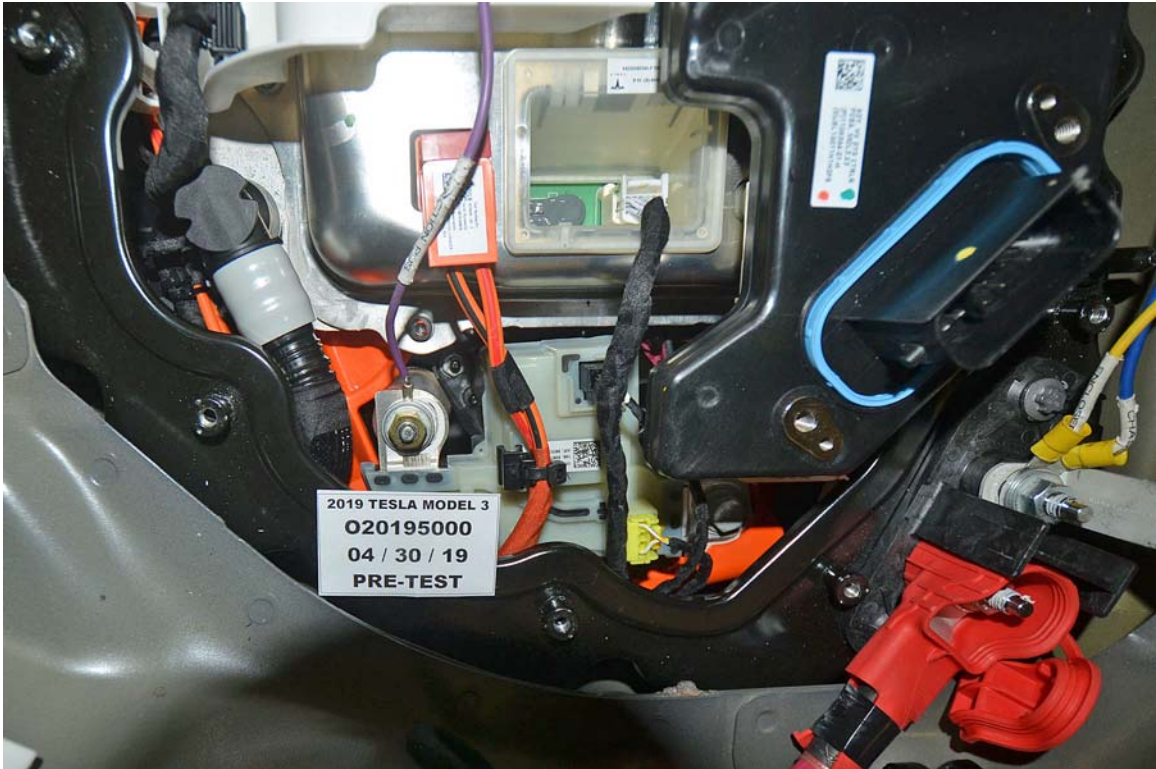
FIGURE 33. Pre-Impact Close-Up View of High Voltage Leads Attached
