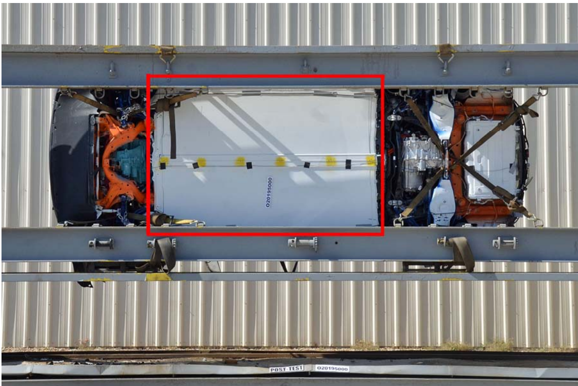
FIGURE 42. FMVSS No. 305 Static Rollover at 270°
