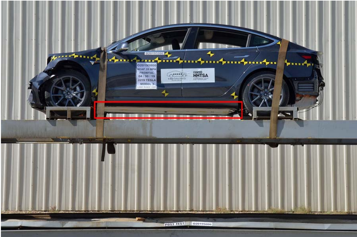
FIGURE 39. FMVSS No. 305 Static Rollover at 0°
