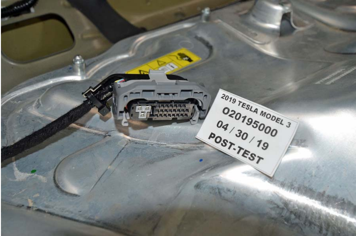
FIGURE 9. Manual High Voltage Service Disconnect Removed
