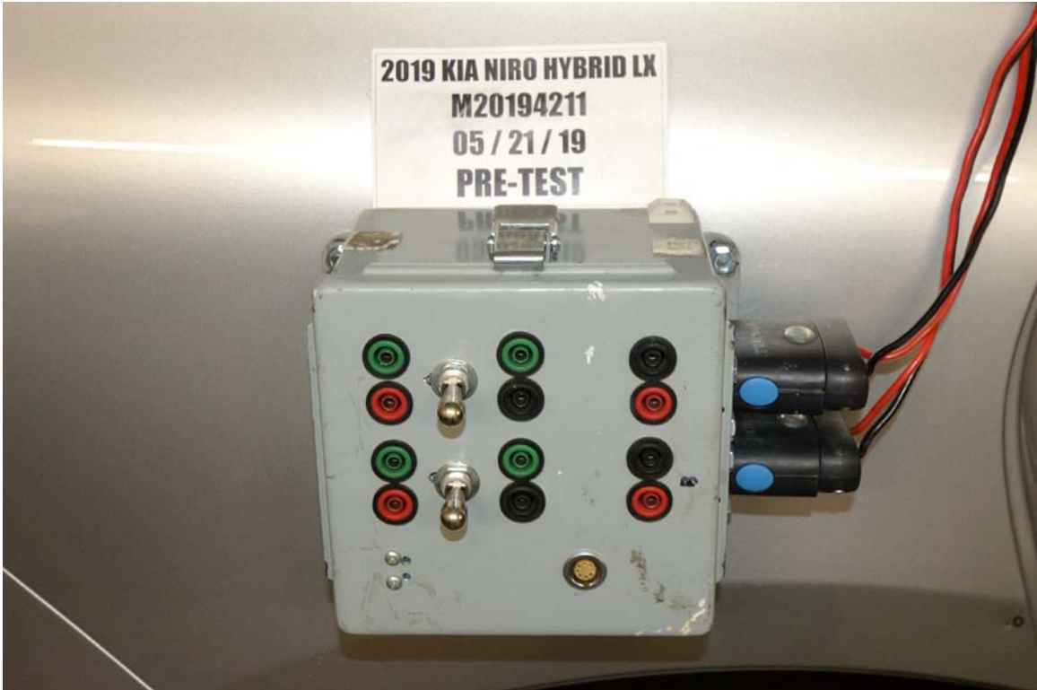
FIGURE 24. Pre-Impact View of Installed Test Interface Port
