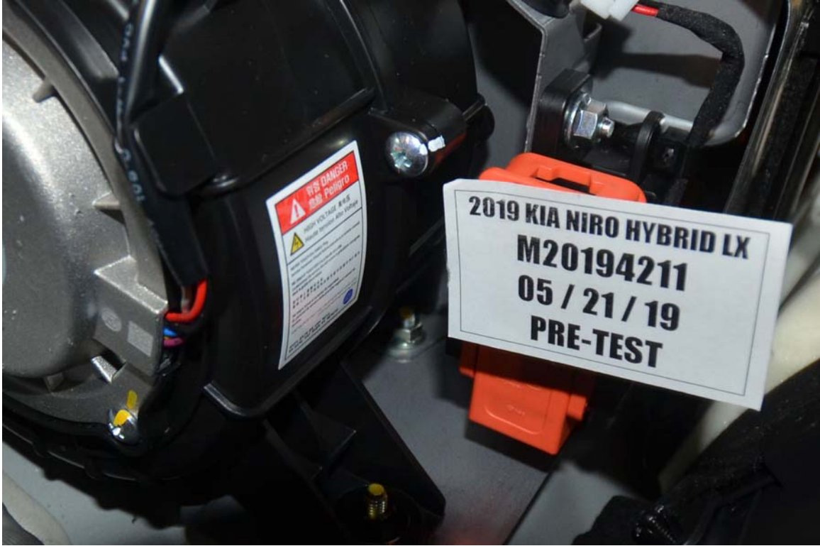
FIGURE 2a. Power Inverter Warning Label
