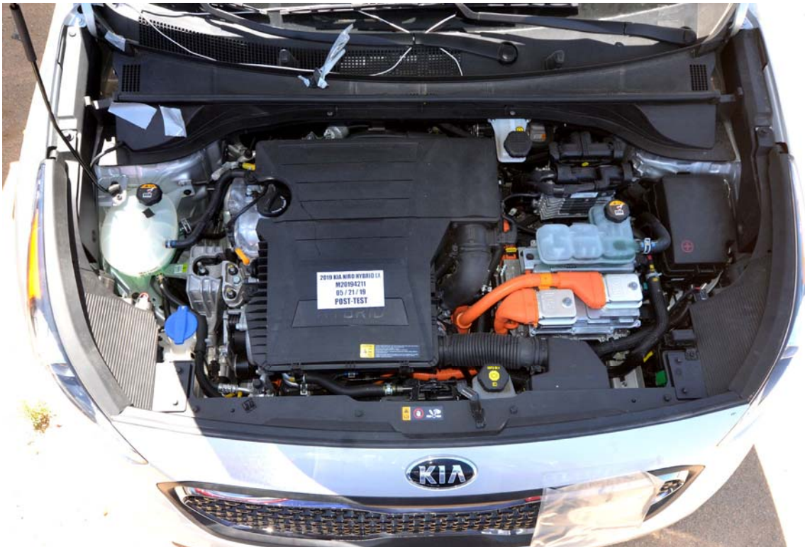
FIGURE 17. Post-Impact View of Electric Propulsion Drive
