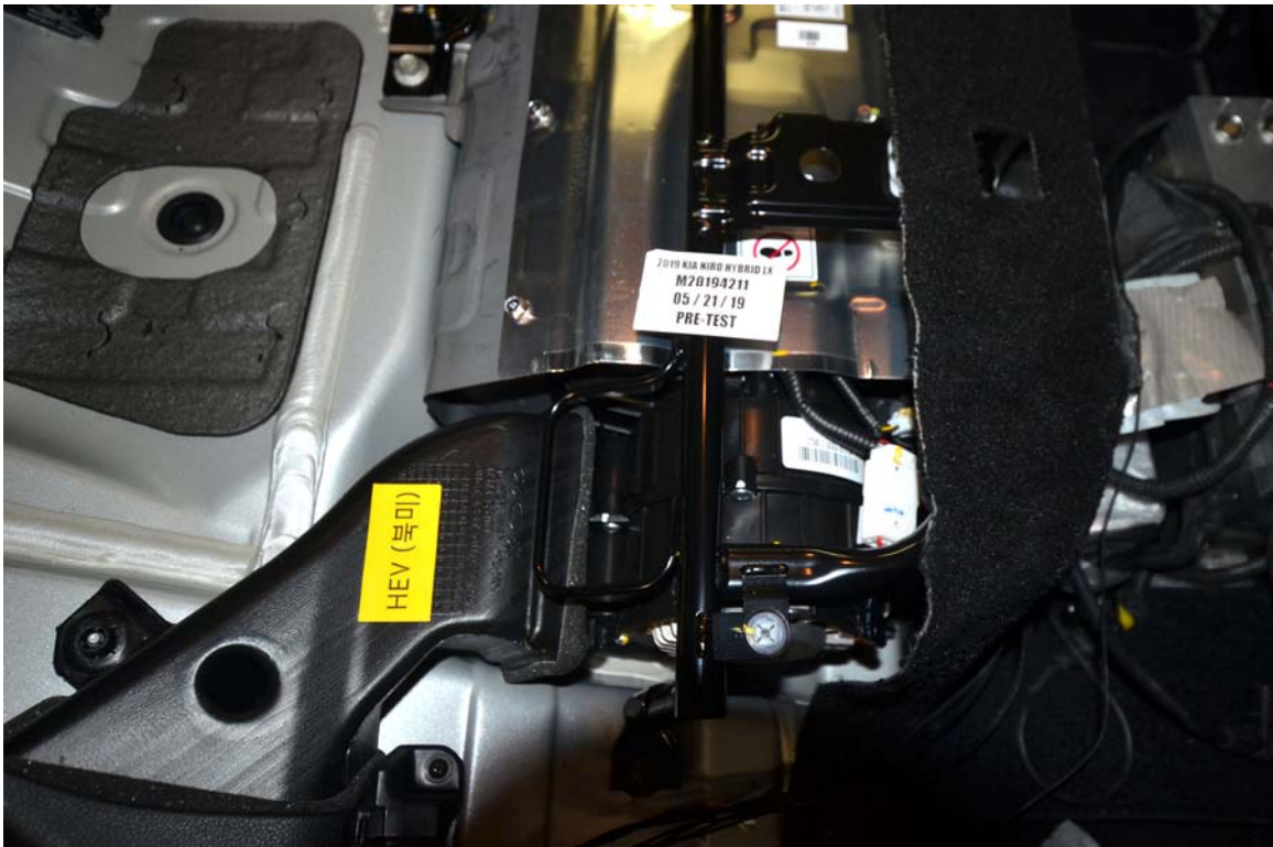
FIGURE 19. Pre-Impact View Propulsion Battery Venting System(s)
