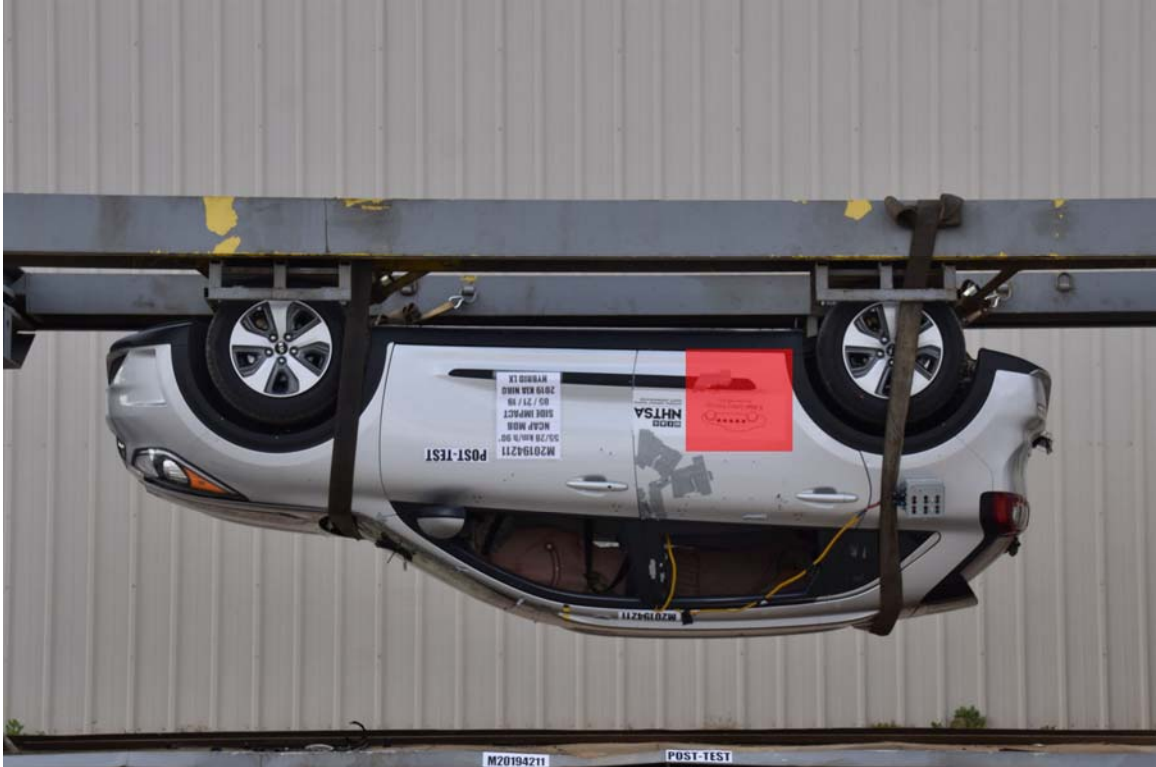
FIGURE 30. FMVSS No. 305 Static Rollover at 180°
