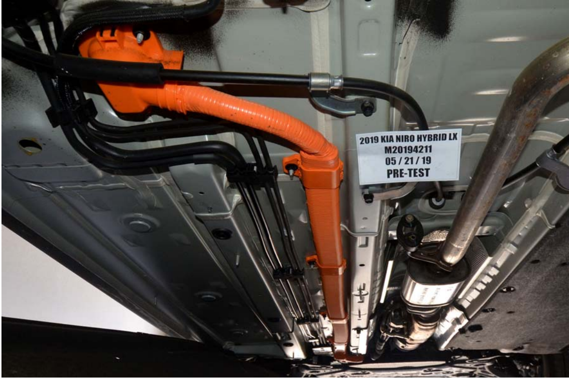
FIGURE 18. Pre-Impact View of High Voltage Interconnect(s)
