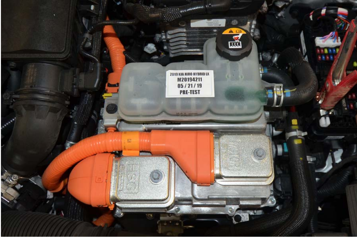
FIGURE 16. Pre-Impact View of Electric Propulsion Drive
