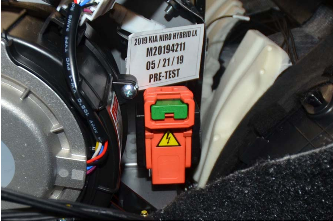
FIGURE 6. Manual High Voltage Service Disconnect in Place
