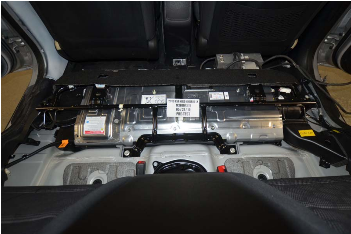
FIGURE 9. Pre-Impact View of Propulsion Battery
