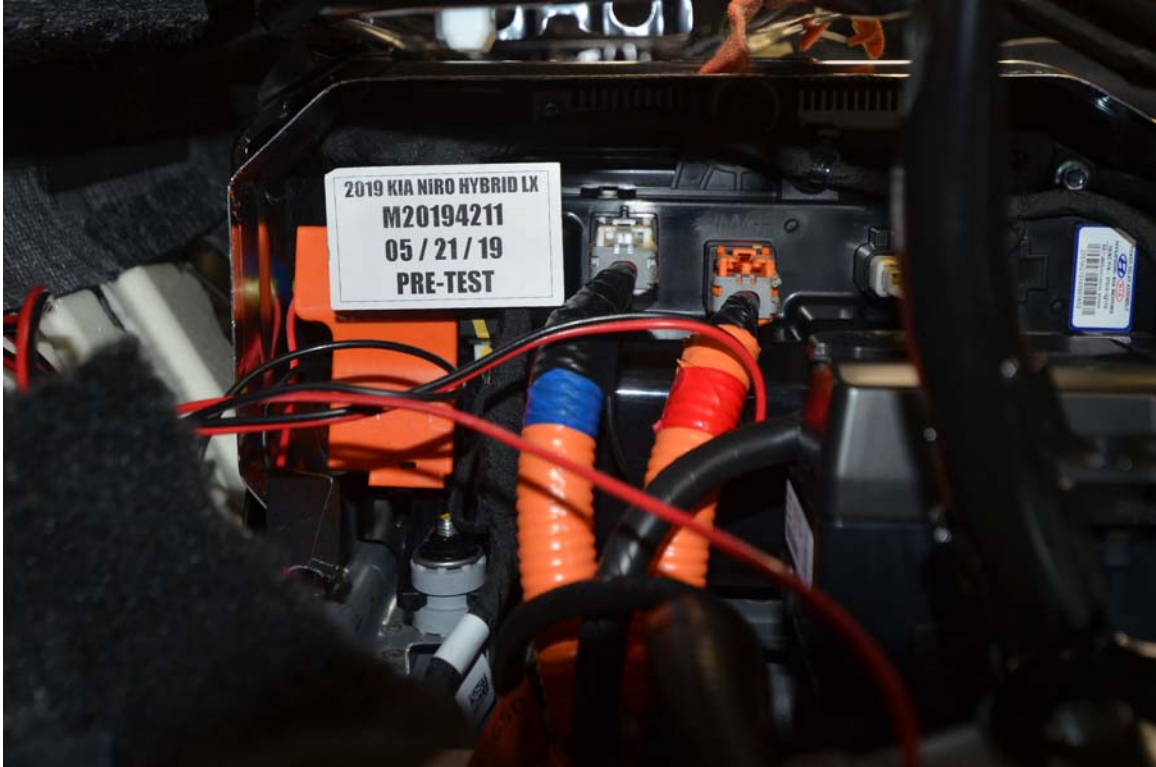
FIGURE 22. Pre-Impact View of High Voltage Leads Attached
