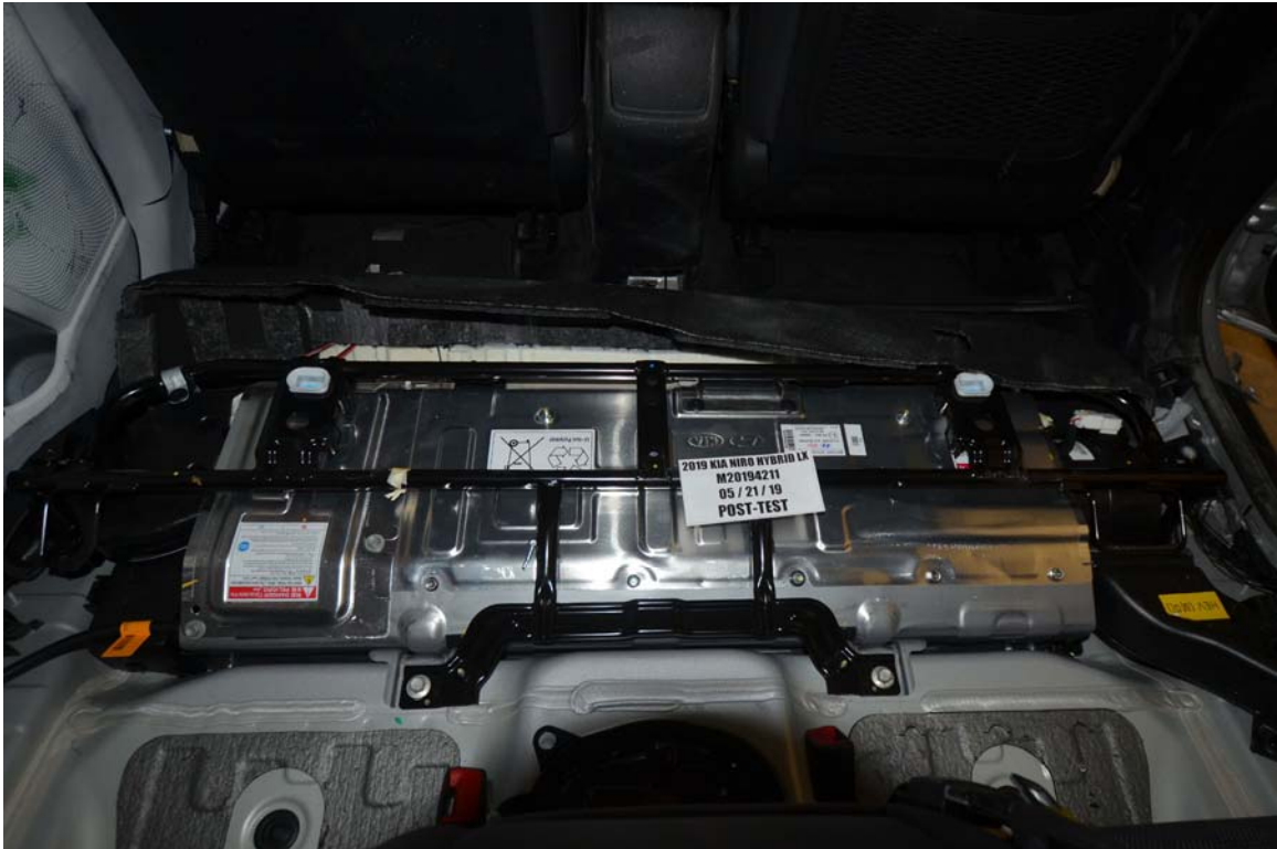
FIGURE 11. Post-Impact Rear View of Propulsion Battery
