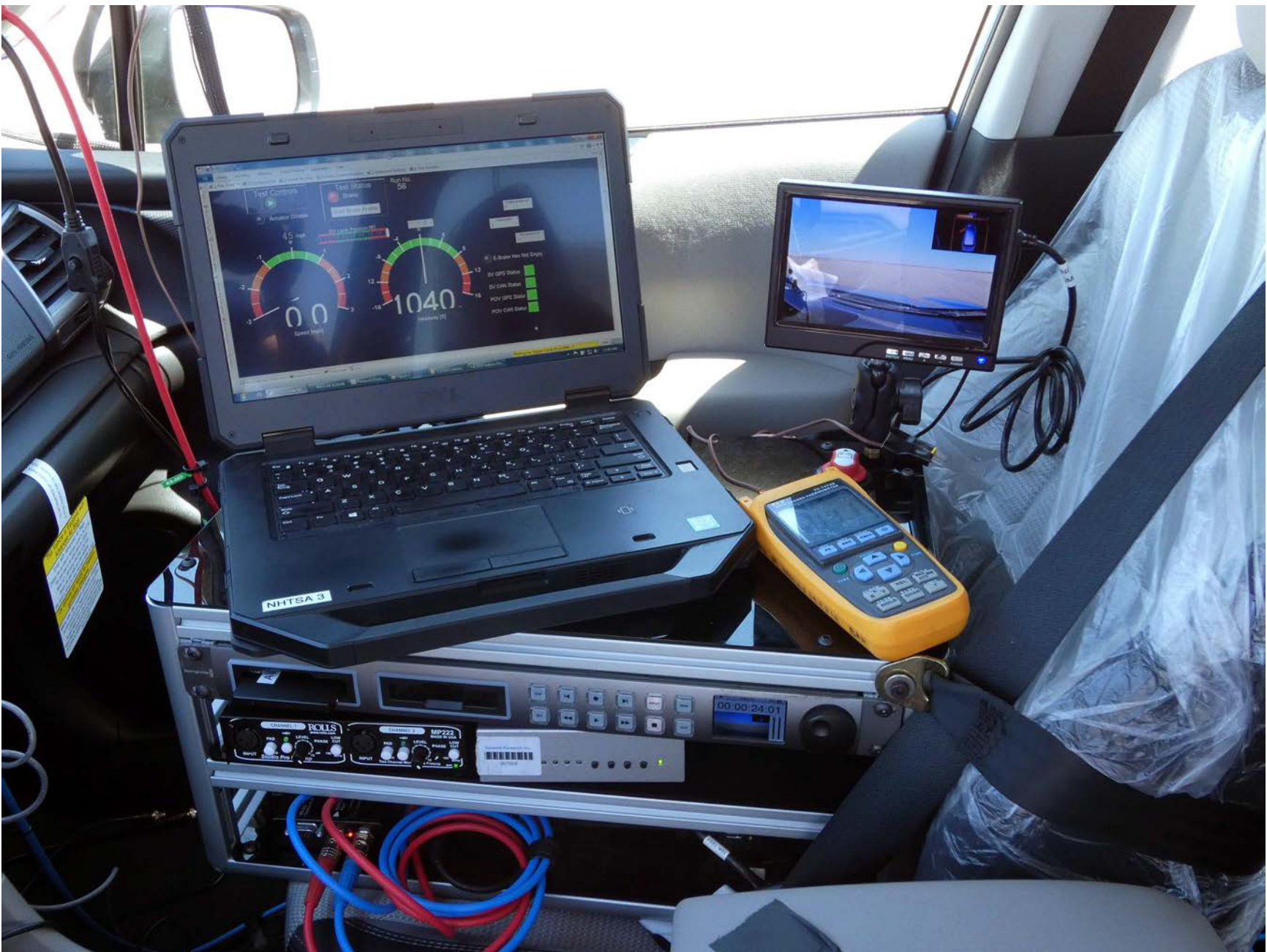
Figure A13. Computer Installed in Subject Vehicle
