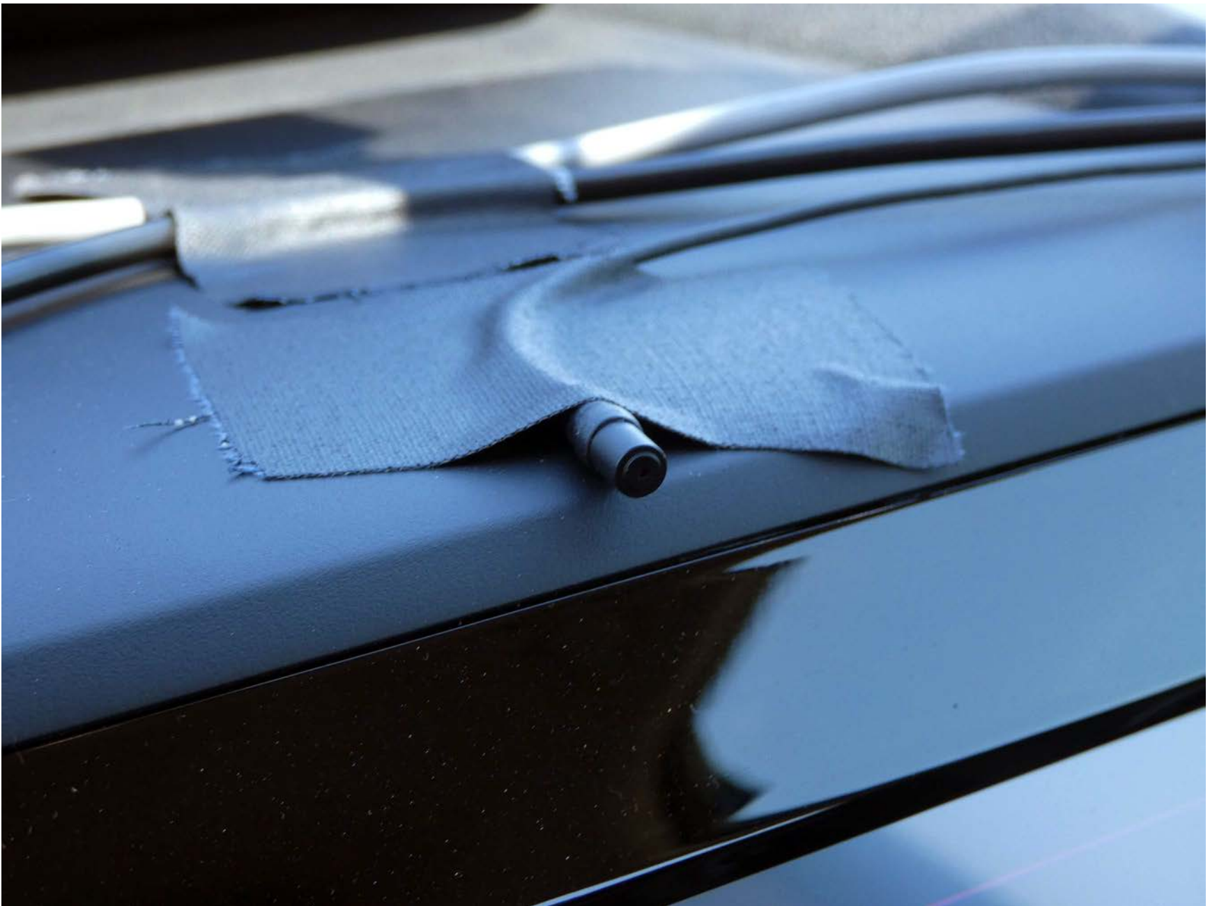
Figure A11. Sensor for Detecting Auditory Alerts
