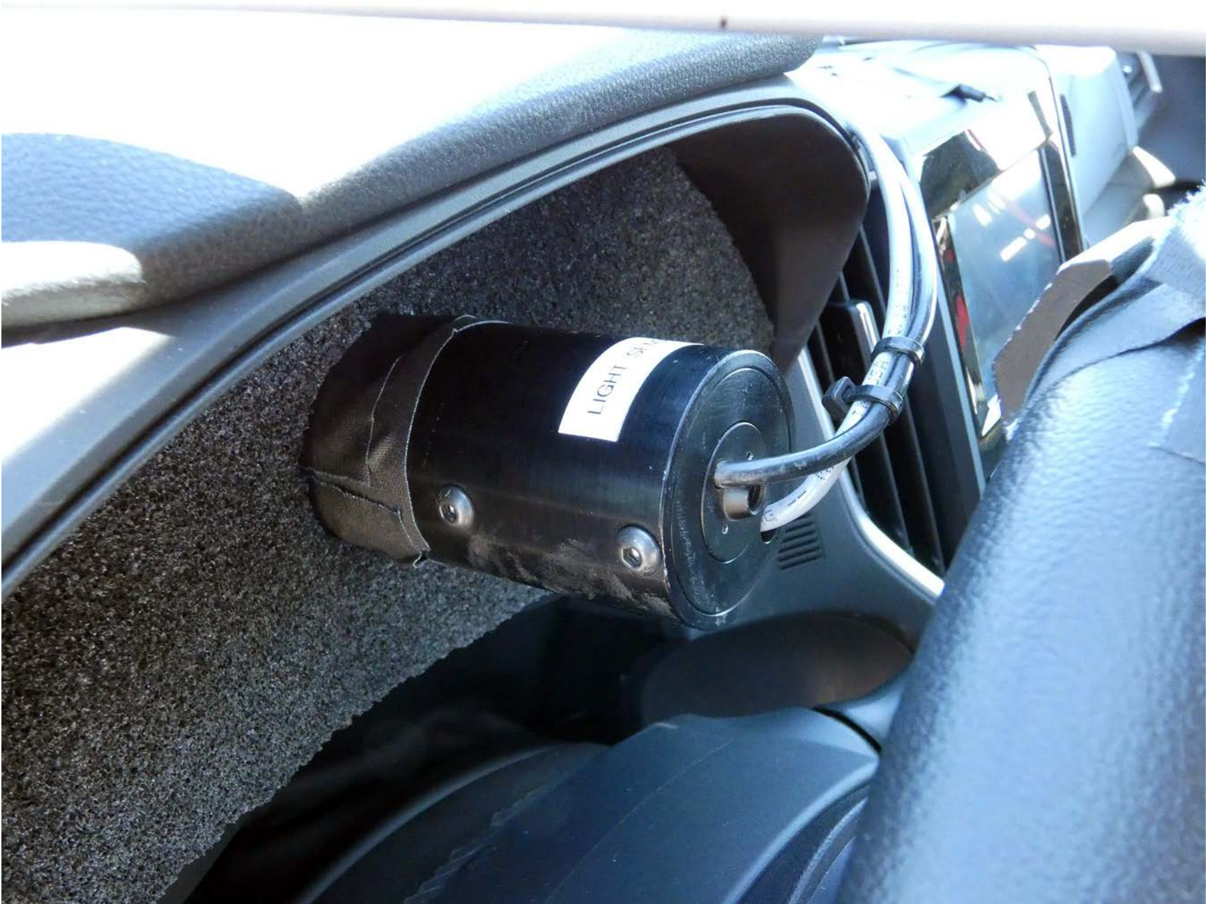
Figure A12. Sensor for Detecting Visual Alert
