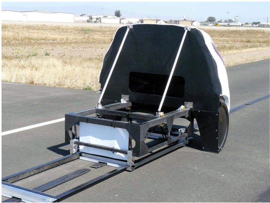
Figure A7. Load Frame/Slider of SSV
