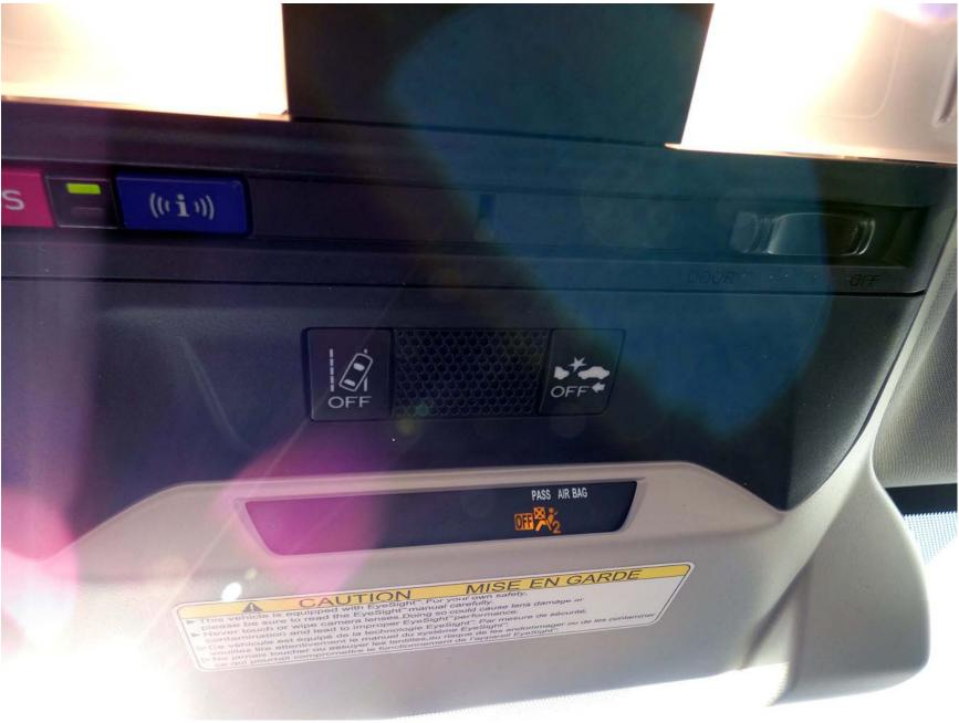
Figure A16. AEB On/Off Switch
