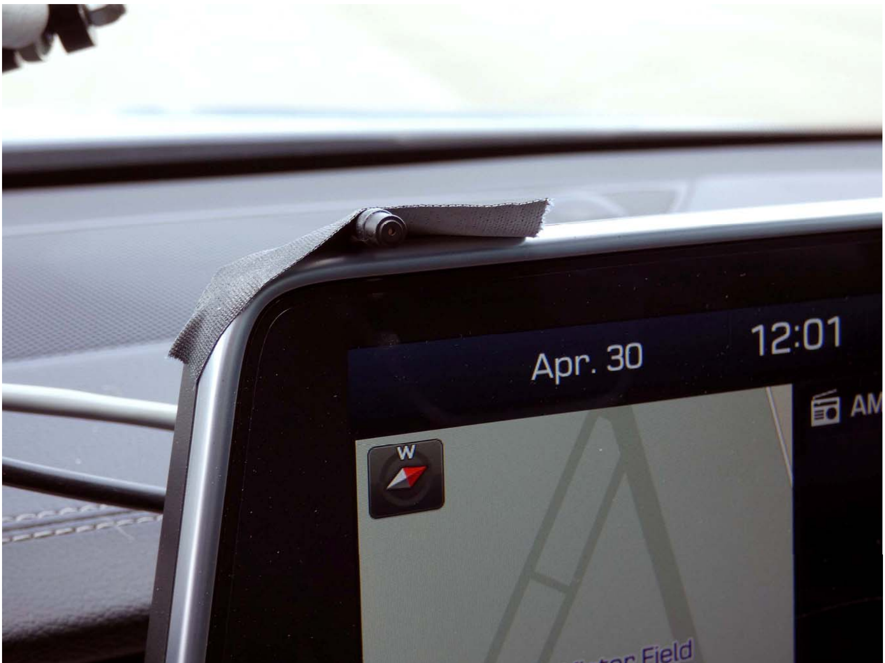
Figure A11. Sensor for Detecting Auditory Alerts
