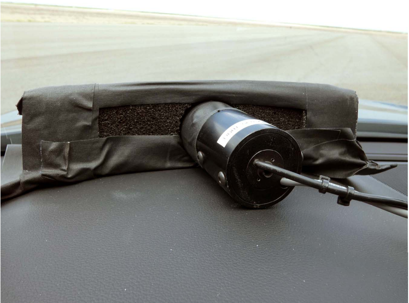
Figure A12. Sensor for Detecting Visual Alert
