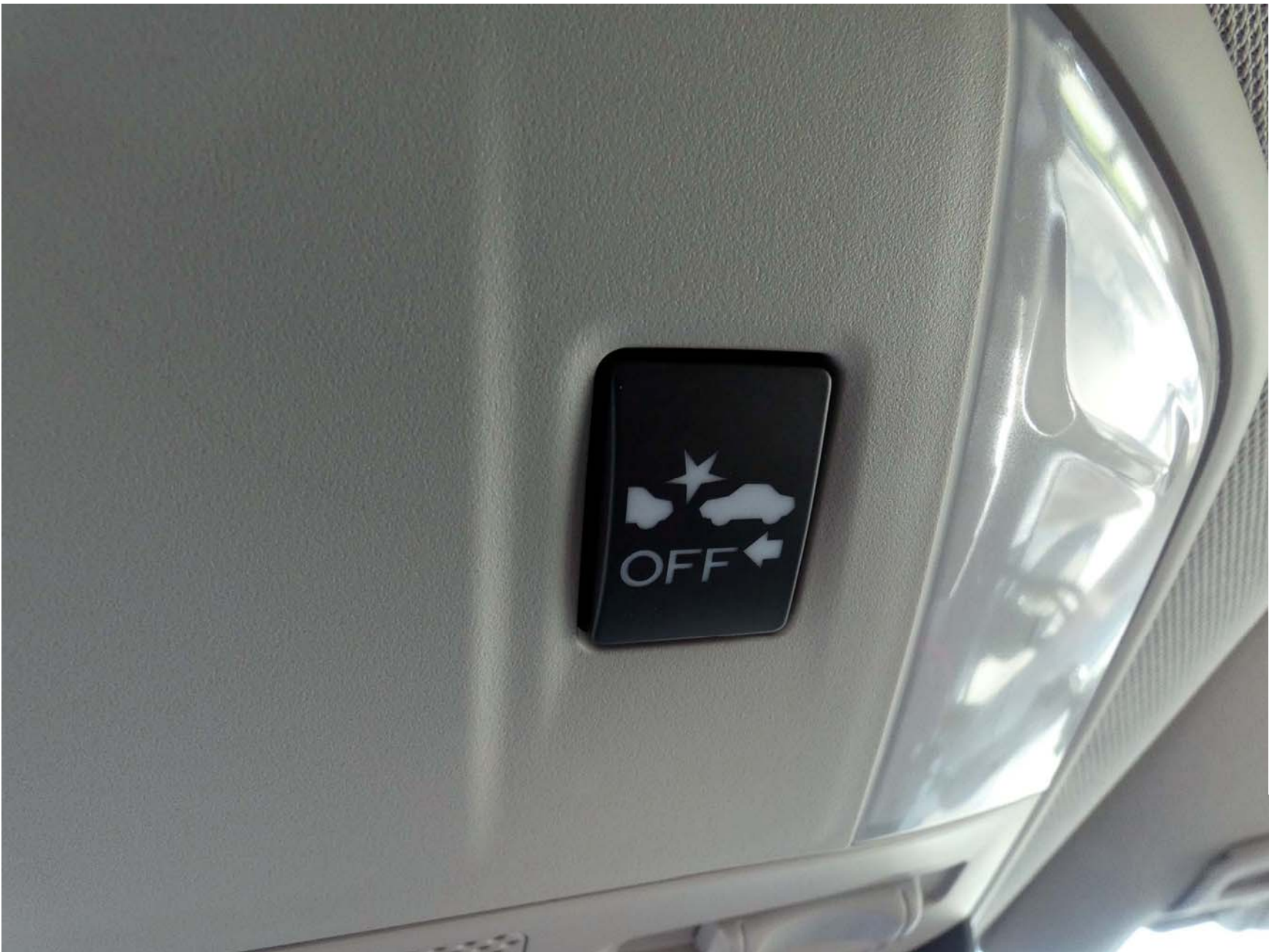
Figure A18. AEB On/Off Switch
