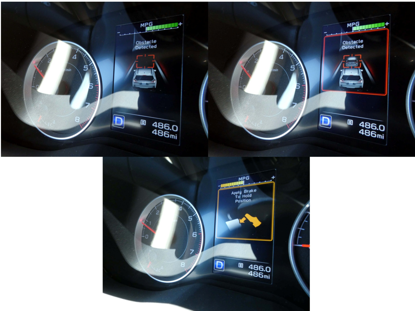
Figure A16. AEB Instrument Panel Visual Alert
