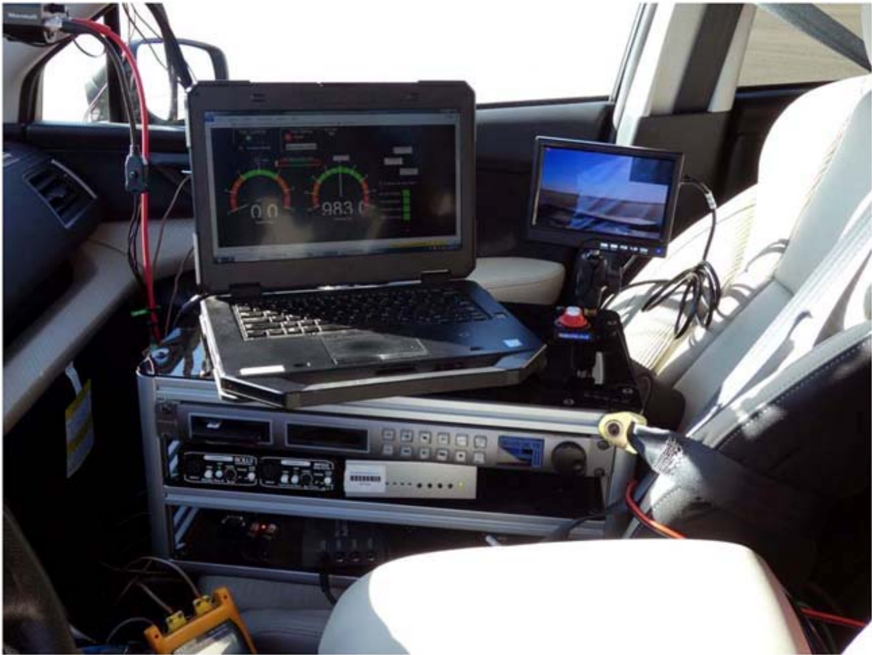
Figure A13. Computer Installed in Subject Vehicle
