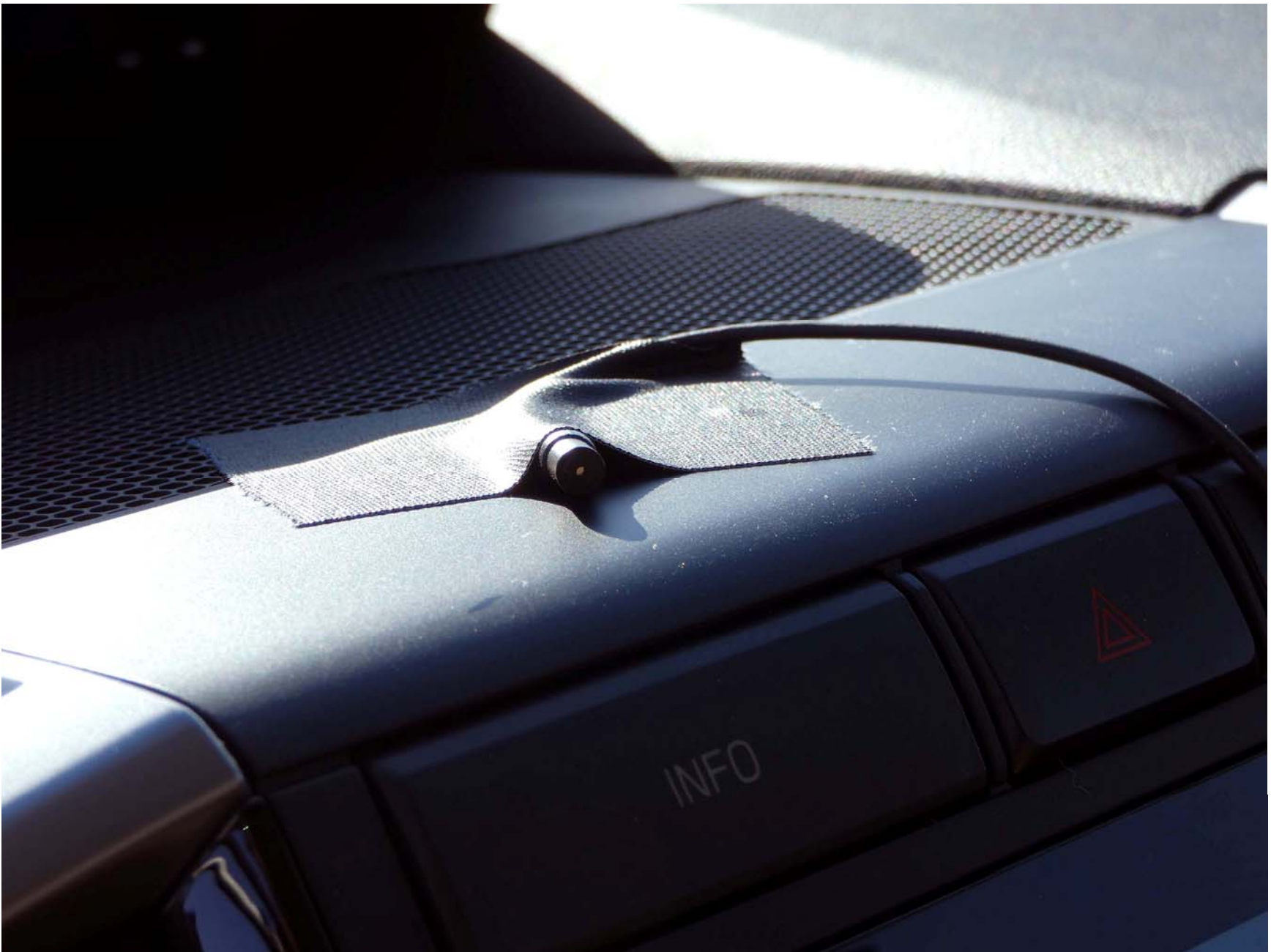
Figure A11. Sensor for Detecting Auditory Alerts
