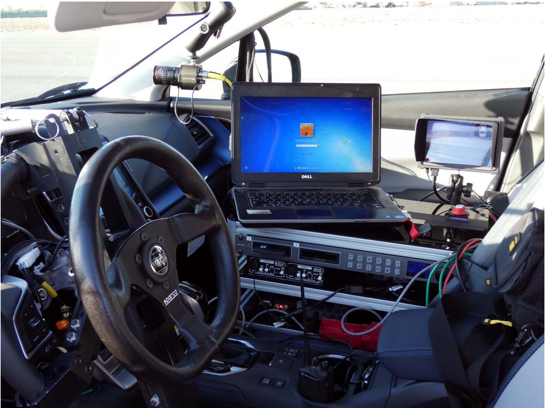
Figure A13. Computer Installed in Subject Vehicle
