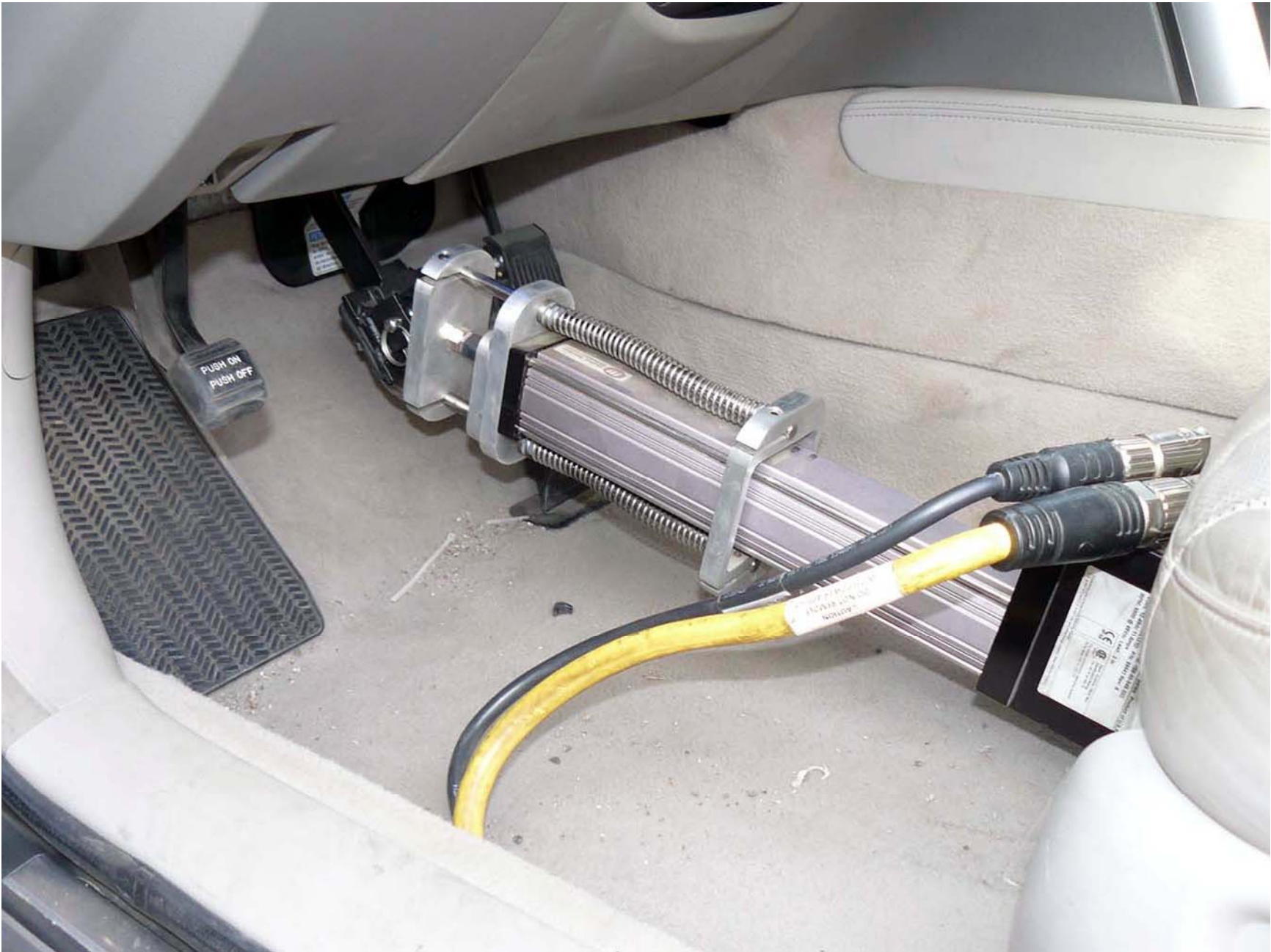
Figure A15. Brake Actuator Installed in POV System
