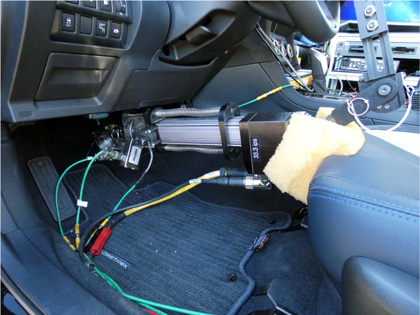
Figure A14. Brake Actuator Installed in Subject Vehicle
