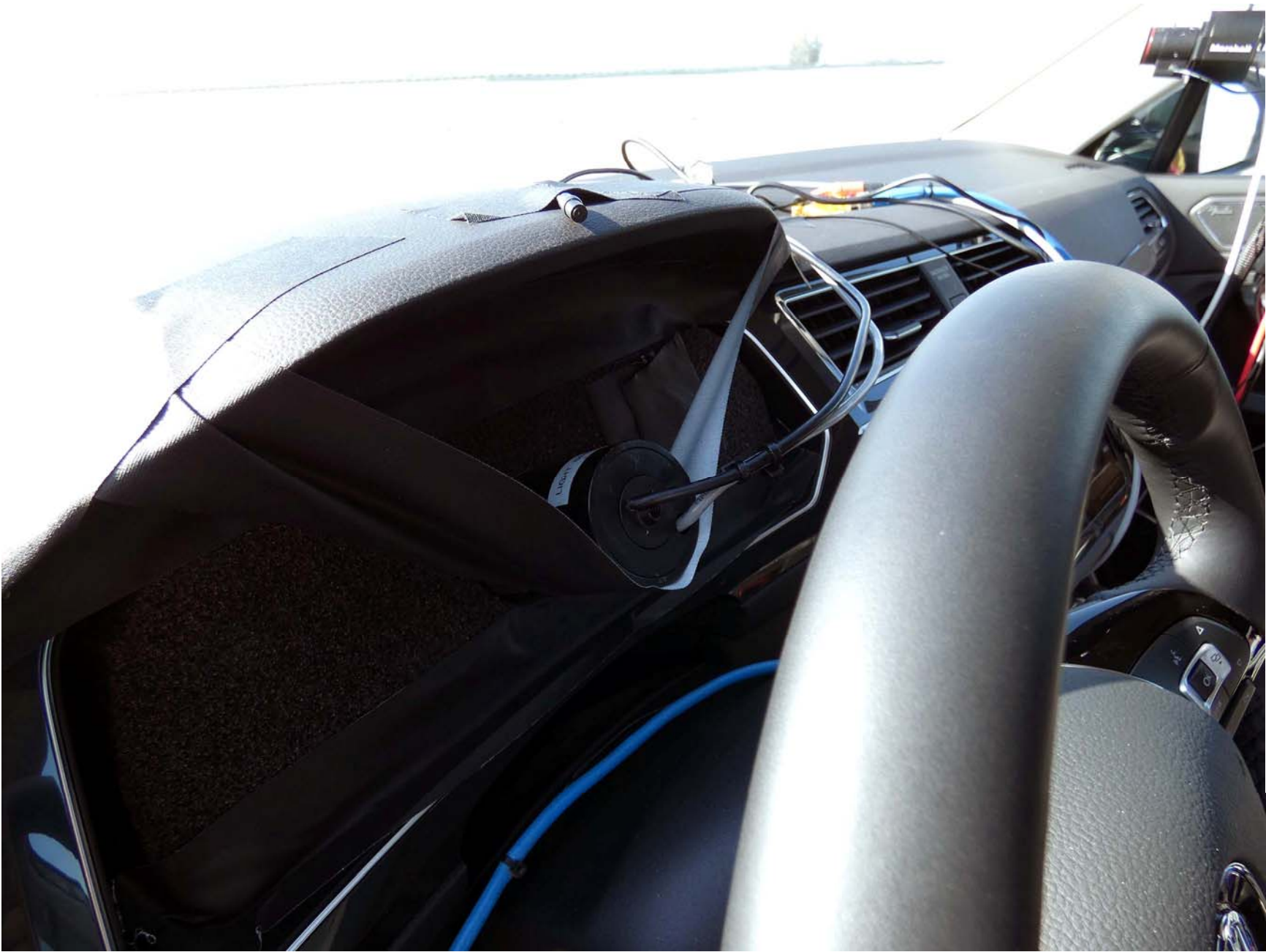
Figure A8. Sensor for Detecting Visual Alerts
