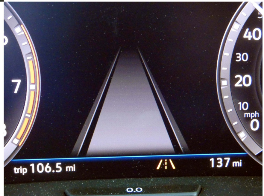
Figure A9. LDW Instrument Panel Visual Alerts
