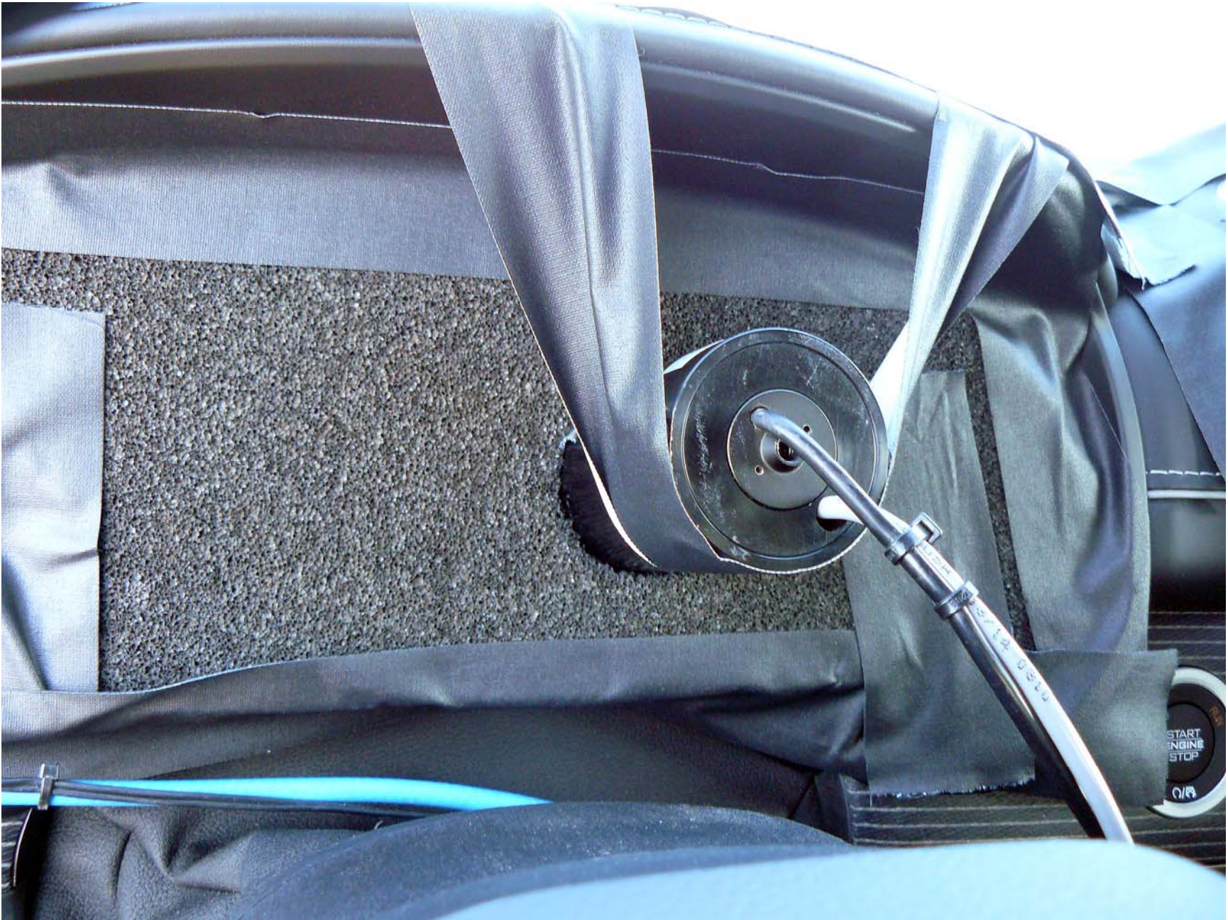
Figure A8. Sensor for Detecting Auditory Alerts
