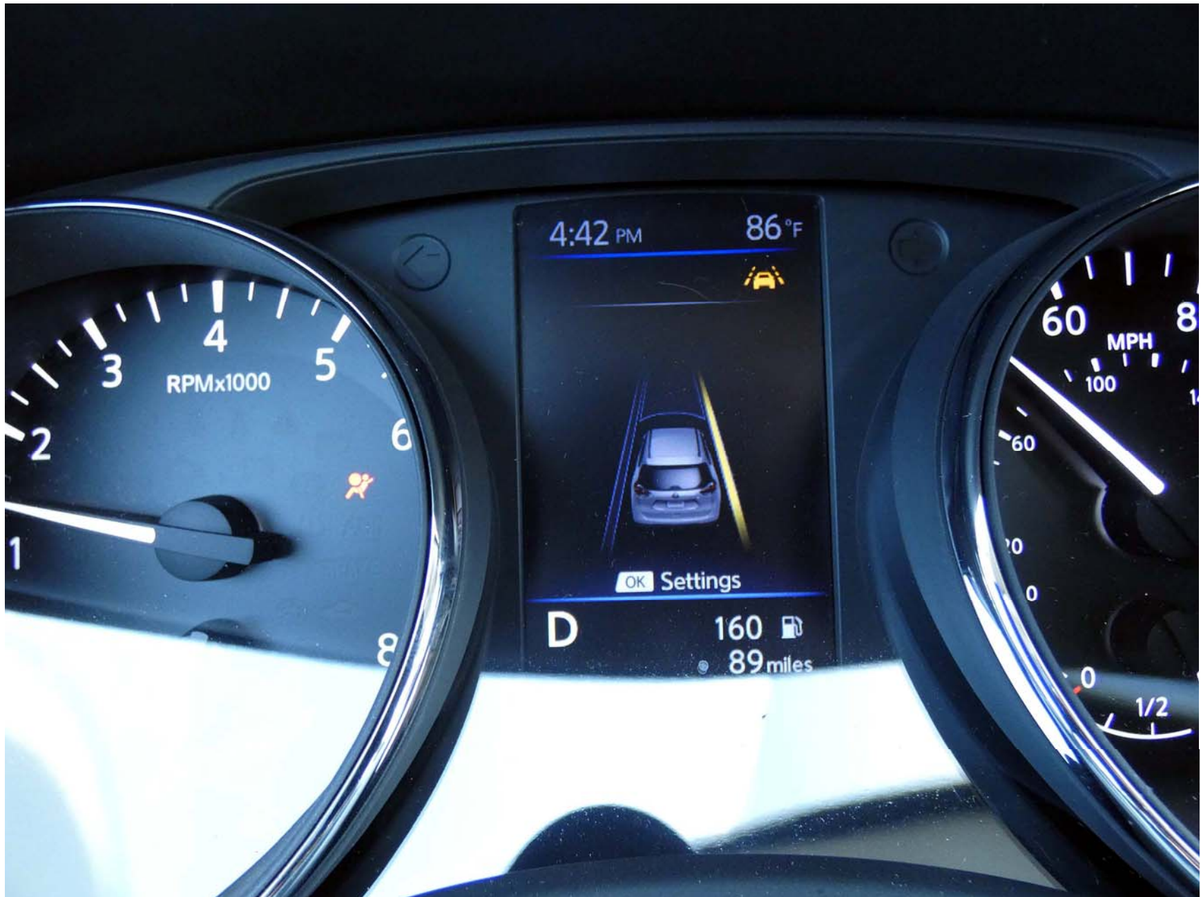
Figure A10. LDW Instrument Panel Visual Alerts
