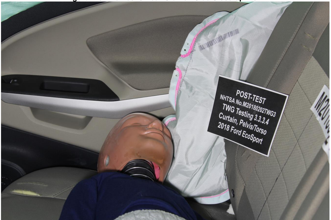
Figure A-6: Post-Test 3-Year-Old Left Side Close-up View
