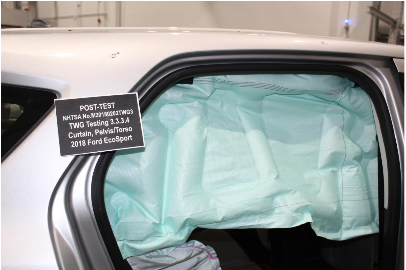
Figure A-13: Post-Test Curtain Airbag View
