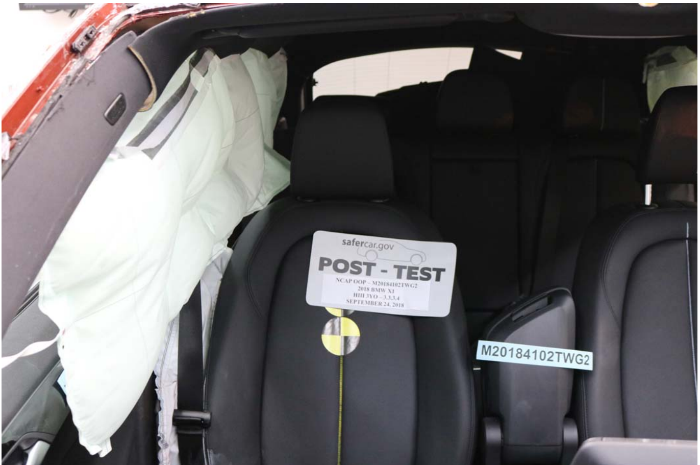
Photo No. 024 - Post-Test Curtain Airbag Front View
