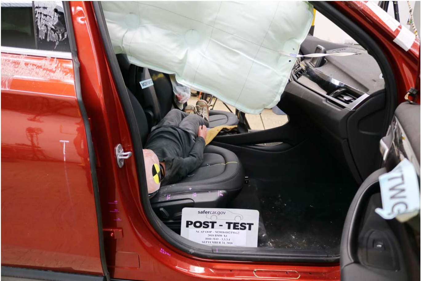
Photo No. 021 - Post-Test 3-Year-Old Child Dummy Right Side View (Door Open)
