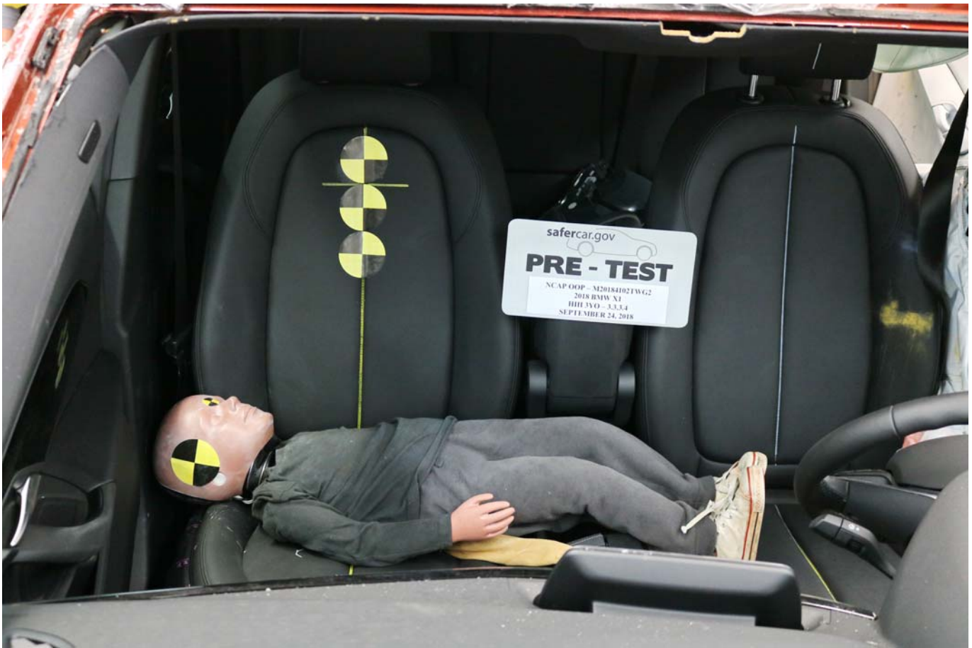
Photo No. 013 - Pre-Test 3-Year-Old Child Dummy Front View
