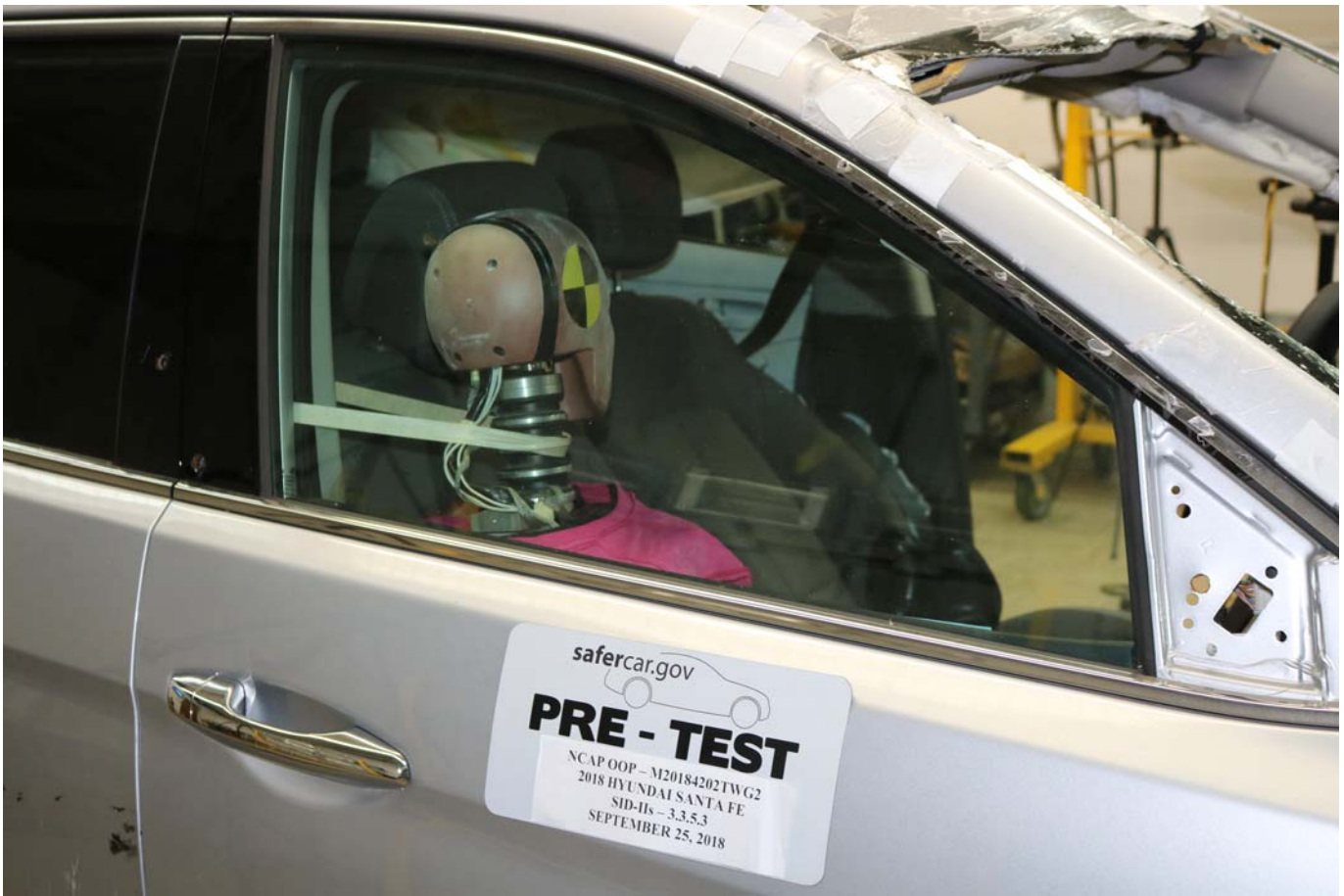
Photo No. 017 - Pre-Test SID-Its Right Three-Quarter Front View
