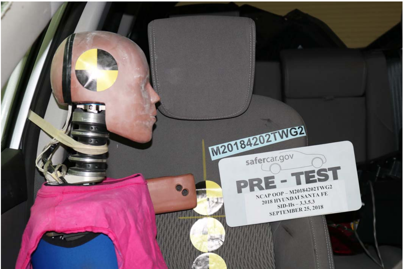
Photo No. 015 - Pre-Test SID-IIs Front Close-Up View
