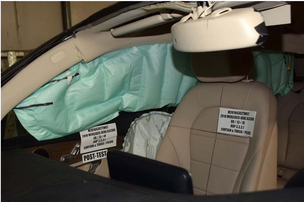
FIGURE 18. Post-Test Airbags, Left Front 3/4 View
