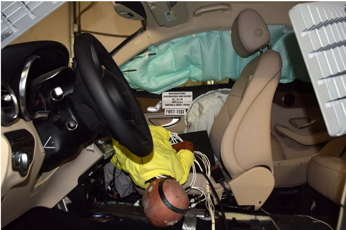
FIGURE 8. Post-Test Dummy Position, Left View
