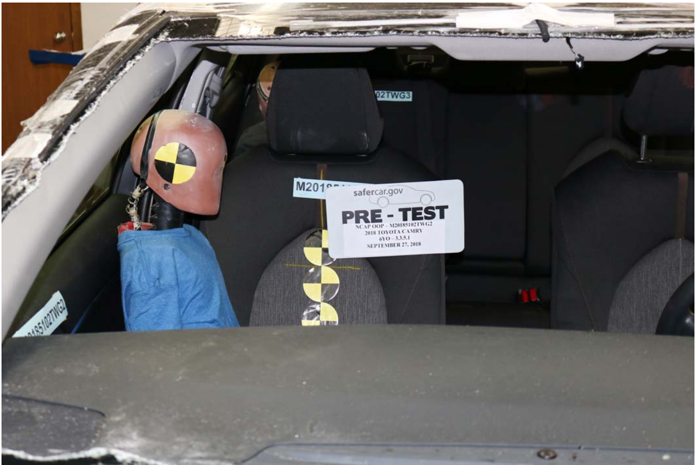
Photo No. 013 - Pre-Test 6-Year-Old Child Dummy Front View
