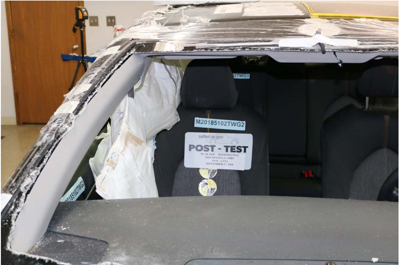
Photo No. 024 - Post-Test Curtain Airbag Front View
