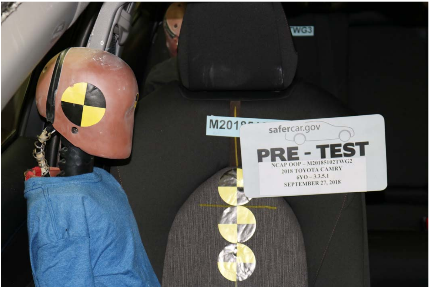
Photo No. 015 - Pre-Test 6-Year-Old Child Dummy Front Close-Up View
