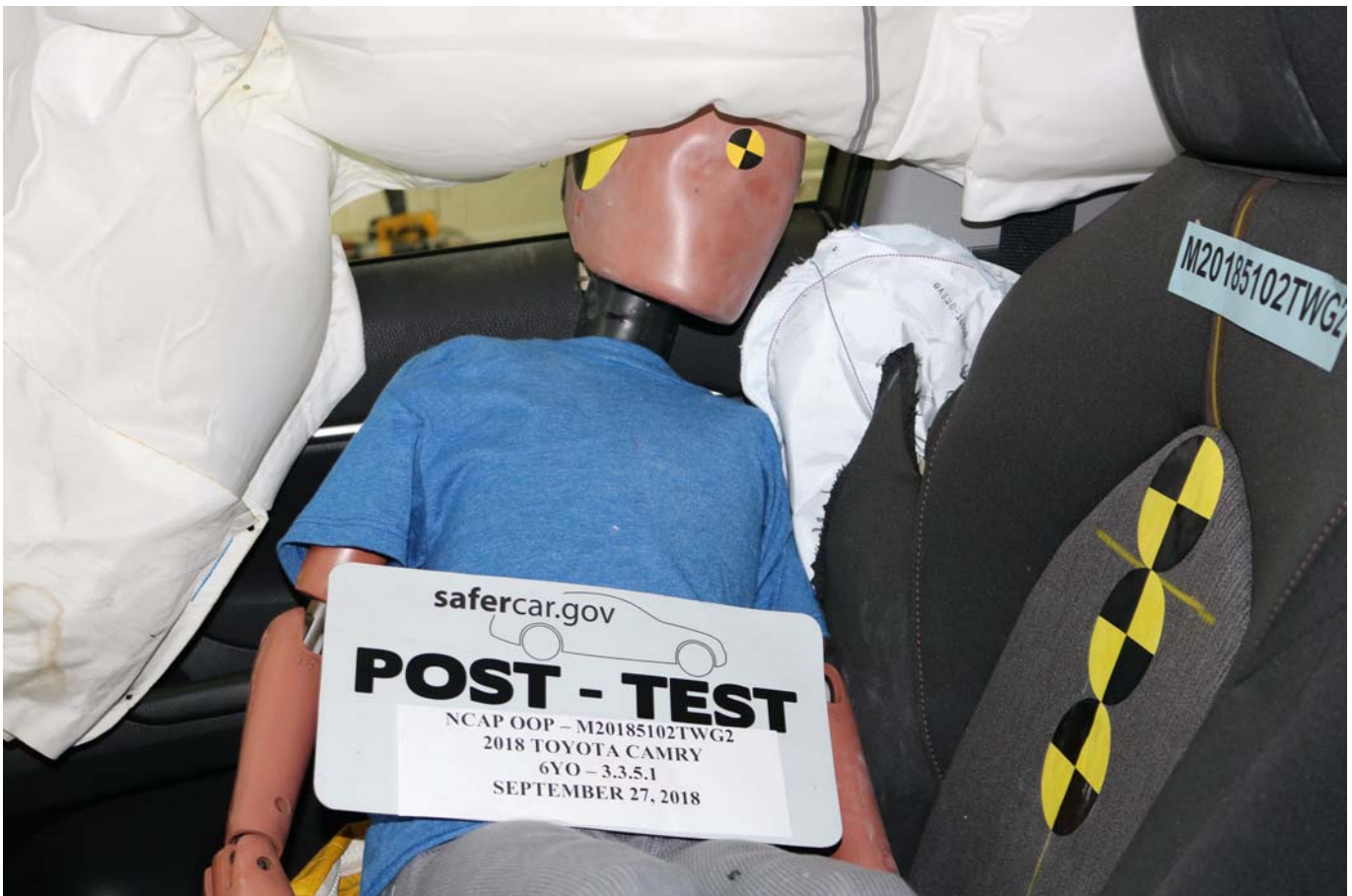
Photo No. 008 - Post-Test 6-Year-Old Child Dummy Left Side Close-Up View
