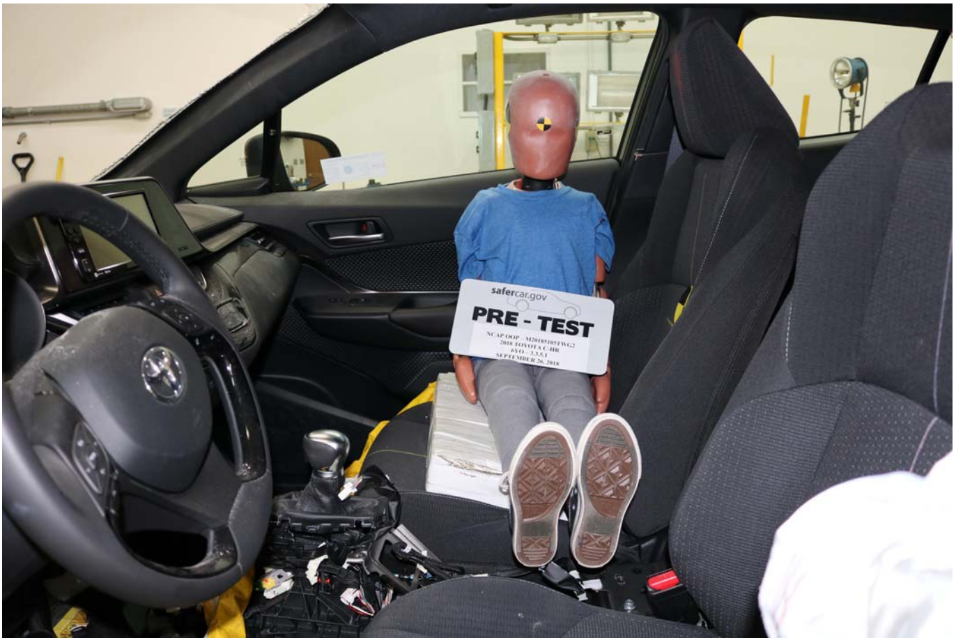
Photo No. 005 - Pre-Test 6-Year-Old Child Dummy Left Side View
