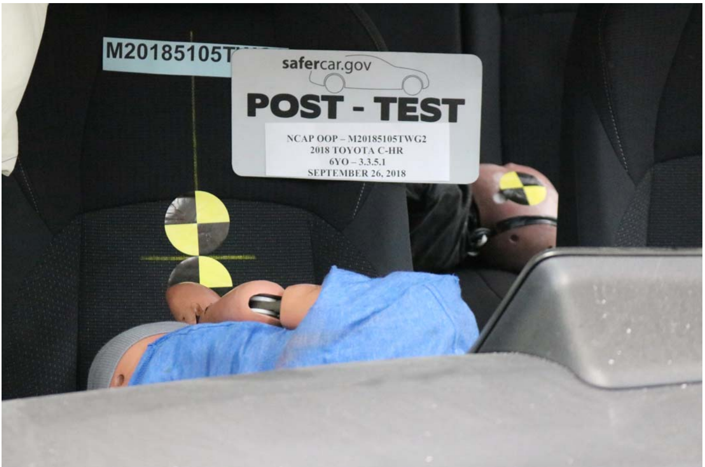
Photo No. 016 - Post-Test 6-Year-Old Child Dummy Front Close-Up View
