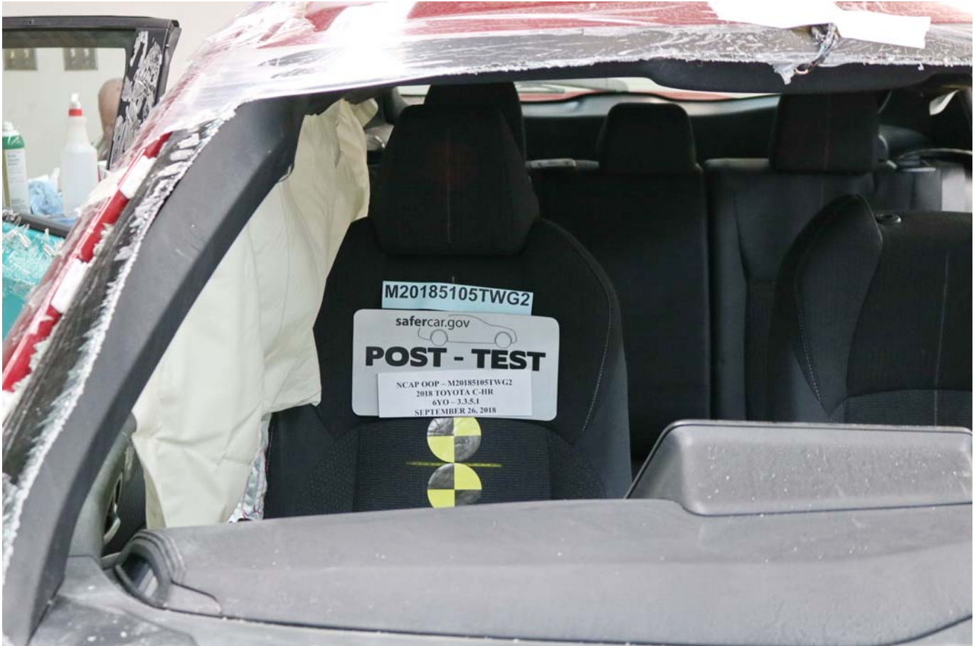
Photo No. 024 - Post-Test Curtain Airbag Front View
