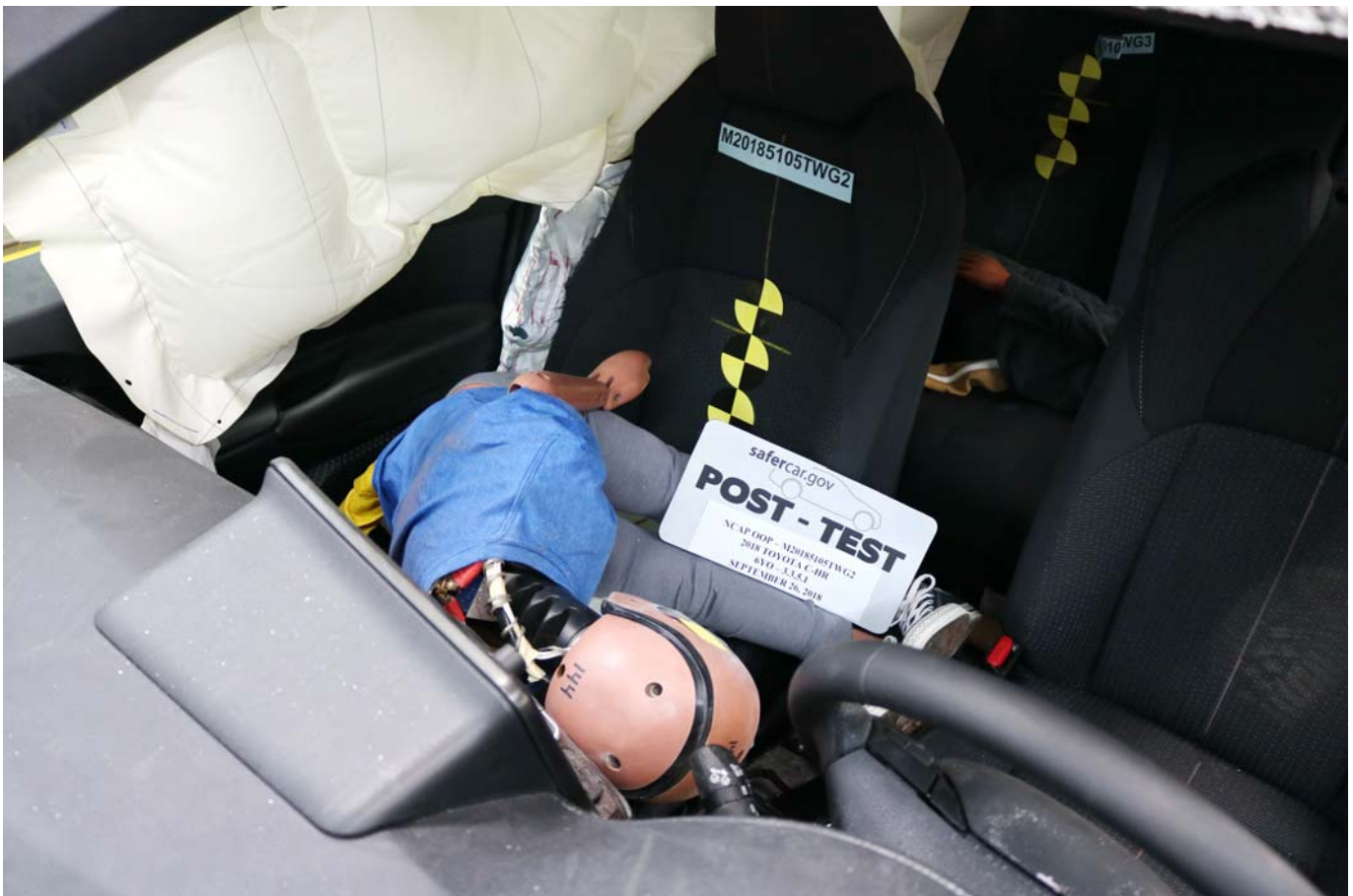
Photo No. 012 - Post-Test 6-Year-Old Child Dummy Left Three-Quarter Front Close-Up View
