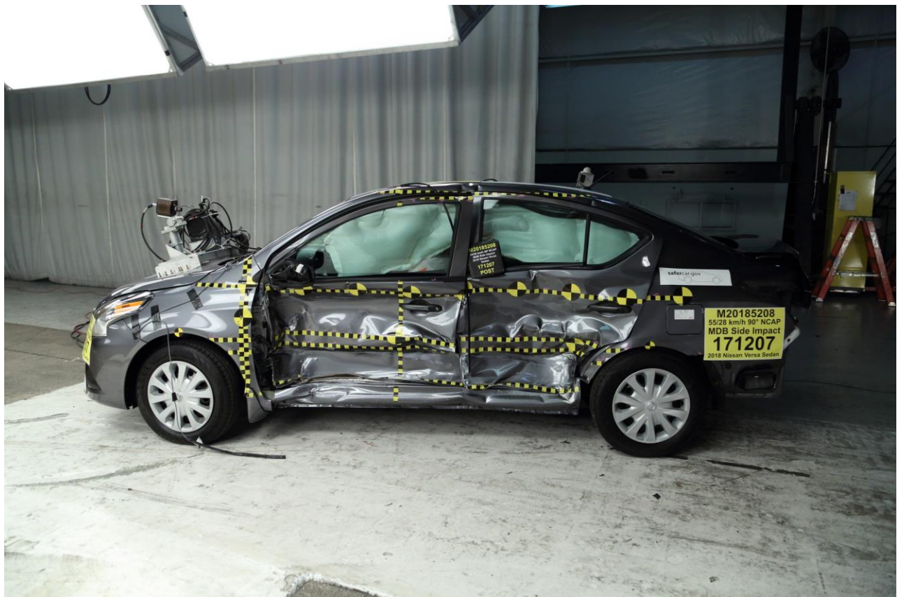
Figure A-4 Post-Test Vehicle Left Side View
