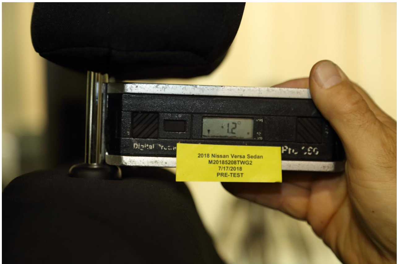
Figure A-8 Pre-Test Vehicle Seat Back Angle
