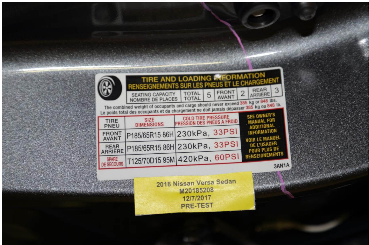
Figure A-2 Vehicle Certification Label
