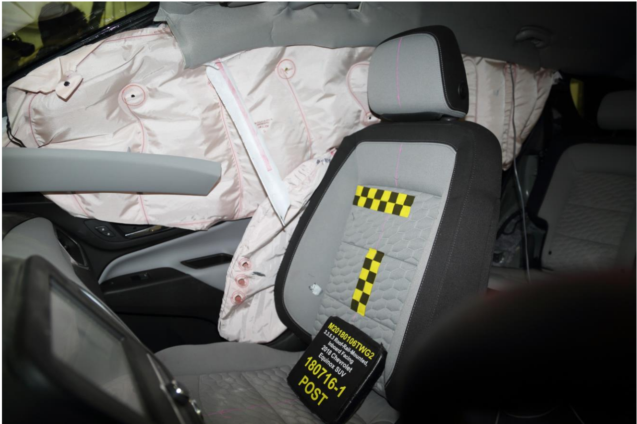
Figure A-27 Post-Test Curtain Air Bag Left 3/4 Front View
