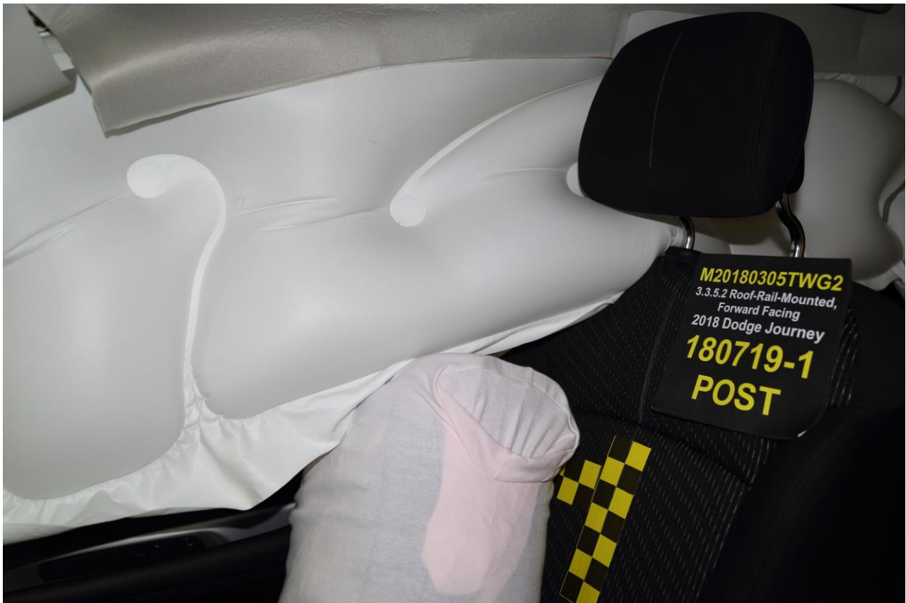
Figure A-16 Post-Test Dummy Left \frac{3}{4} Front Close-up View
