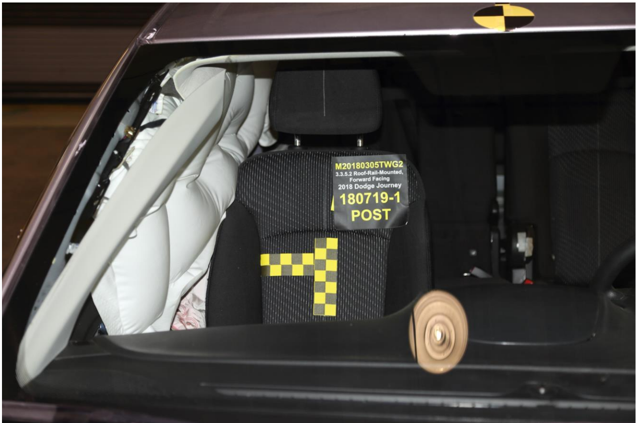
Figure A-28 Post-Test Curtain Air Bag Front View
