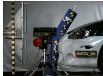
**Figure 5. Legform at time of maximum bending angle in Mazda Miata center impact (C).**
