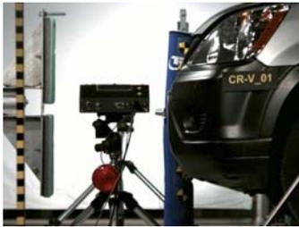
**Figure 13. Legform at time of maximum bending angle in Honda CR-V impact (C).**
