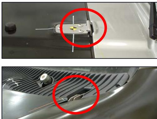
**Figure 18. Wrangler (Top) & E350 Hinges.**
