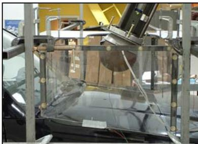
**Figure 2. Test setup for adult headform impact on Toyota 4Runner.**
