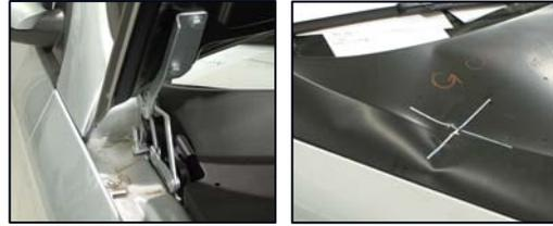
**Figure 19. Passat hinge with low-profile deformable hinge and crush space over hinge.**
