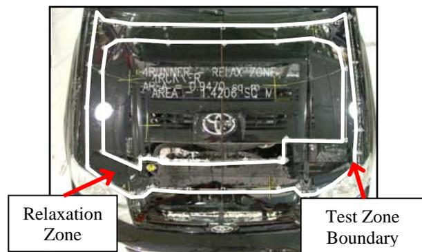
**Figure 3. Example of test zone and relaxation zone boundaries in Toyota 4Runner.**
