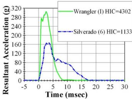
**Figure 17. Resultant acceleration of most severe hinge impact (Wrangler, green solid) and least severe hinge impact (Silverado, blue dashed), showing difference in impact duration.**
