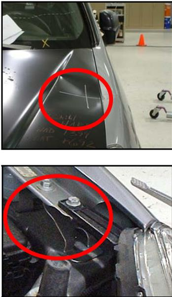
**Figure 22. CR-V Countermeasures at Fender.**
