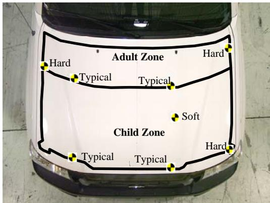
**Figure 1. Test zones and eight impact points shown for the 2006 Toyota Tacoma.**
