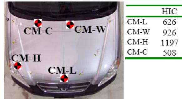
Figure 15. 2005 Honda CR-V counter-measure impacts for comparison only.
