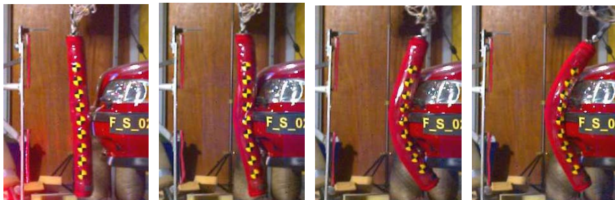
Figure 10. Kinematics of FlexPLI legform for three vehicles.
