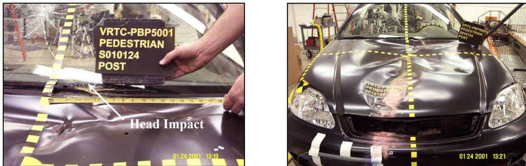
Figure 3.2. Damage patterns and comparison with marked contact points documented from actual case
