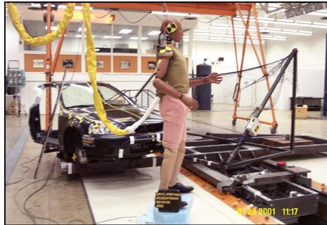
Figure 2.5. Civic Test Setup
