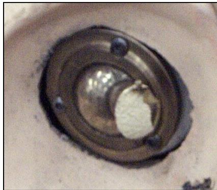
Figure 3.8. Broken right hip sustained in Test 3
