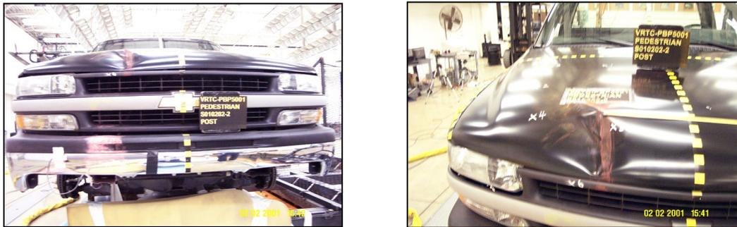
Figure 4.6. Damage patterns and comparison with marked contact points documented from actual case
