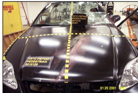
Figure 3.7. Damage patterns and comparison with marked contact points documented from actual case
