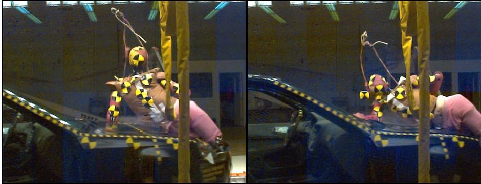
Figure 5.11. Left shoulder shaft fracture
