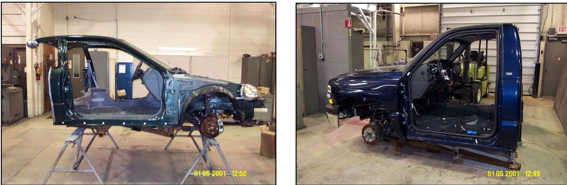
Figure 2.3. Civic (left) and Silverado (right) with frame for buck attachment
