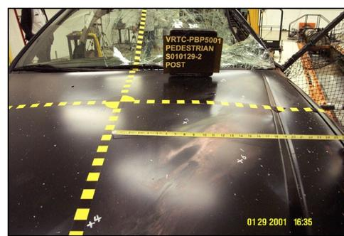
Figure 3.10. Damage patterns and comparison with marked contact points documented from actual case
