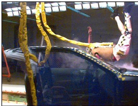
Figure 5.12. Circumstances leading to rupture of the rear neck cable
