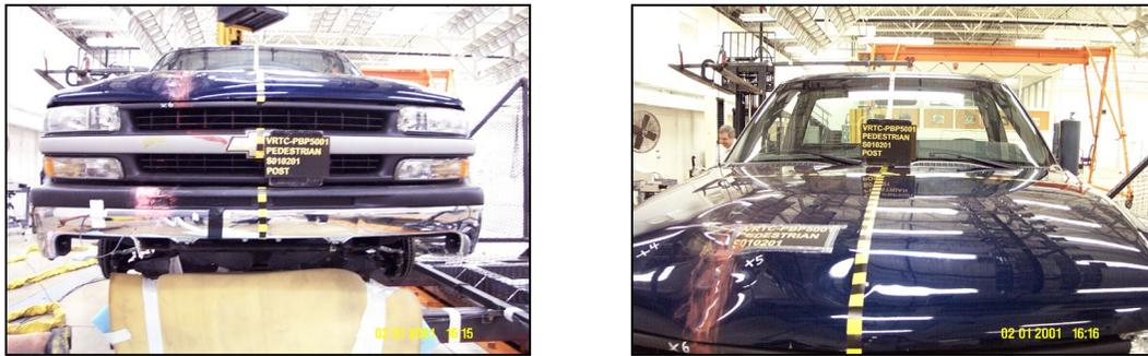
Figure 4.2. Damage patterns and comparison with marked contact points documented from actual case
