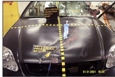
Figure 3.12. Damage patterns and comparison with marked contact points documented from actual case
