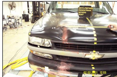
Figure 4.4. Damage patterns and comparison with marked contact points documented from actual case
