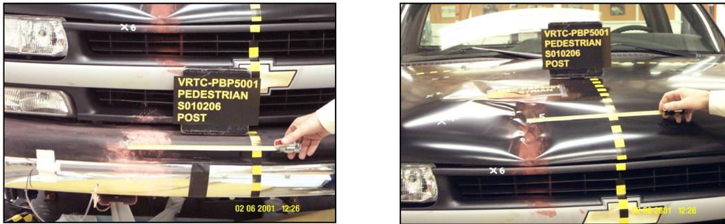
Figure 4.10. Damage patterns and comparison with marked contact points documented from actual case
