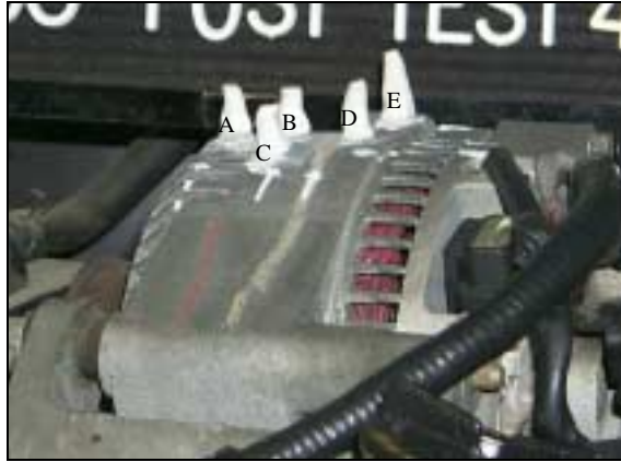
Figure 7. Clay Cone Configuration on Alternator
