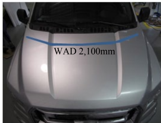
Figure 2. Ford F-150 with rearward portion of hood excluded beyond WAD 2,100 mm
