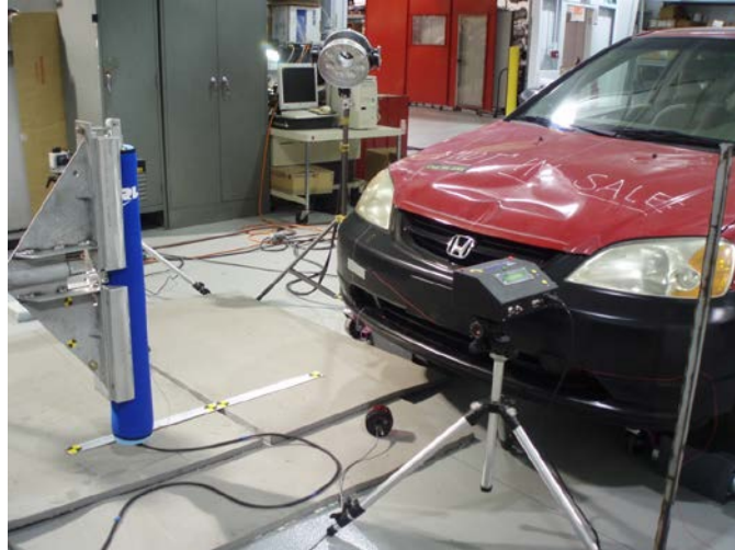
Figure 50. Test setup with the EEVC legform. The instrumentation wires exit from the bottom of leg.
