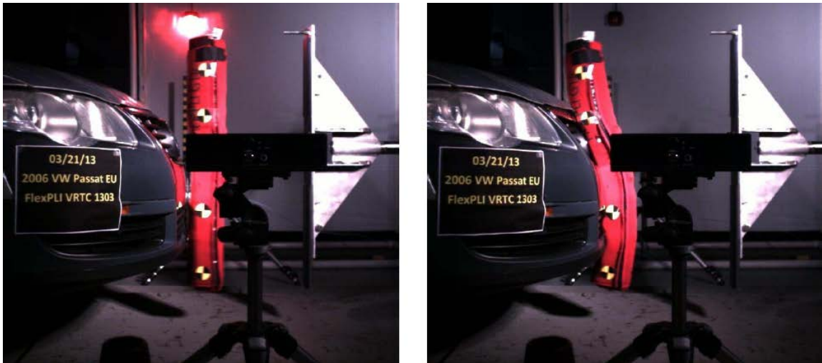
Figure 106. 2006 European Volkswagen Passat impact at times of first contact (left) and maximum deflection (right).
