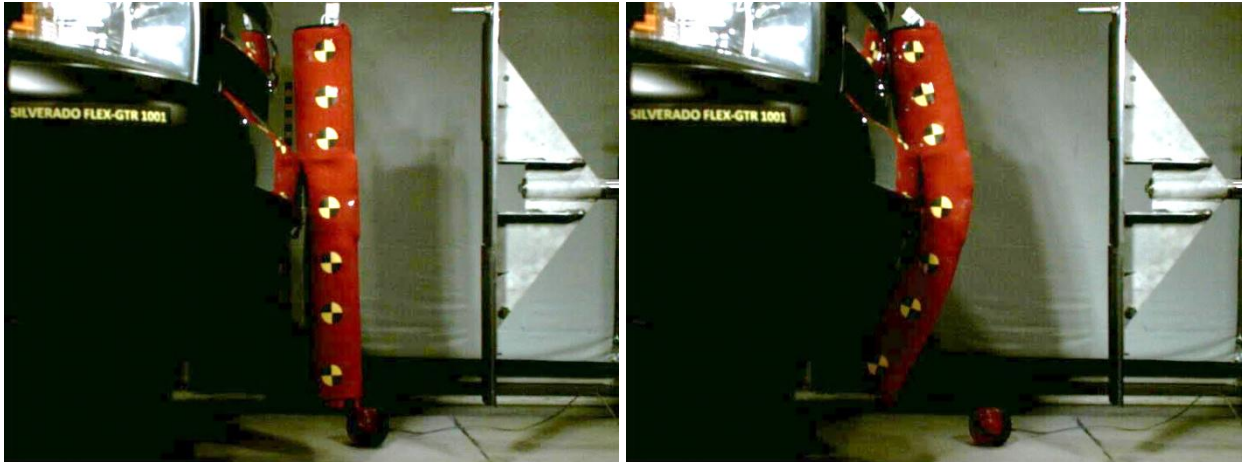
Figure 143. 2007 Chevrolet Silverado impact at times of first contact (left) and maximum deflection (right).
