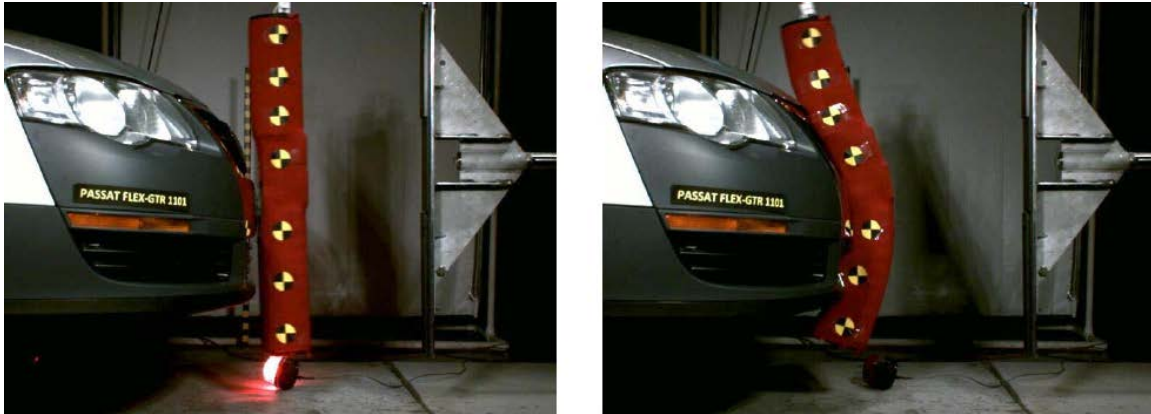
Figure 105. 2006 North American Volkswagen Passat impact at times of first contact (left) and maximum deflection (right).
