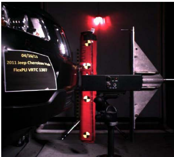
Figure 126. Figure 143. 2011 Hybrid Jeep Grand Cherokee impact at times of first contact (left) and maximum deflection (right).
