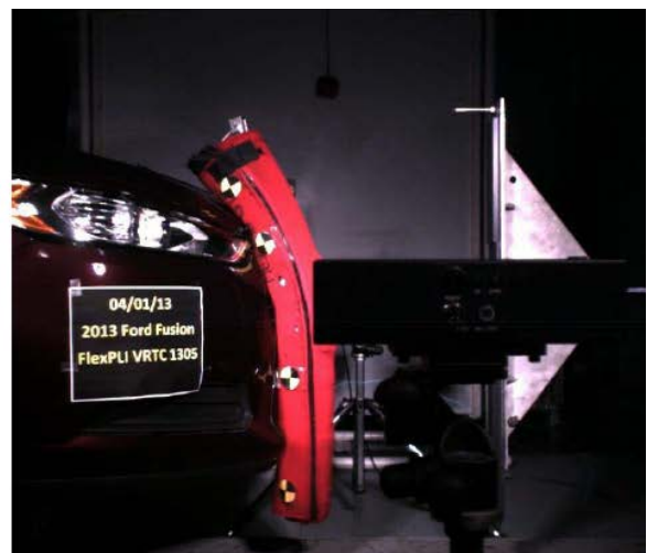
Figure 83. 2013 Ford Fusion outboard impact at times of first contact (left) and maximum deflection (right).
