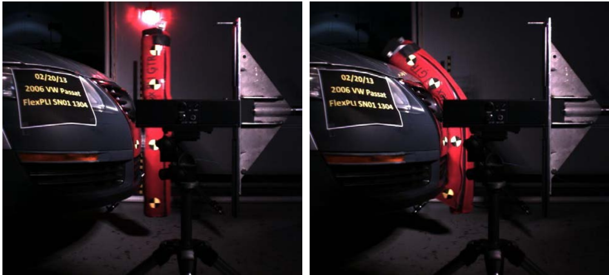
Figure 151. 2006 Volkswagen Passat impact at times of first contact (left) and maximum deflection (right).
