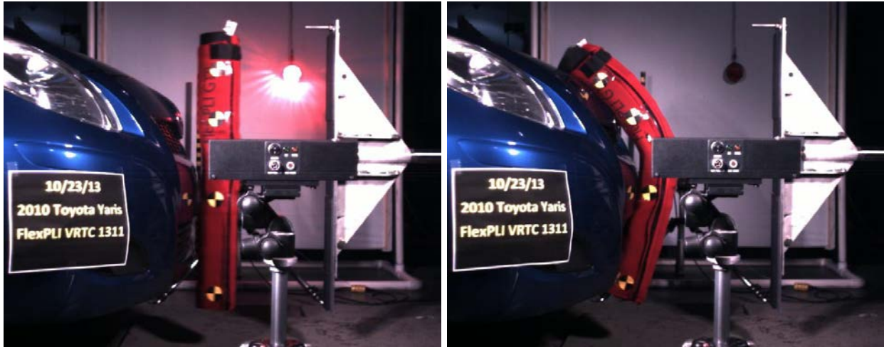
Figure 97. 2010 North American Toyota Yaris impact at times of first contact (left) and maximum deflection (right).
