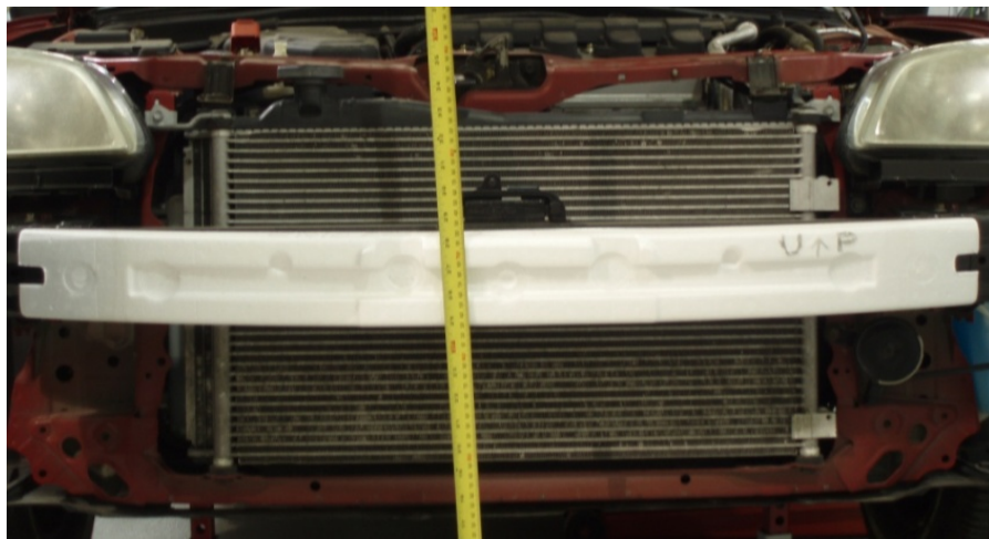
Figure 19. 2002 Honda Civic front view without the fascia.
