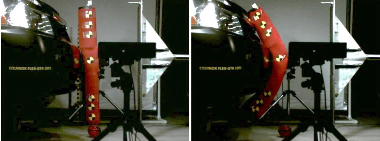
Figure 58. 2009 Chevrolet Equinox impact at times of first contact (left) and maximum deflection (right).
