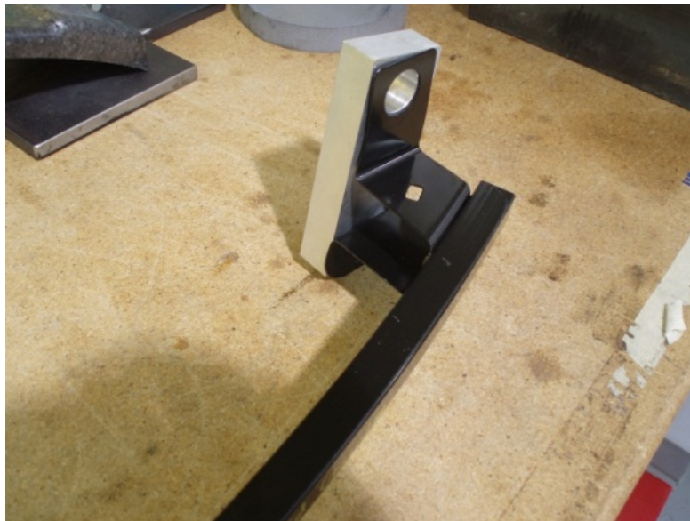
Figure 124. A close-up view of a lower bumper stiffener (LBS) for the 2011 Jeep Grand Cherokee. A spacer was fabricated to push the LBS forward so that its front edge was up against the fascia.
