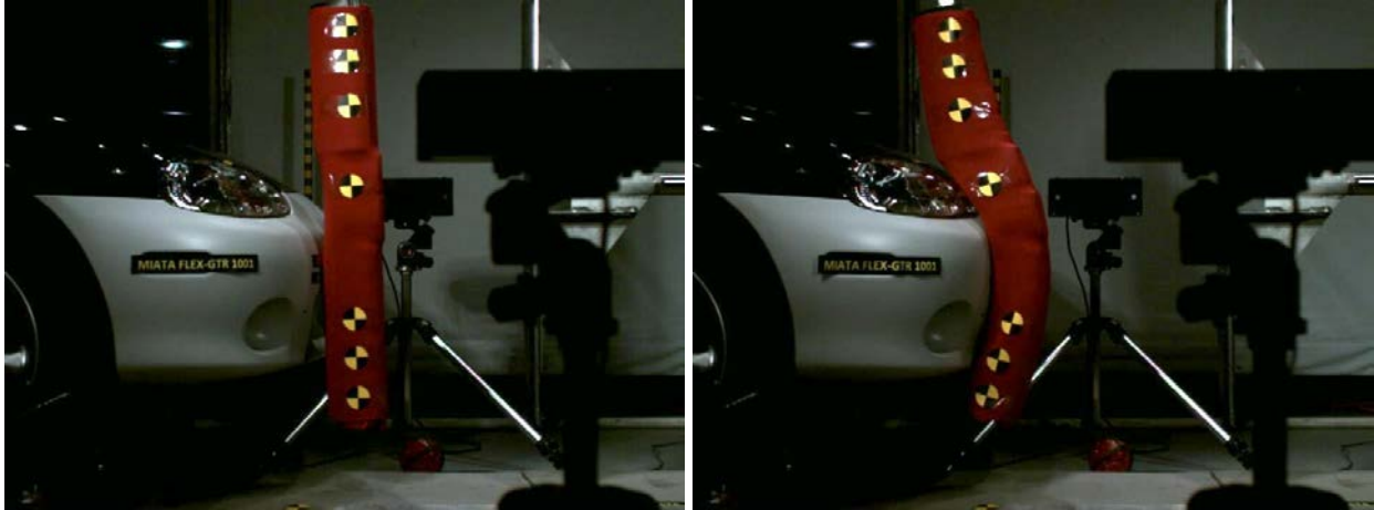
Figure 66. 2002 Mazda Miata impact at times of first contact (left) and maximum deflection (right).
