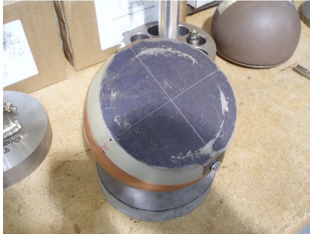
Figure 26. Cellbond headform with additional thin metal back plate used to produce a stronger connection with the launch plate magnet.
