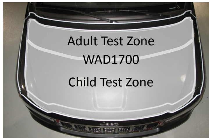
Figure 9. Child & adult test zones shaded in gray as defined by the GTR on vehicle's bonnet top.
