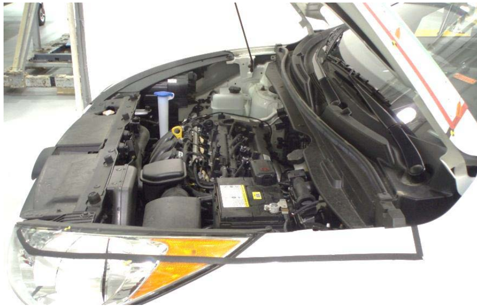
Figure 49. Increased space in the engine bay between engine components and the hood.
