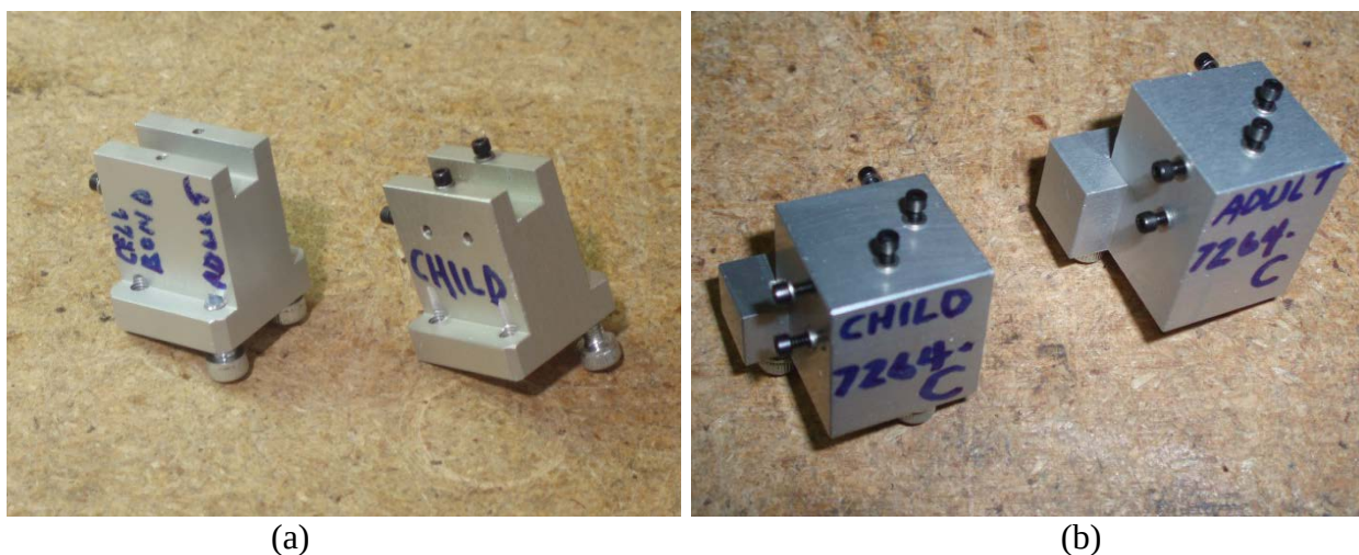
Figure 25. Accelerometer mount for uni-axial Kyowa ASE or Endevco 7264B accelerometers (a) and for Endevco 7264C/7264G accelerometers (b).
