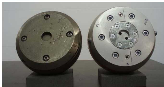
Figure 19. Backplates of the FTSS child (left) and Cellbond child (right) headforms.
