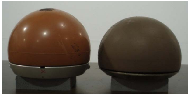
Figure 17. Cellbond (left) and FTSS (right) child headforms.
