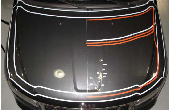
Figure 10. Evaluation of impact point definition on a vehicle. The outer white boundary represents the bonnet top. The inner white boundary represents the test zone as well as the 3D first contact launch area. The orange boundary represents the driver side half of the aiming point launch area. The launch area using the 2D measuring point is not pictured (to be discussed later).
