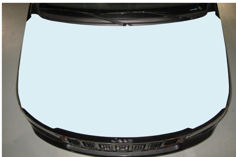
Figure 8. The bonnet top of a vehicle as defined by the GTR
