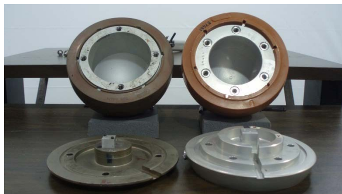
Figure 20. FTSS child (left) and Cellbond child (right) headforms with backplates removed.
