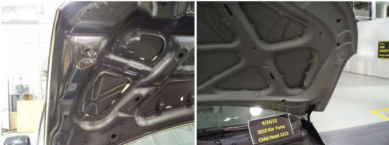
Figure 47. Crush spaces on the underside of hoods.
