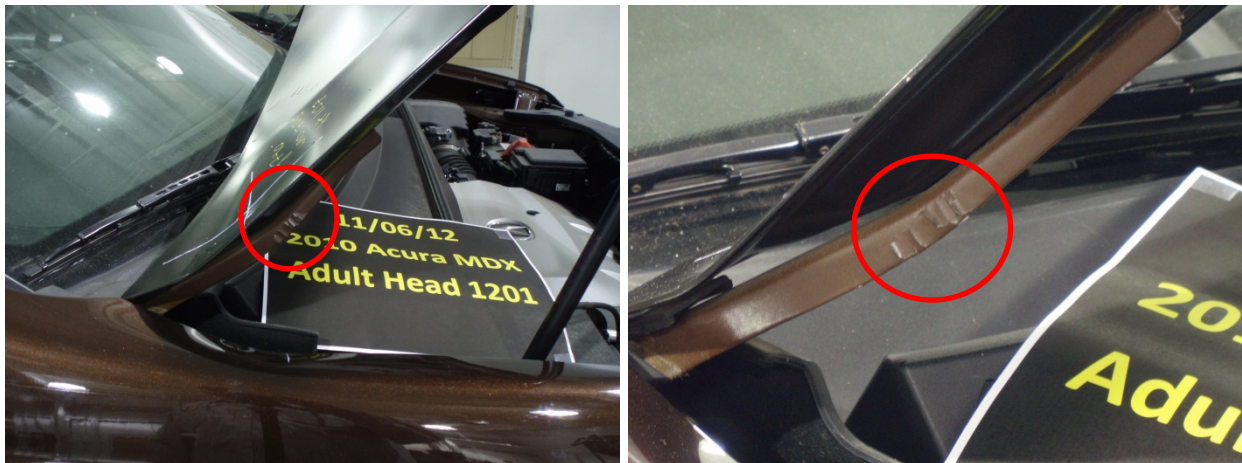
Figure 48. The hood hinge for the Acura MDX is normally unbent. Circled in red is a bent and deformed hood hinge as result of a head impact.
