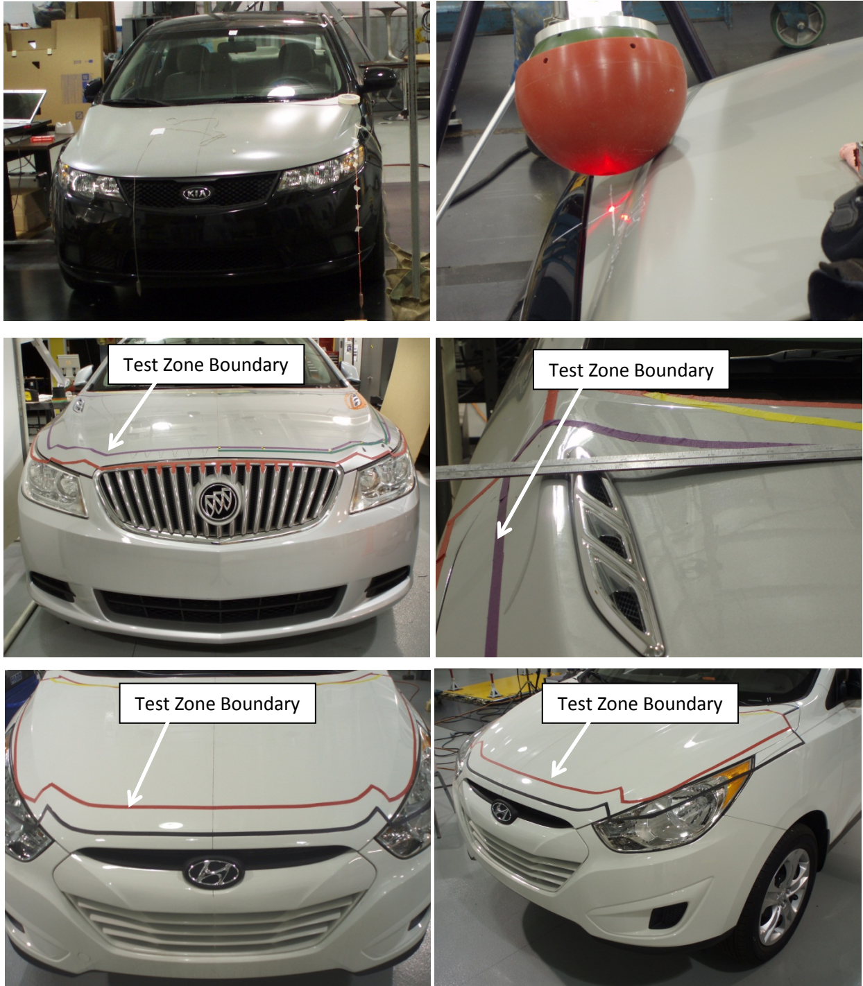
Figure 45. The Kia Forte (top), Buick LaCrosse (center), and Hyundai Tucson (bottom) have more of a clamshell-like geometry and the hood is steeper along the sides compared to traditional flat hood designs. The side boundaries of the hood test zone lie on these steeper side portions of the hood, which produces different launch area side boundaries for the different targeting protocols.
