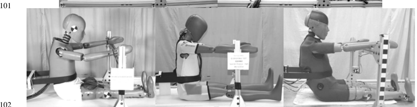
101 102 Fig. 2. Pre-test positions of HIII-50M (top left), THOR-K (top right), HIII 10yo (bottom left), Q10 (bottom center), 103 and LODC (bottom right). 104 105
