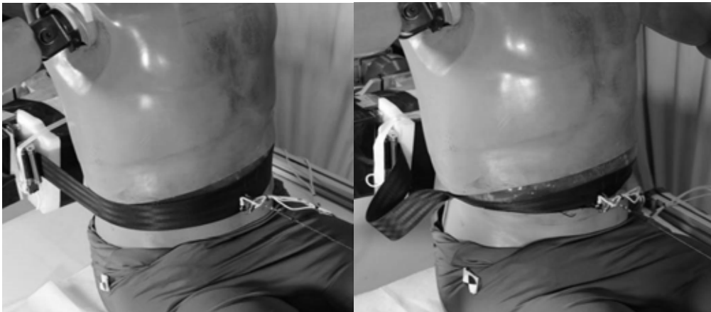
250 Fig. 7. Initial placement of seatbelt on the Hybrid III with RRSA (left); final position of seatbelt trapped between 251 the chest jacket and pelvis (right)
