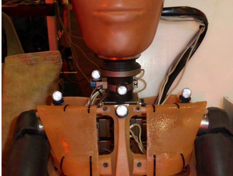
Figure 15. VICON marker locations on LODC
