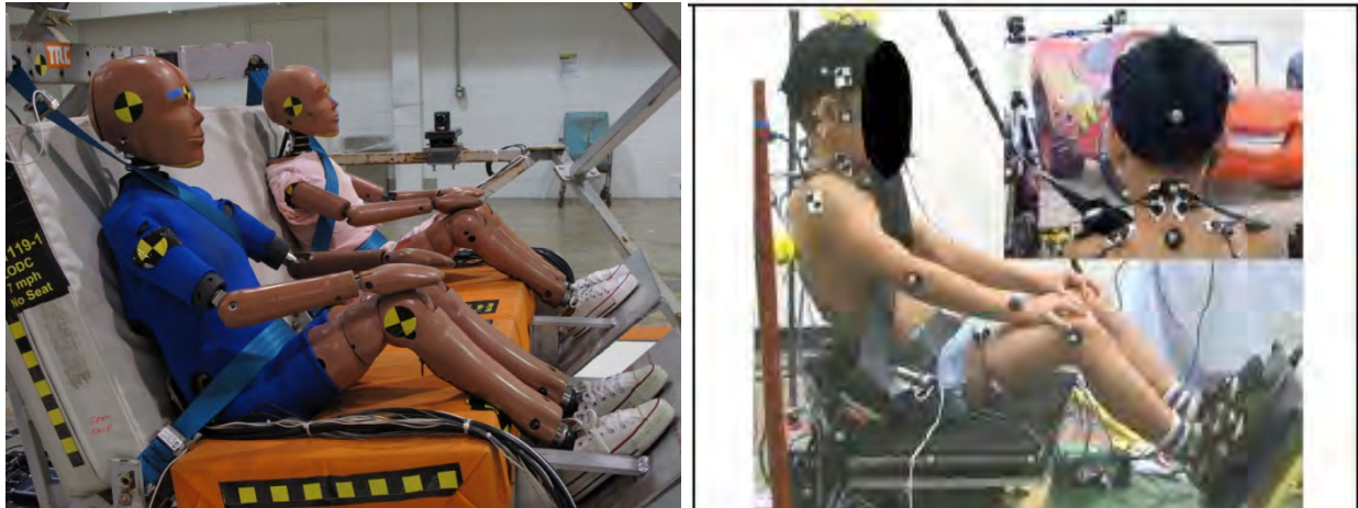
Figure 31. LODC and HIII-10C test setup on revised 213 bench to mimic pediatric volunteer test
