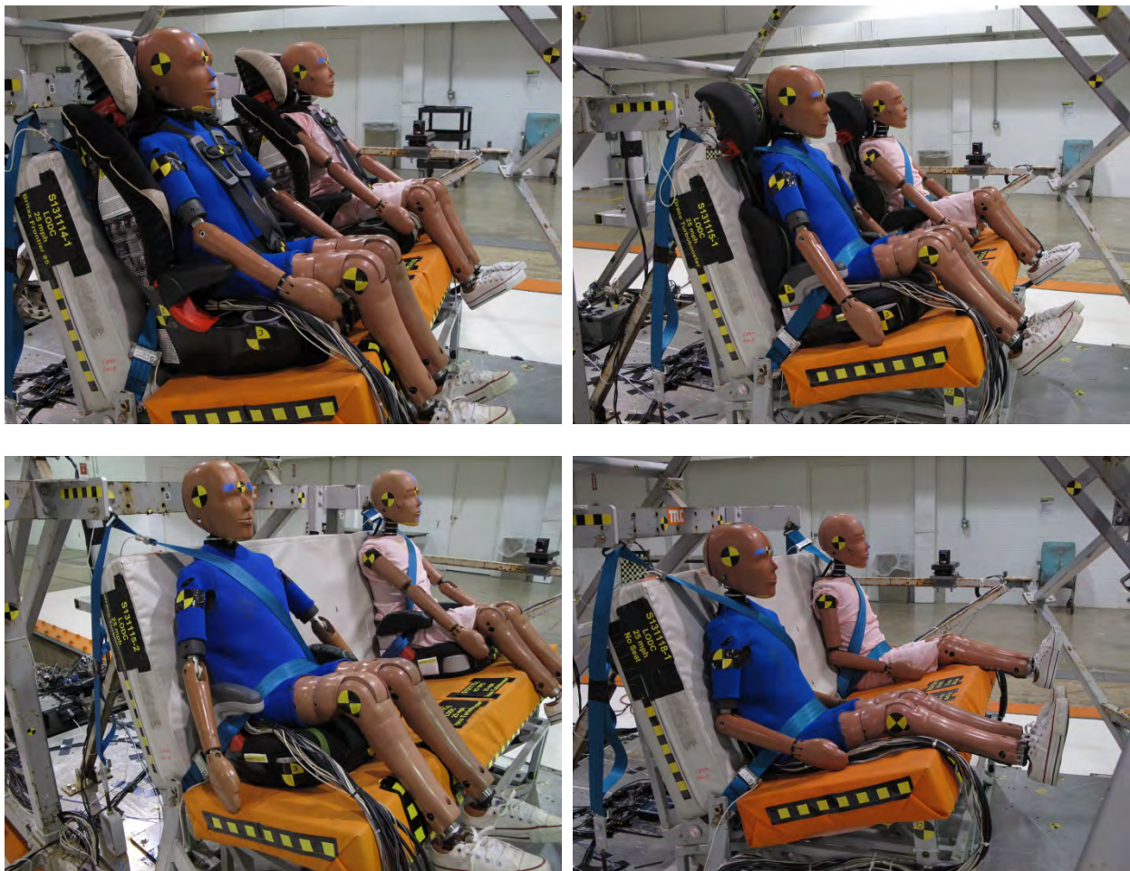
Figure 34. LODC and HIII-10C in (top left) 5 point harness CRS, (top right) highback belt positioning booster, (bottom left) backless belt positioning booster, and (bottom right) non-CRS condition
