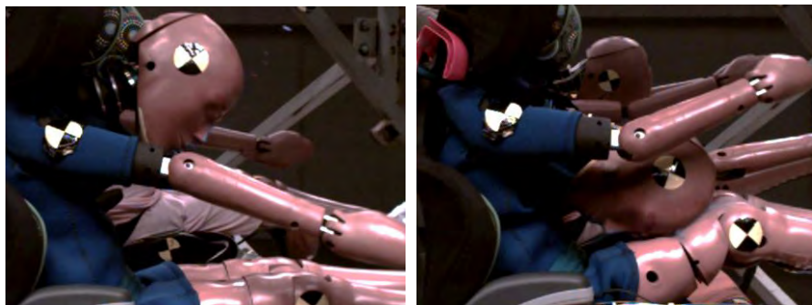
Figure 97. Head-upper leg contact in LODC in highback BPB test (48 km/h)
