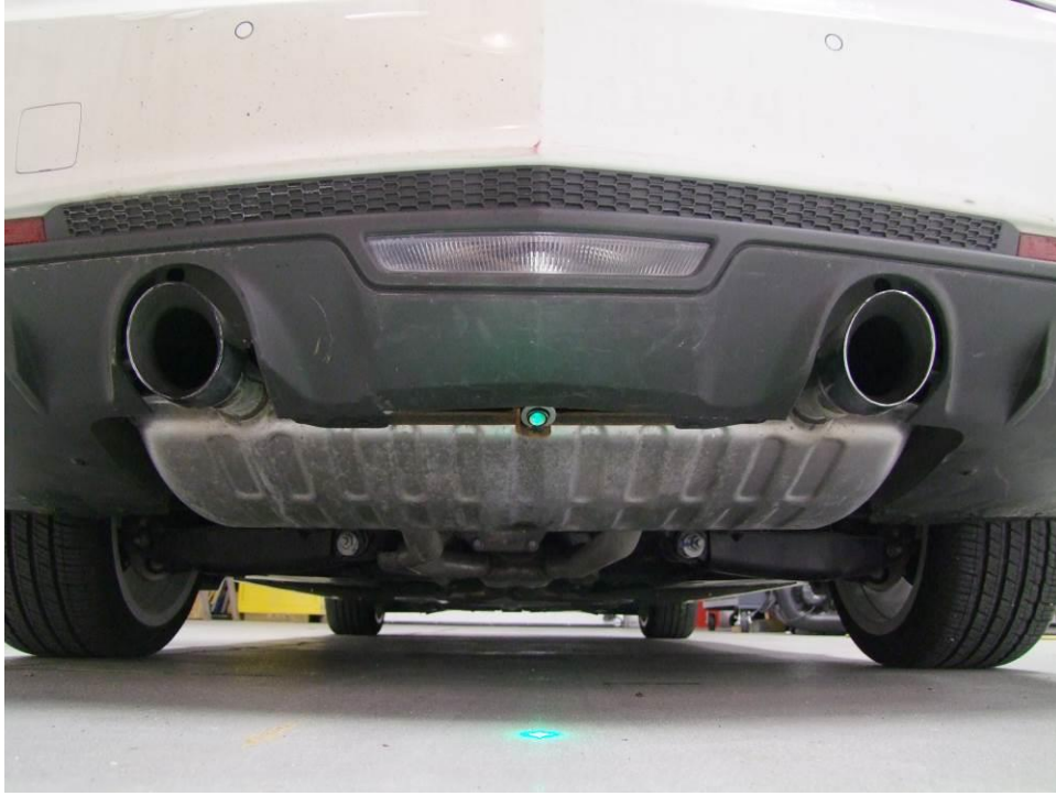
Figure 8. Image of Green Laser Installed on Vehicle Bumper for Alignment Purposes
