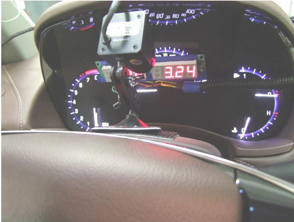
Figure 7. Image of Camera and Equipment, Capturing Instrument Panel Warnings and Vehicle Speed
