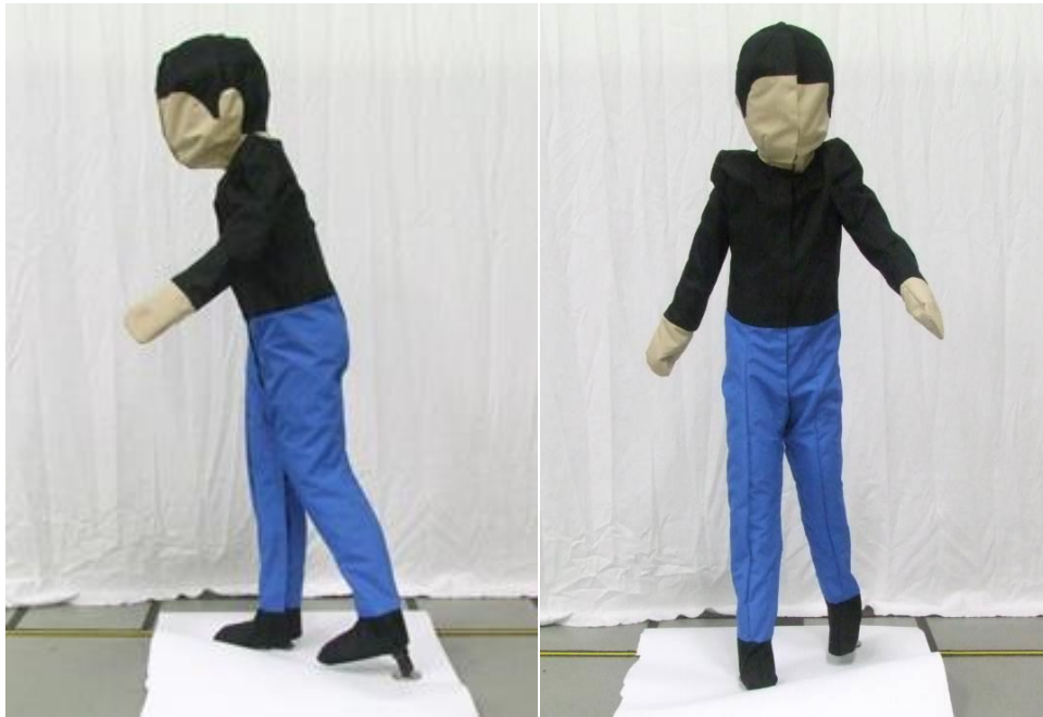
Figure 1. Child Mannequin Test Object, Side View and Front View
