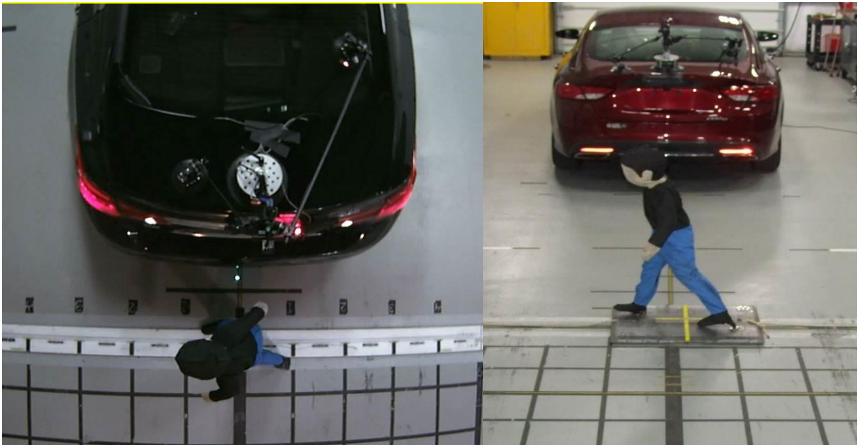
Figure 2. Child Mannequin Test Object at Grid Location 0 Behind Backing Test Vehicle
