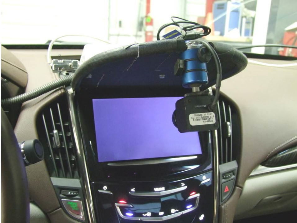
Figure 6. Image of Camera, Capturing Vehicle's Rearview Video Display
