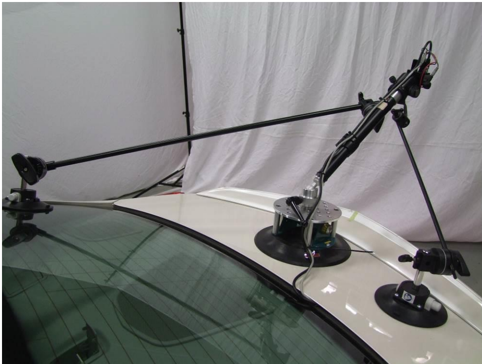
Figure 9. Image of Camera Mounted to Rear Trunk Lid of Vehicle
