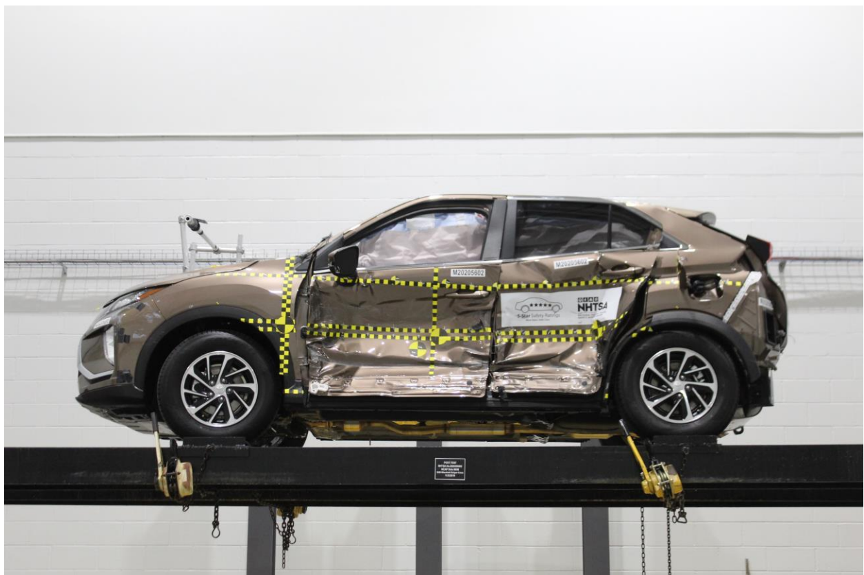
Figure A-100: FMVSS No. 301 Static Rollover 360 Degrees
