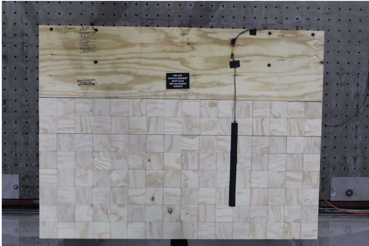
Figure A-2: Pre-Test Load Cell Wall
