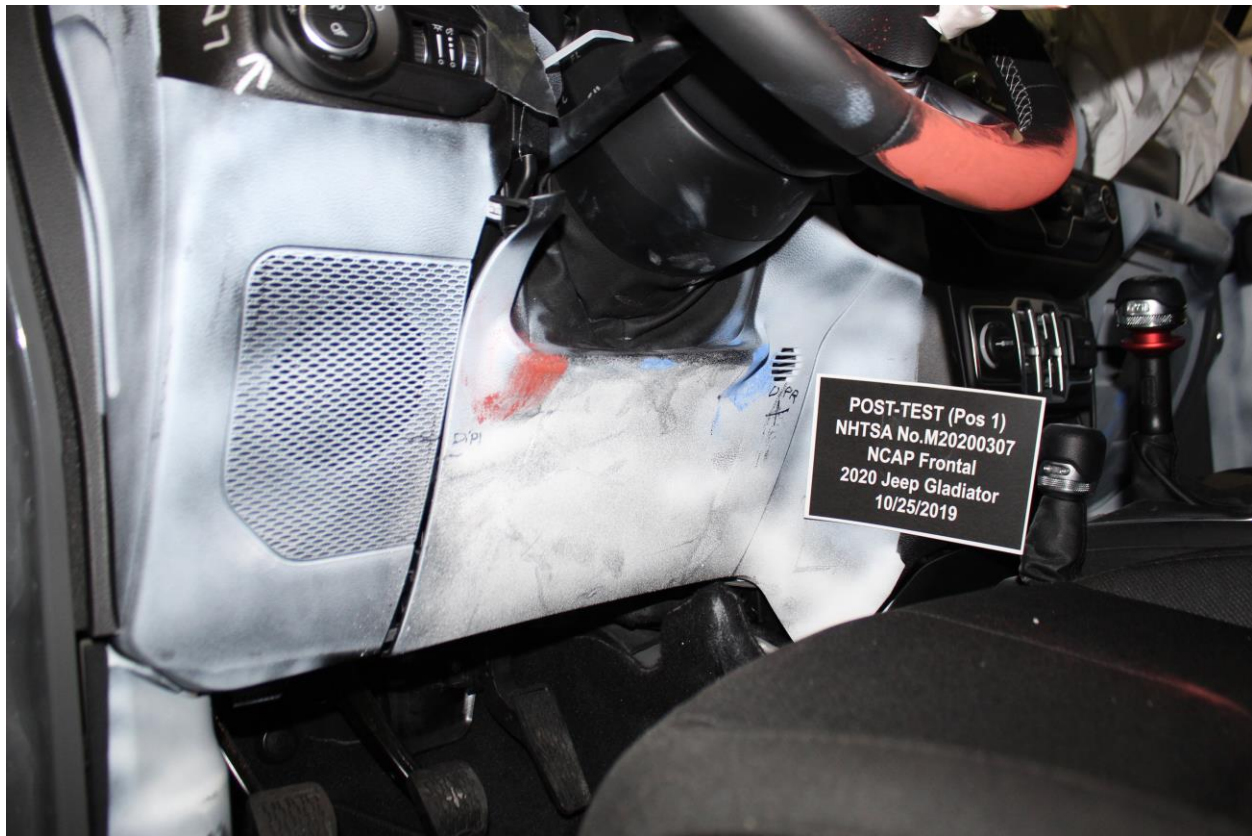
Figure A-45: Post-Test Driver's Side Knee Bolster
