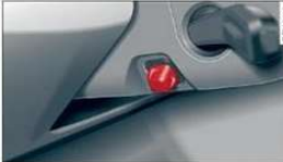
Fig. 53 Steering column: switch for adjusting the steering wheel position
