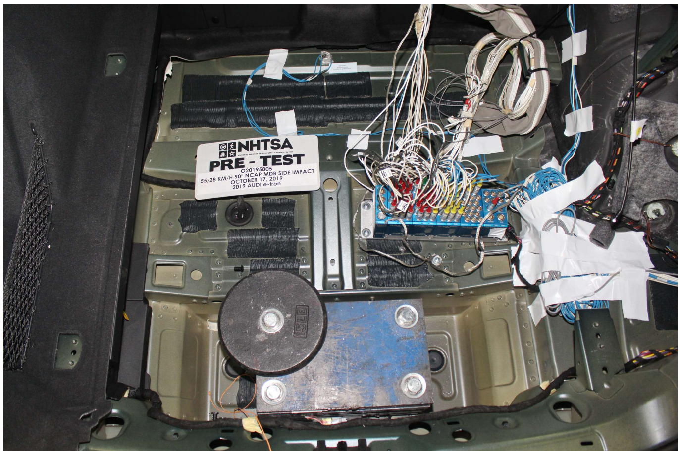
Photo No. 094 - Pre-Test Ballast View
