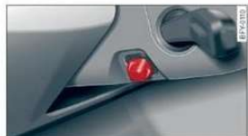
Fig. 53 Steering column: switch for adjusting the steering wheel position
