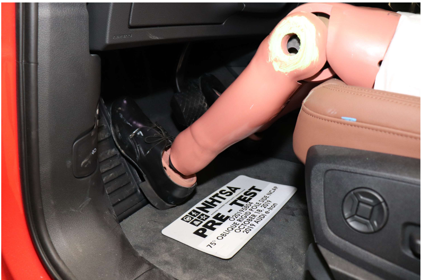
Photo No. 032 - Pre-Test Placement of Dummy Feet
