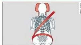
Fig. 54 Correctly adjusted head restraints
