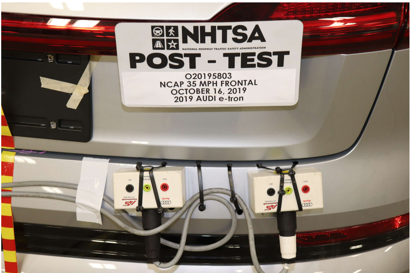
Photo No. 305-025 - Post-Impact View of Installed Test Interface Port
