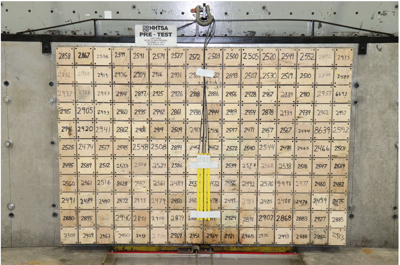
Photo No. 002 - Pre-Test Load Cell Wall
