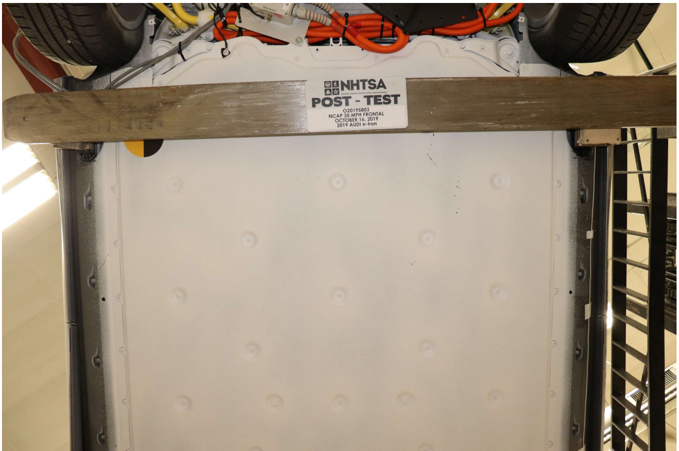
Photo No. 305-011 - Post-Impact Rear View of Propulsion Battery
