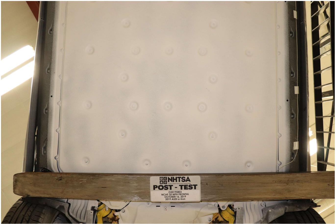
Photo No. 305-010 - Post-Impact Front View of Propulsion Battery
