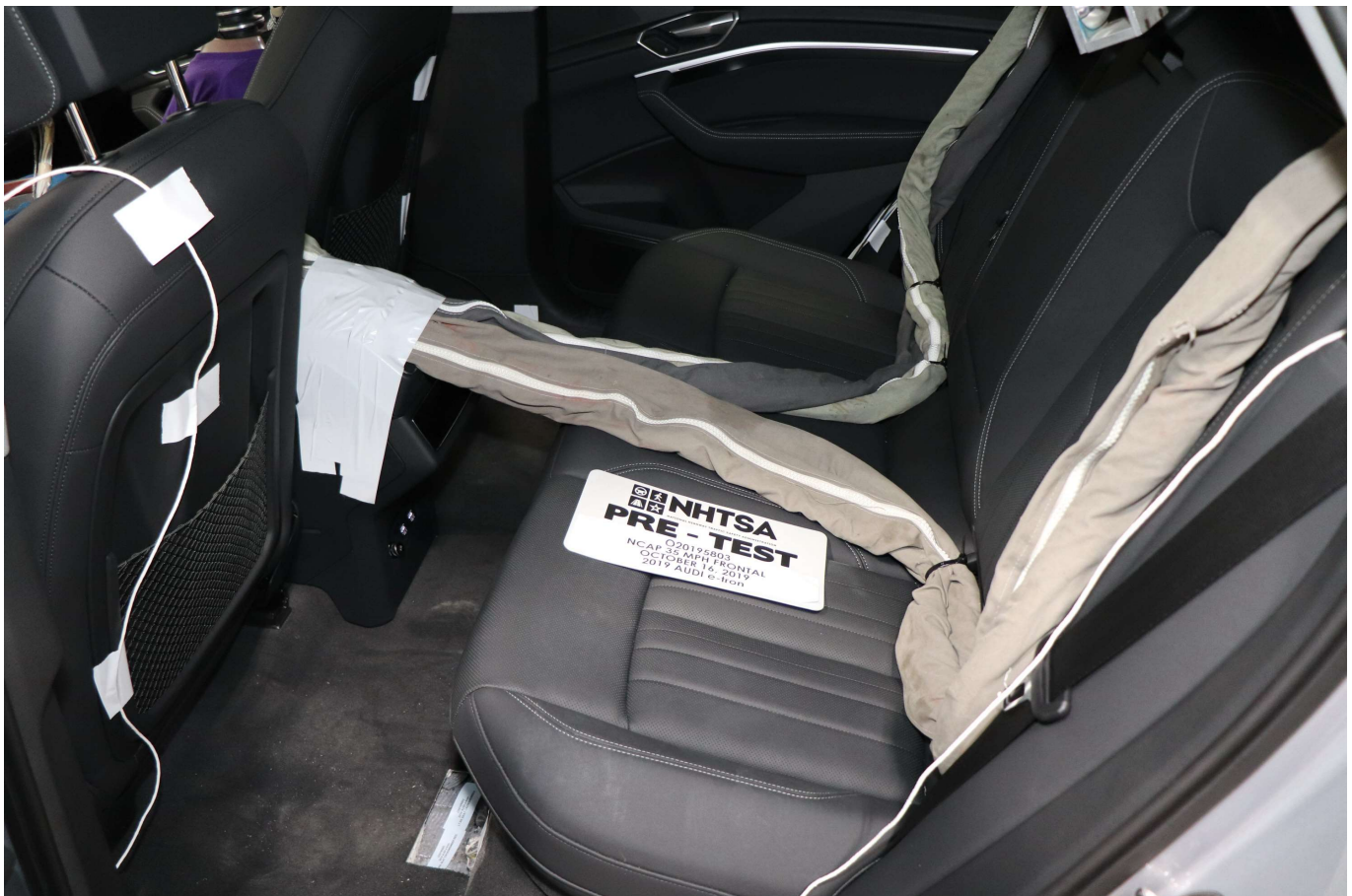
Photo No. 028 - Pre-Test Dummy Cable Routing
