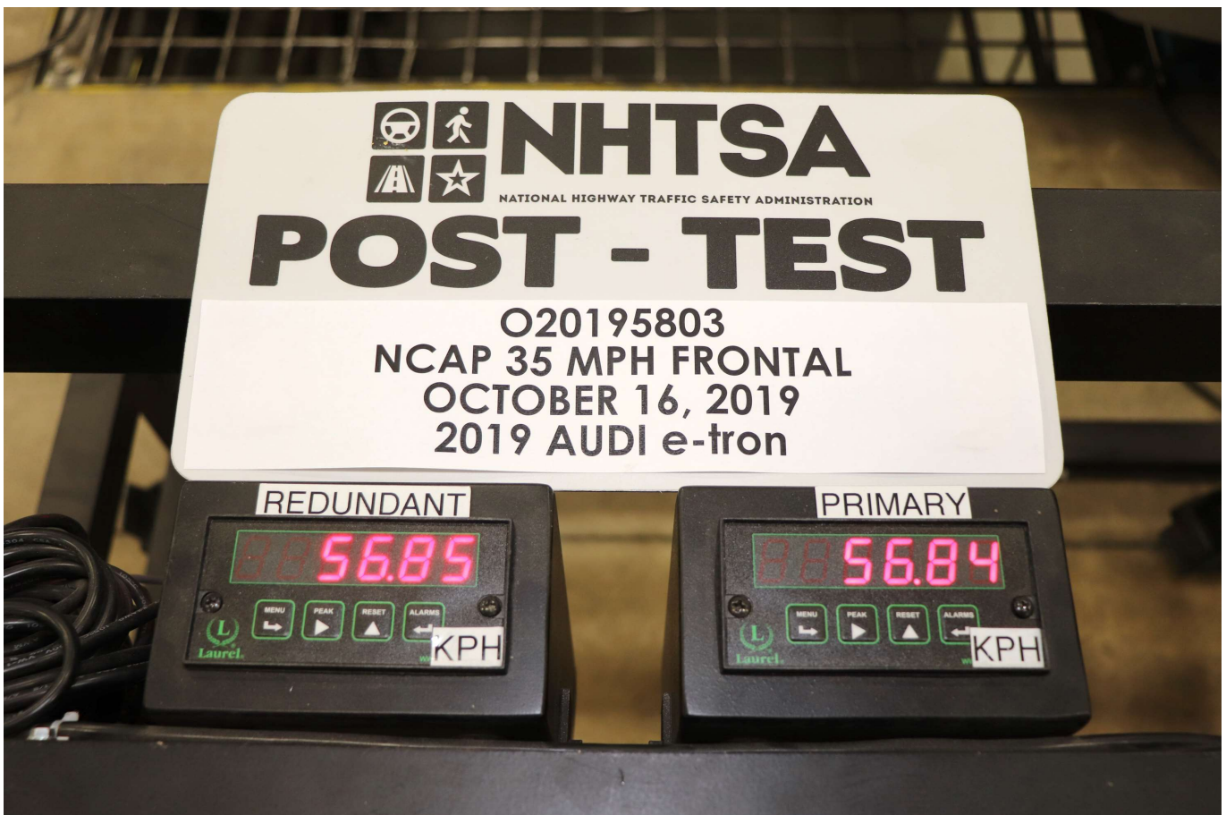
Photo No. 076 - Post-Test Speed Trap Read-Out
