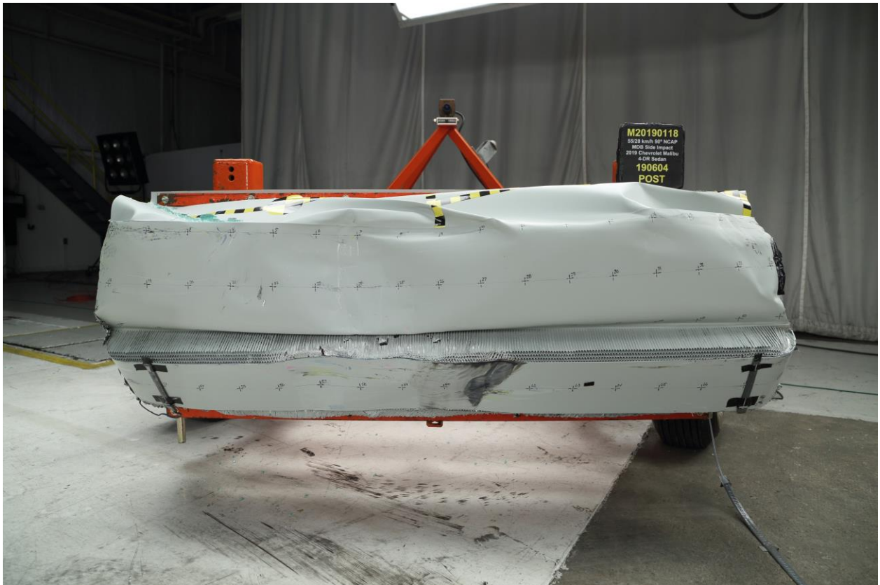
085 Post-Test Front View of MDB Impactor Face
