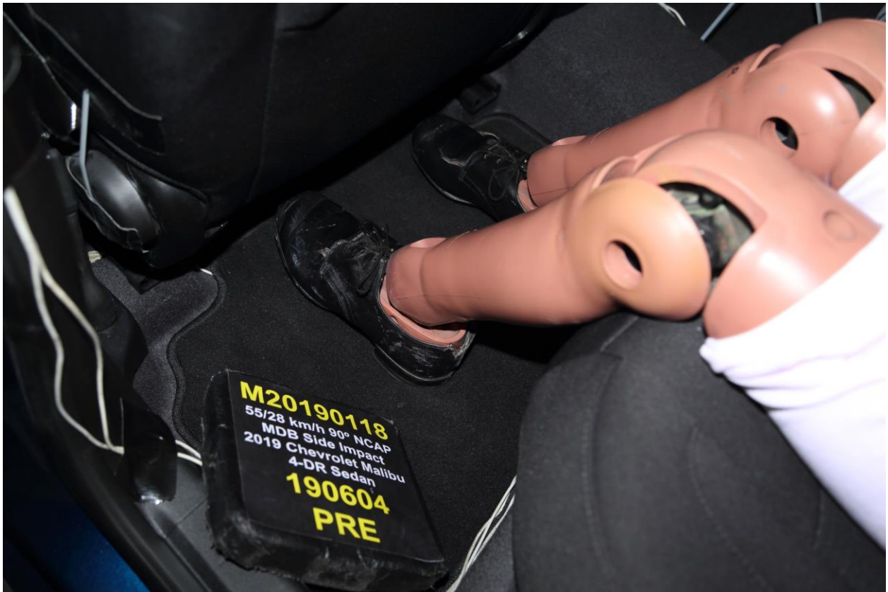
064 Pre-Test Placement of Rear Passenger Dummy's Feet
