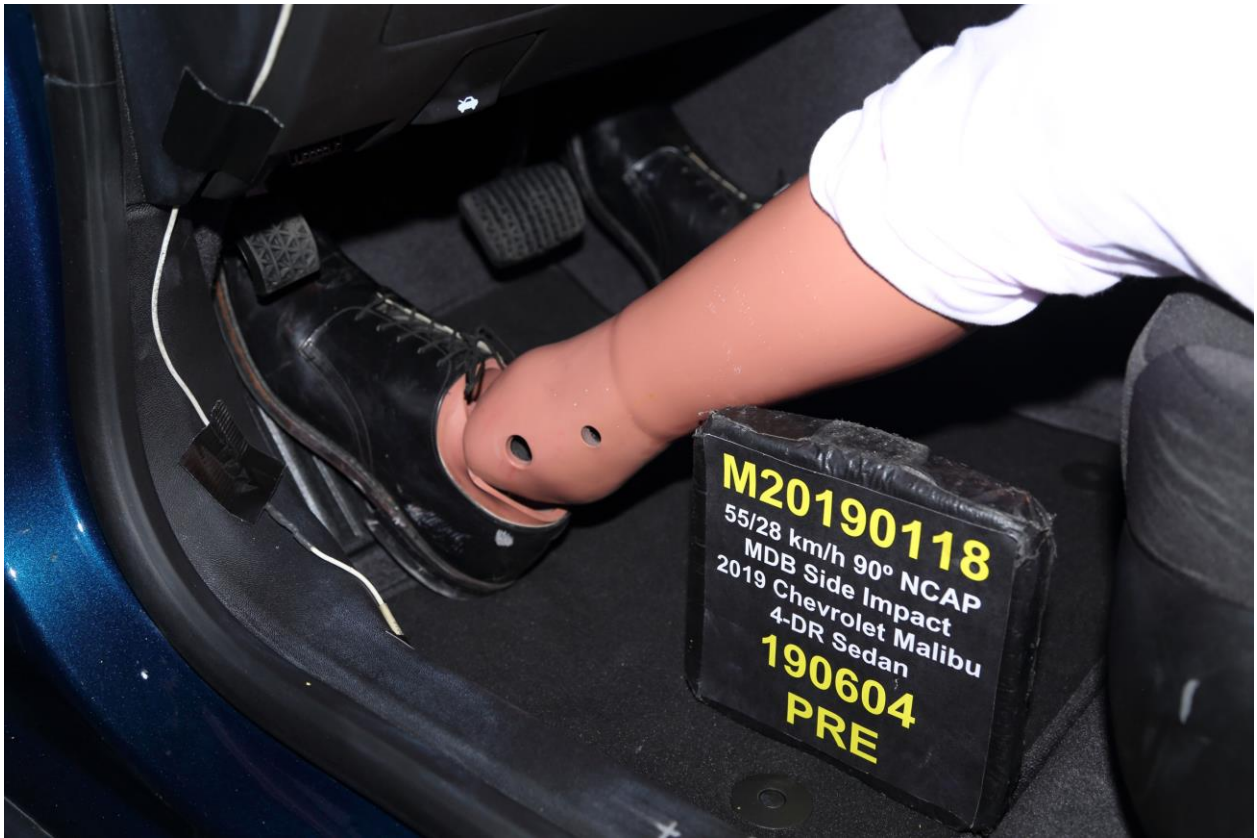
034 Pre-Test Placement of Driver's Dummy Feet
