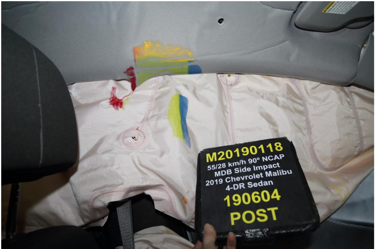
049 Post-Test Driver Dummy Close-Up Head Contact with Side Airbag View
