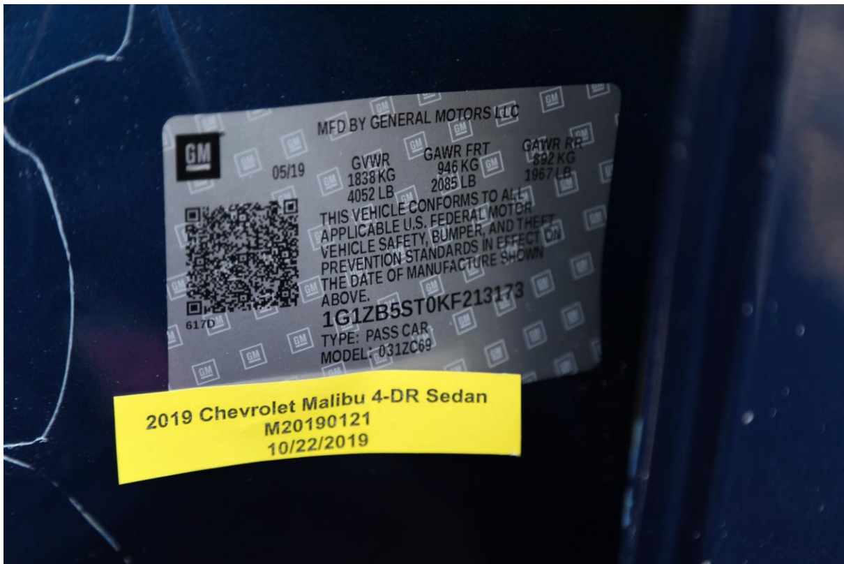
No. 055 Close-Up View of Vehicle Certification Label
