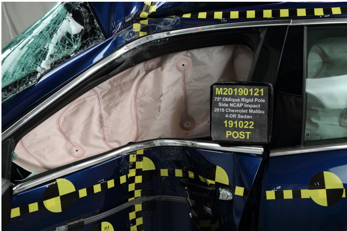
No. 025 Post-Test Left Side View of Dummy Shoulder and Door Top View
