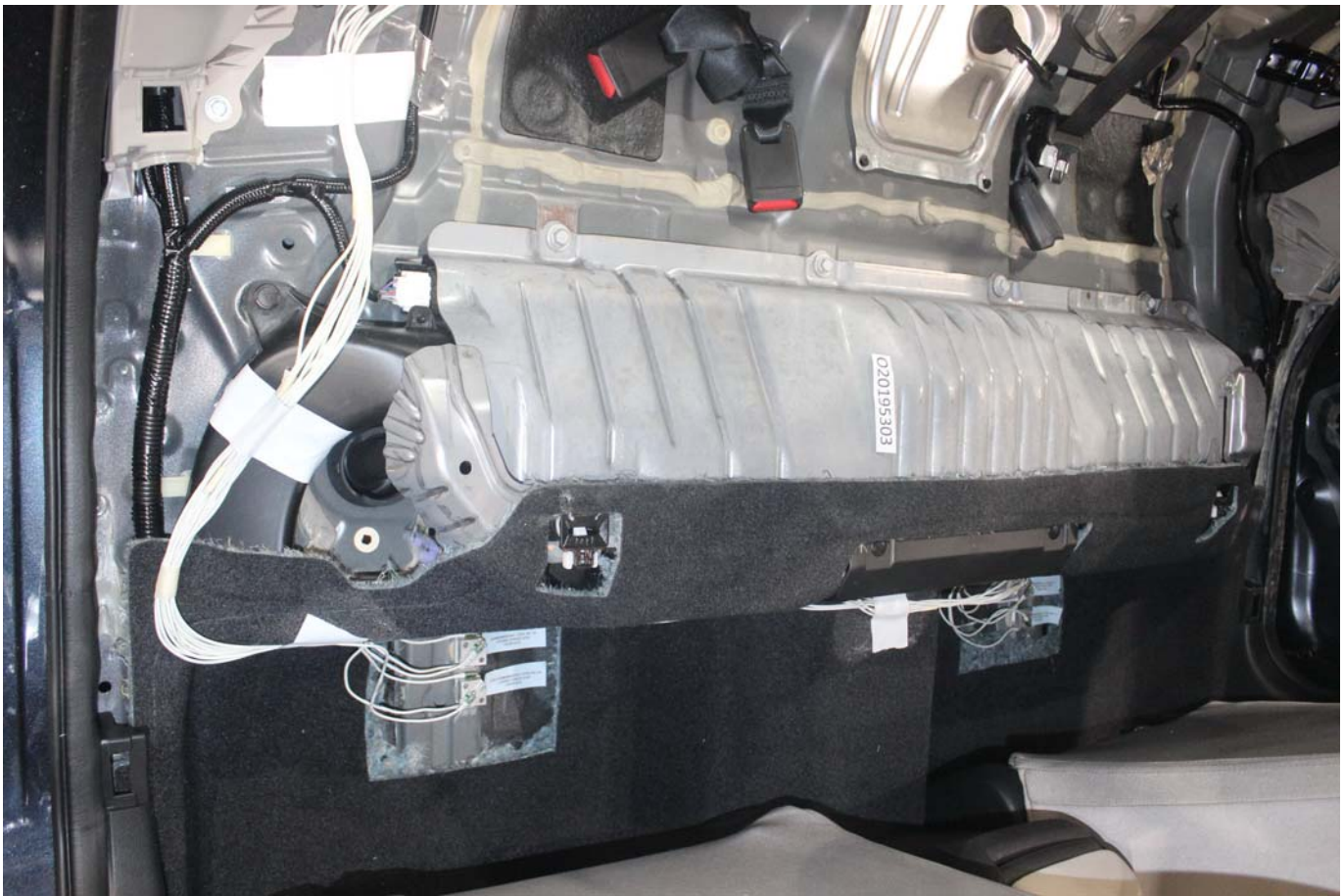
Photo No. 008 - Pre-Impact View of Propulsion Battery
